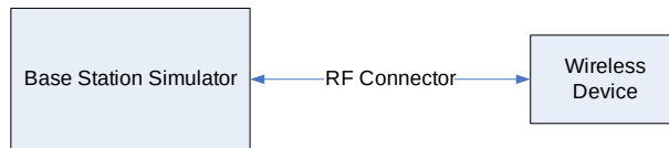
Figure 9-1 Power Measurement Setup
