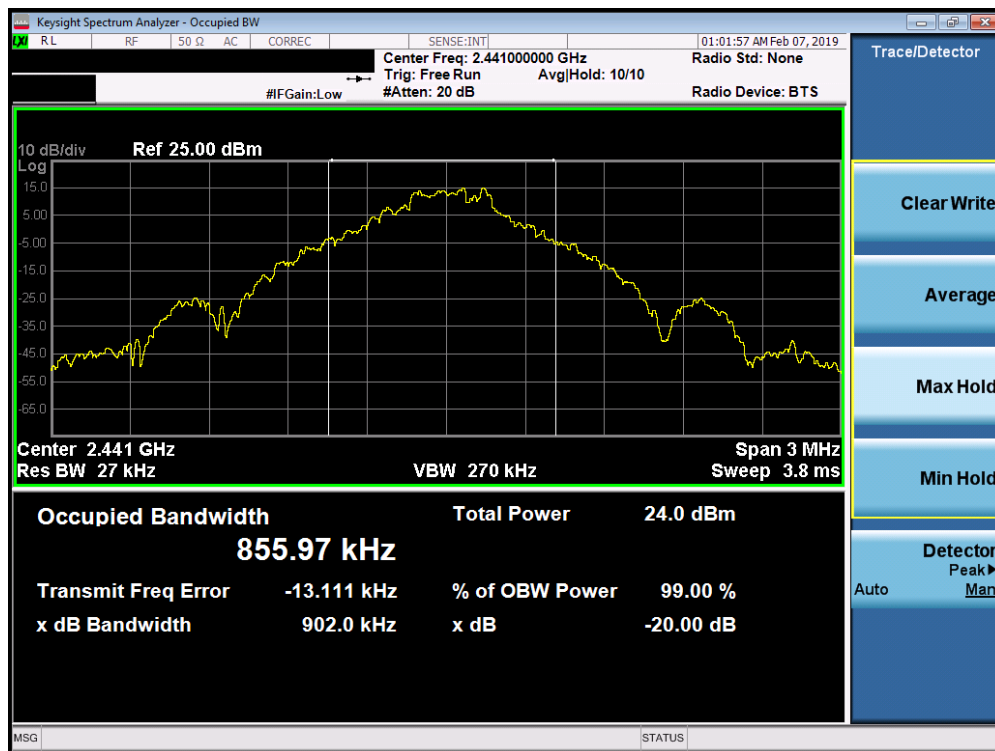
Plot 7-2. 20dB Bandwidth Plot (Bluetooth, 1Mbps – Ch. 39)
