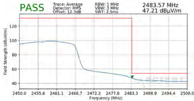
Plot 7-105. Radiated Restricted Upper Band Edge Measurement SISO ANT1 (Average – 242 Tones)
