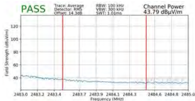
Plot 7-143. Radiated Restricted Upper Band Edge Measurement MIMO (Average – 26 Tones)
