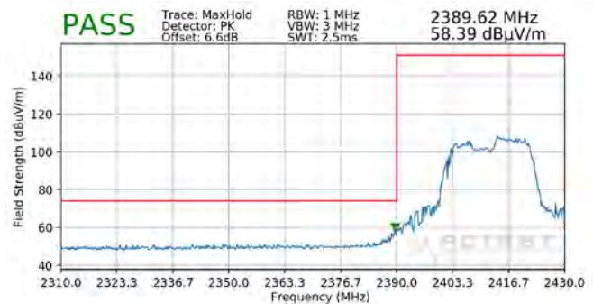
Plot 7-114. Radiated Restricted Lower Band Edge Measurement SISO ANT2 (Peak – 106 Tones)
