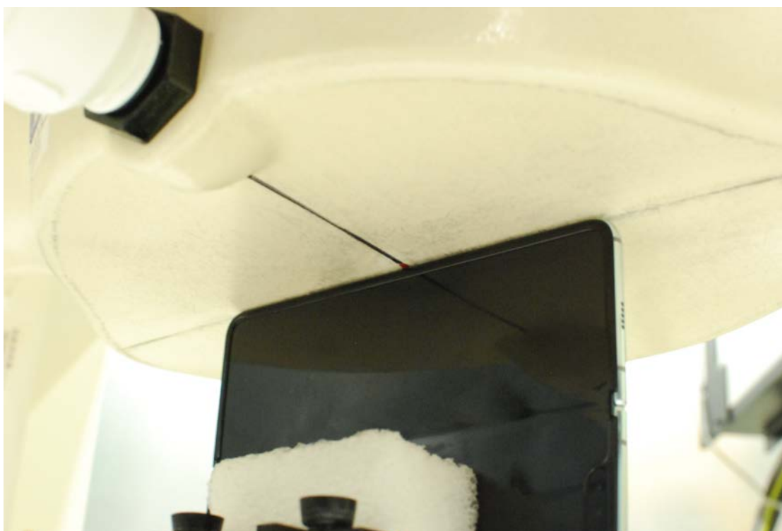
SAR Test Setup Photo 32 – Open Configuration Right Edge at 0.0 cm
