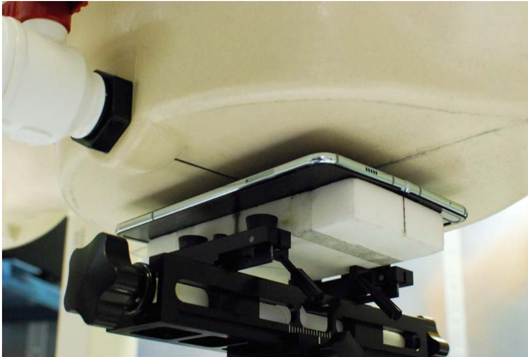
SAR Test Setup Photo 21 – Open Configuration Back Side at 0.8 cm
