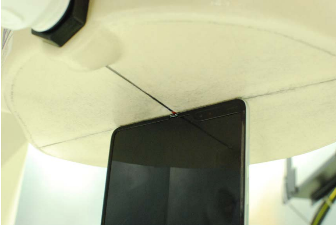
SAR Test Setup Photo 27 – Open Configuration Top Edge at 0.0 cm
