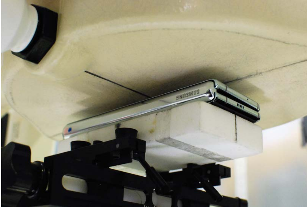
SAR Test Setup Photo 7 – Closed Configuration Back Side at 0.7 cm
