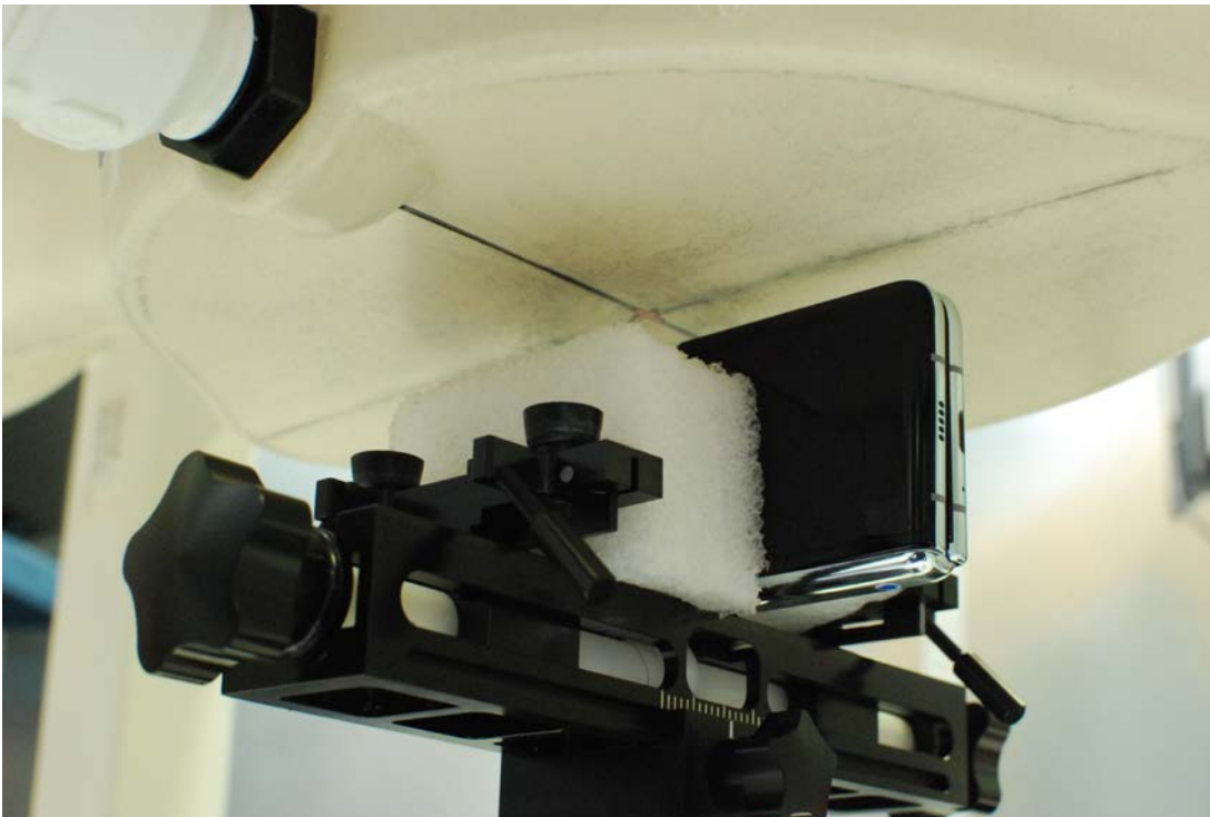
SAR Test Setup Photo 16 – Closed Configuration Right Edge at 1.0cm
