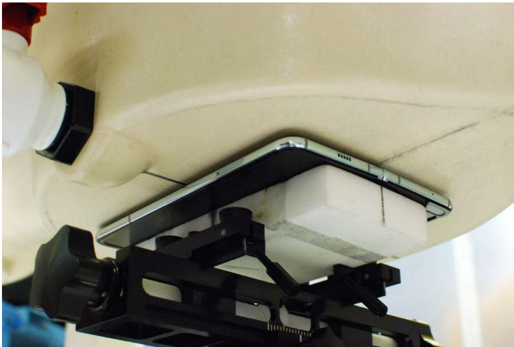
SAR Test Setup Photo 22 – Open Configuration Back Side at 0.0 cm
