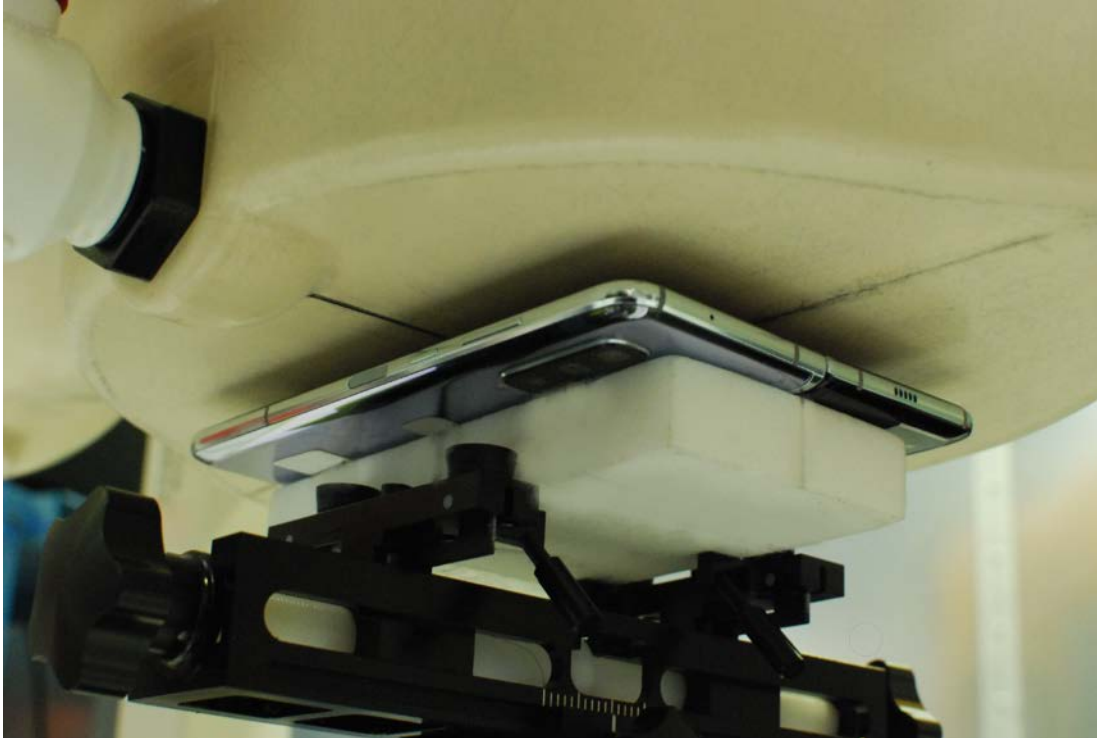
SAR Test Setup Photo 23 – Open Configuration Front Side at 1.0 cm
