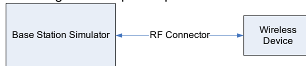
Figure 9-2 Power Measurement Setup
