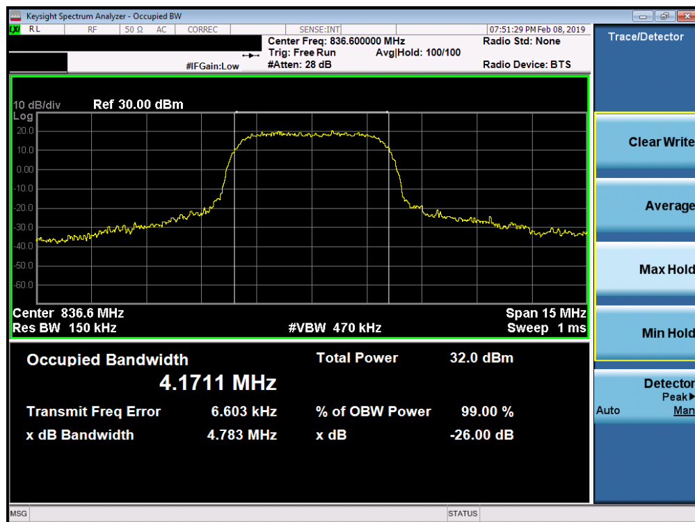
Plot 7-5. Occupied Bandwidth Plot (Cellular WCDMA Mode)
