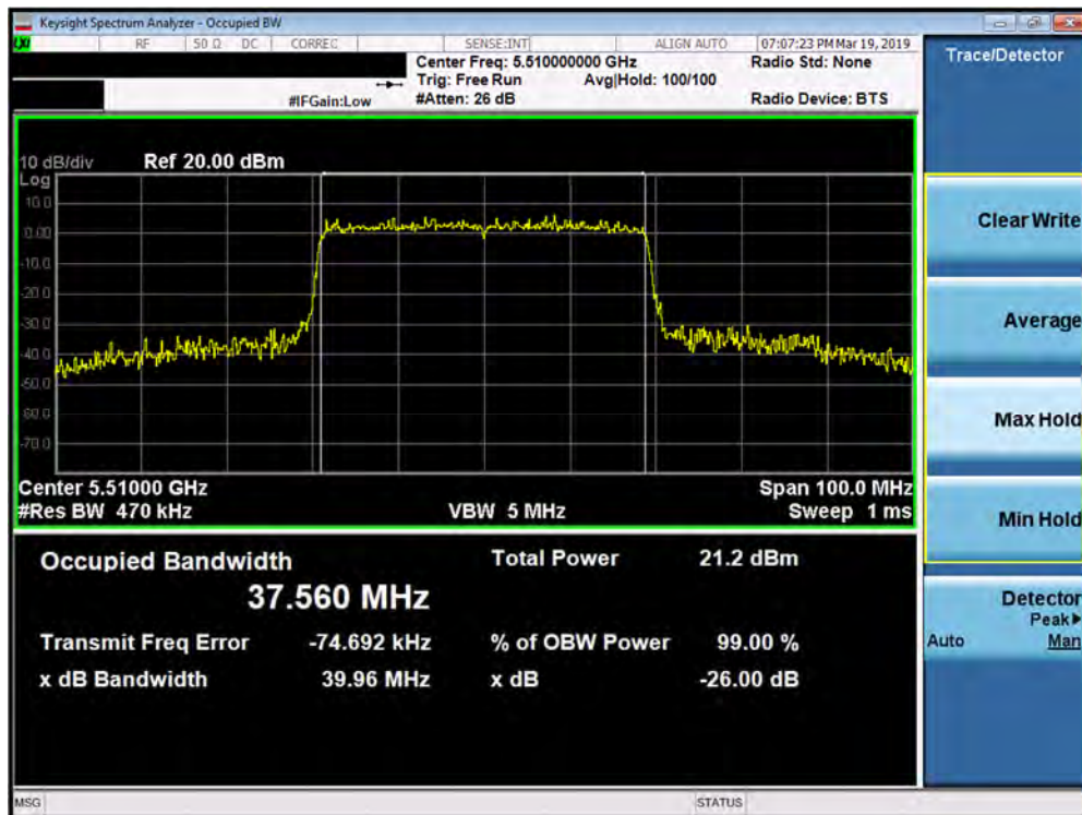
Plot 7-79. 26dB Bandwidth Plot SISO ANT2 (40MHz BW 802.11ax – 26 Tones (UNII Band 2C) – Ch. 102)
