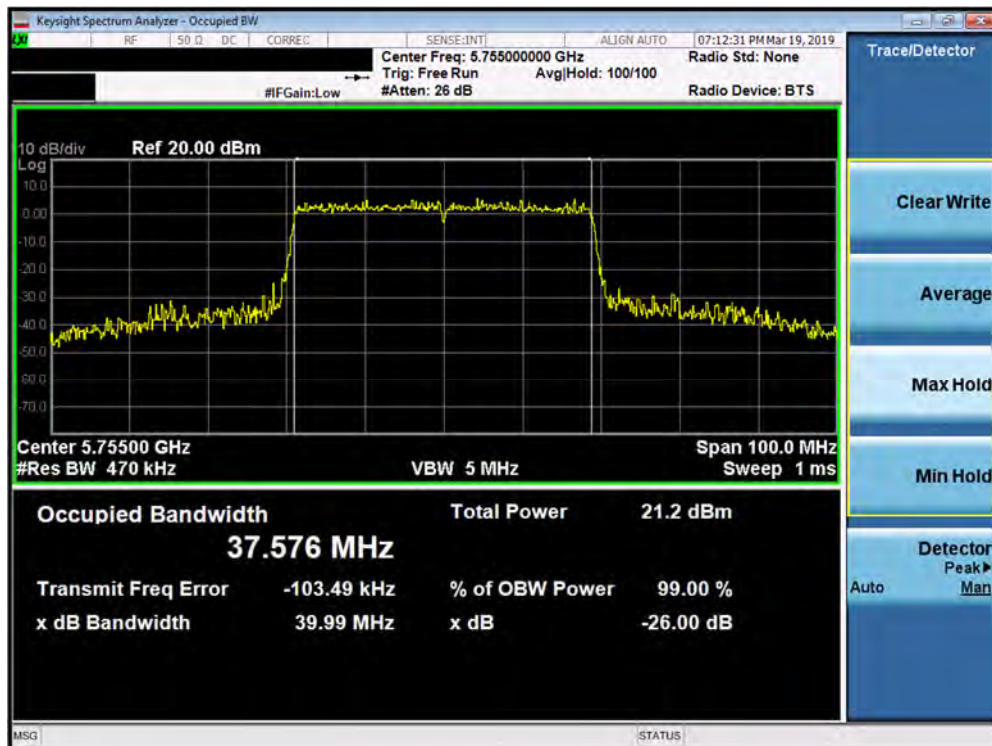
Plot 7-106. 6dB Bandwidth Plot SISO ANT2 (40MHz BW 802.11ax – 484 Tones (UNII Band 3) – Ch. 151)
