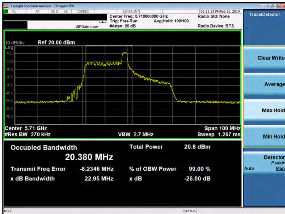
Plot 7-60. 26dB Bandwidth Plot SISO ANT2 (40MHz BW 802.11ax – 26 Tones (UNII Band 2C) – Ch. 142)
