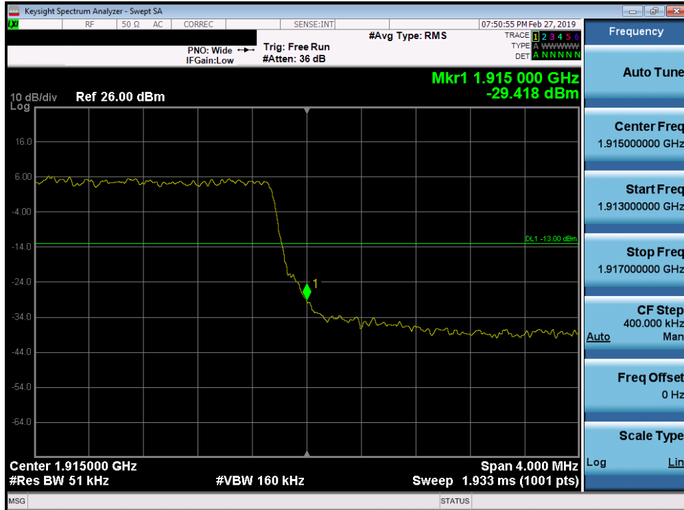
Plot 7-214. Upper Band Edge Plot (Band 25 - 5.0MHz QPSK - Full RB Configuration)
