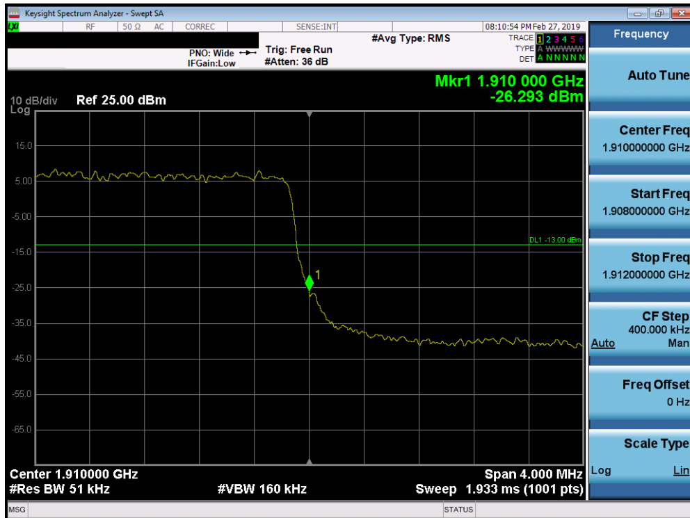
Plot 7-206. Upper Band Edge Plot (Band 2 – 3.0MHz QPSK - Full RB Configuration)
