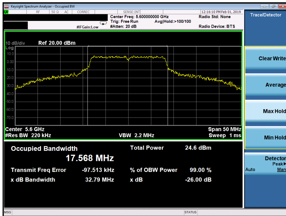
Plot 7-32. 26dB Bandwidth Plot SISO ANT1 (802.11a (UNII Band 2C) – Ch. 120)
