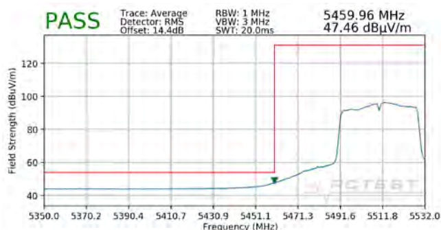
Plot 7-318. Radiated Lower Band Edge Plot SISO ANT1 (Average – UNII Band 2C)
