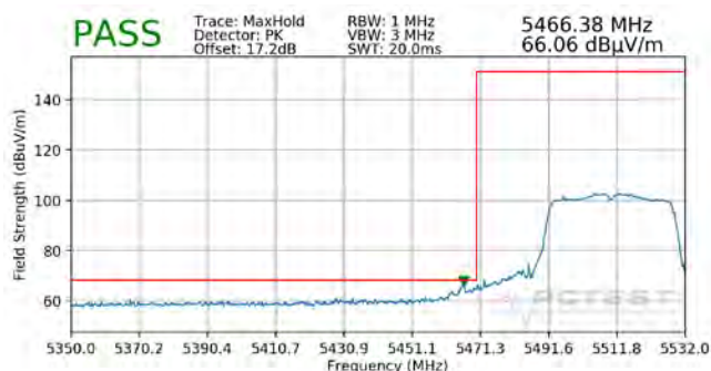
Plot 7-342. Radiated Lower Band Edge Plot SISO ANT2 (Peak - UNII Band 2C)
