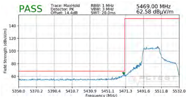
Plot 7-319. Radiated Lower Band Edge Plot SISO ANT1 (Peak – UNII Band 2C)
