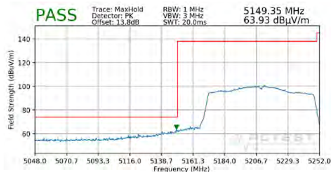
Plot 7-322. Radiated Lower Band Edge Plot SISO ANT1 (Peak - UNII Band 1)
