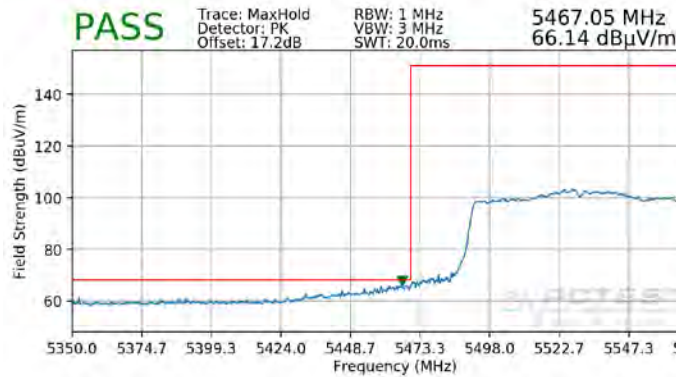
Plot 7-372. Radiated Lower Band Edge Plot MIMO (Peak – UNII Band 2C)
