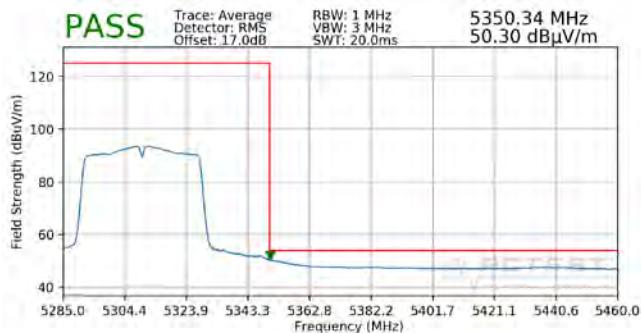
Plot 7-339. Radiated Upper Band Edge Plot SISO ANT2 (Average - UNII Band 2A)
