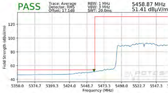
Plot 7-371. Radiated Lower Band Edge Plot MIMO (Average – UNII Band 2C)
