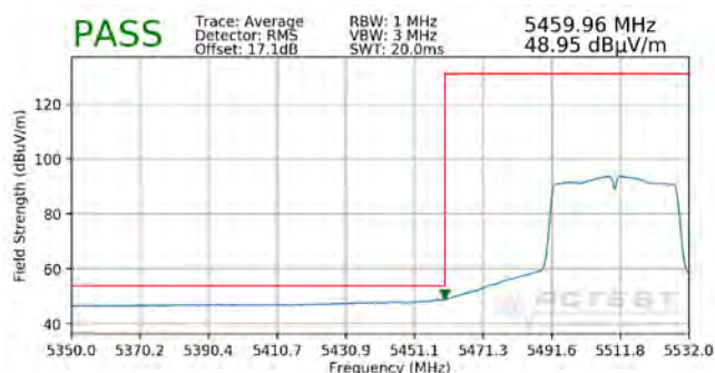
Plot 7-341. Radiated Lower Band Edge Plot SISO ANT2 (Average - UNII Band 2C)
