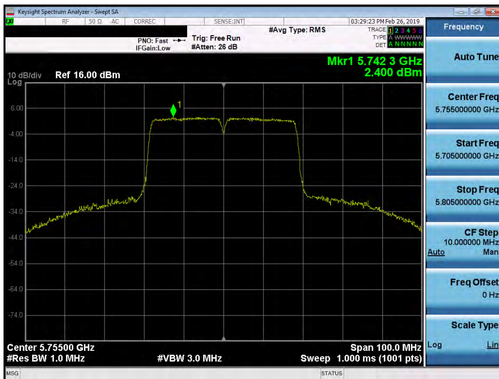
Plot 7-259. Power Spectral Density Plot SISO ANT2 (40MHz BW 802.11n (UNII Band 3) – Ch. 151)
