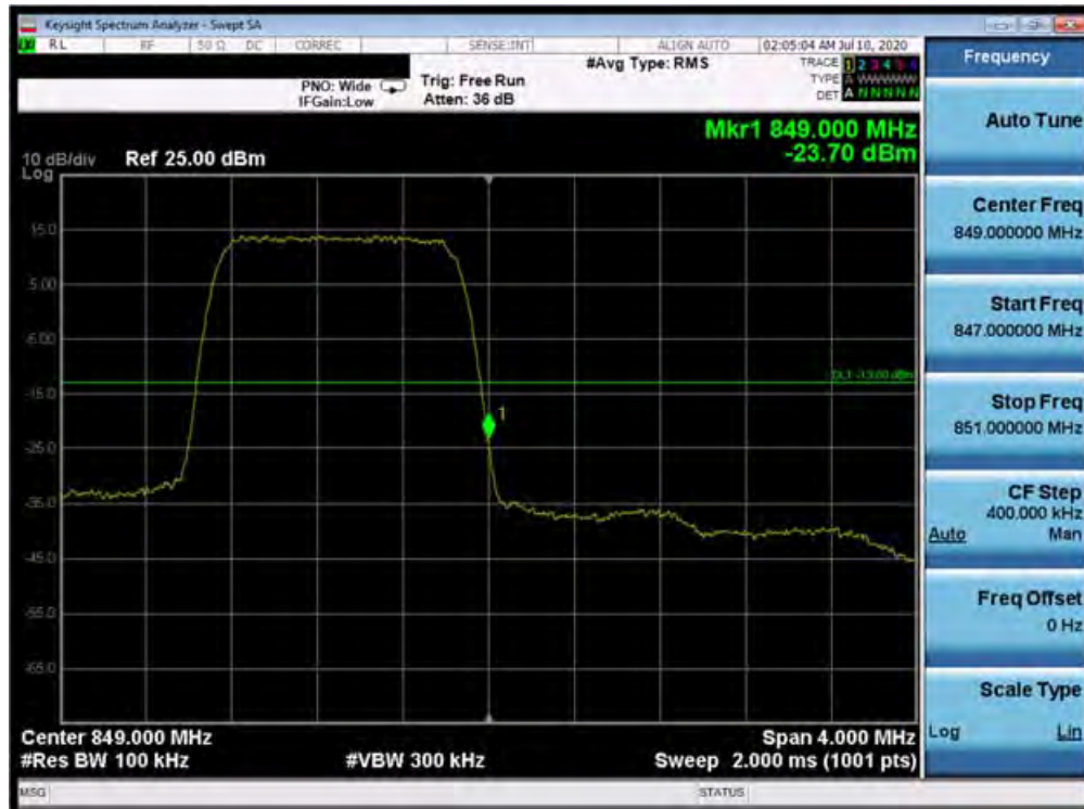
Plot 7-104. Upper Band Edge Plot (Band 5 - 1.4MHz QPSK - Full RB Configuration)
