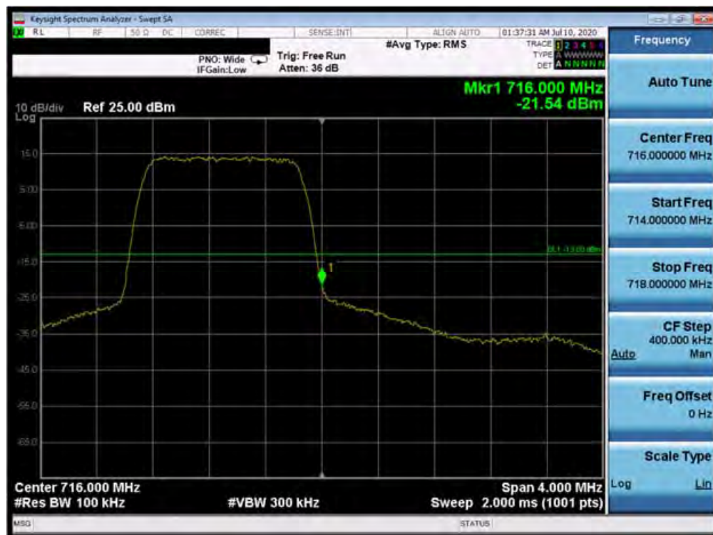
Plot 7-88. Upper Band Edge Plot (Band 12 - 1.4MHz QPSK - Full RB Configuration)
