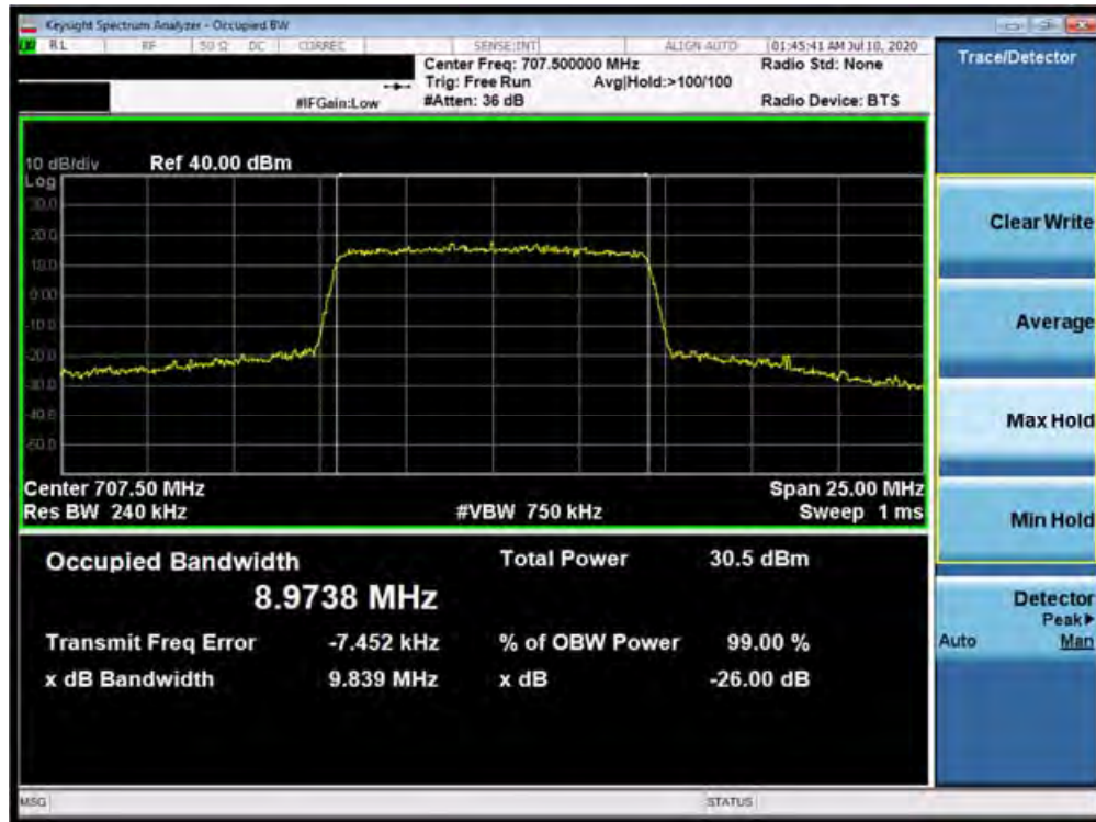
Plot 7-3. Occupied Bandwidth Plot (Band 12 - 10.0MHz 64-QAM - Full RB Configuration)
