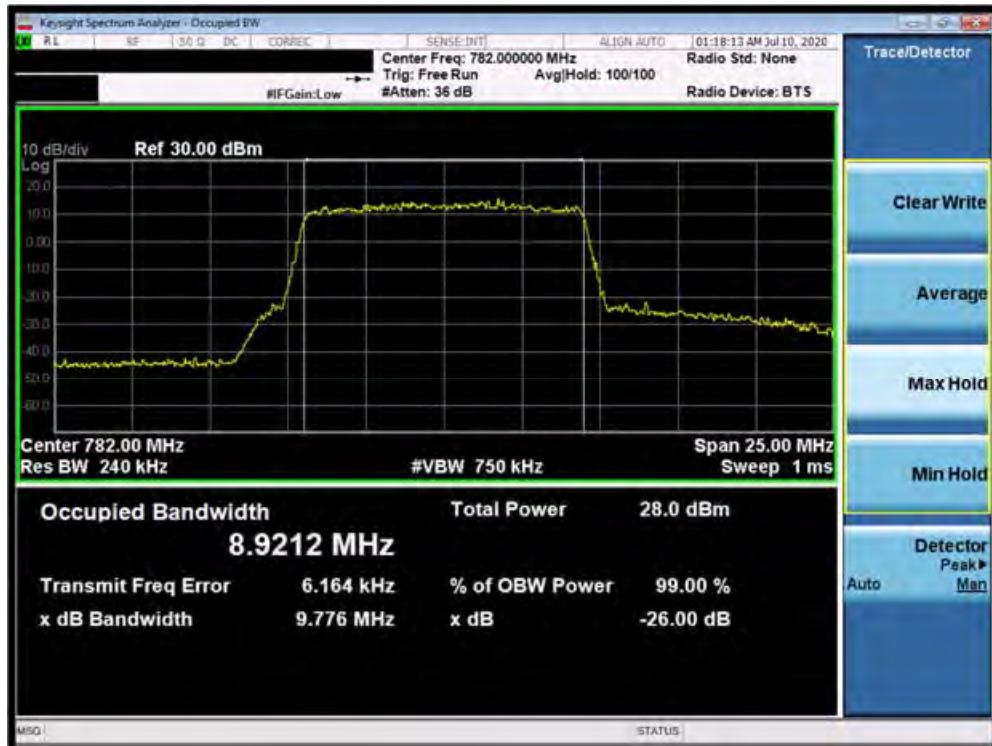
Plot 7-20. Occupied Bandwidth Plot (Band 13 - 10.0MHz 256-QAM - Full RB Configuration)
