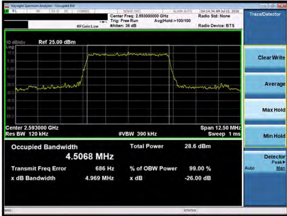
Plot 7-55. Occupied Bandwidth Plot (Band 41 (PC3) - 5.0MHz 64-QAM - Full RB Configuration)
