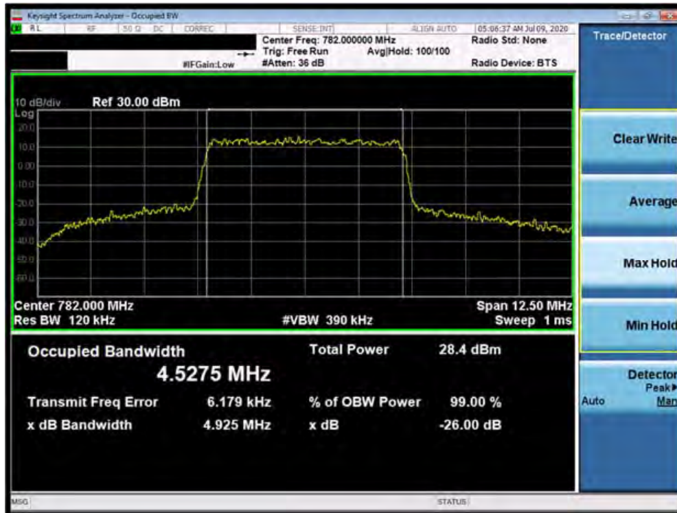
Plot 7-23. Occupied Bandwidth Plot (Band 13 - 5.0MHz 64-QAM - Full RB Configuration)
