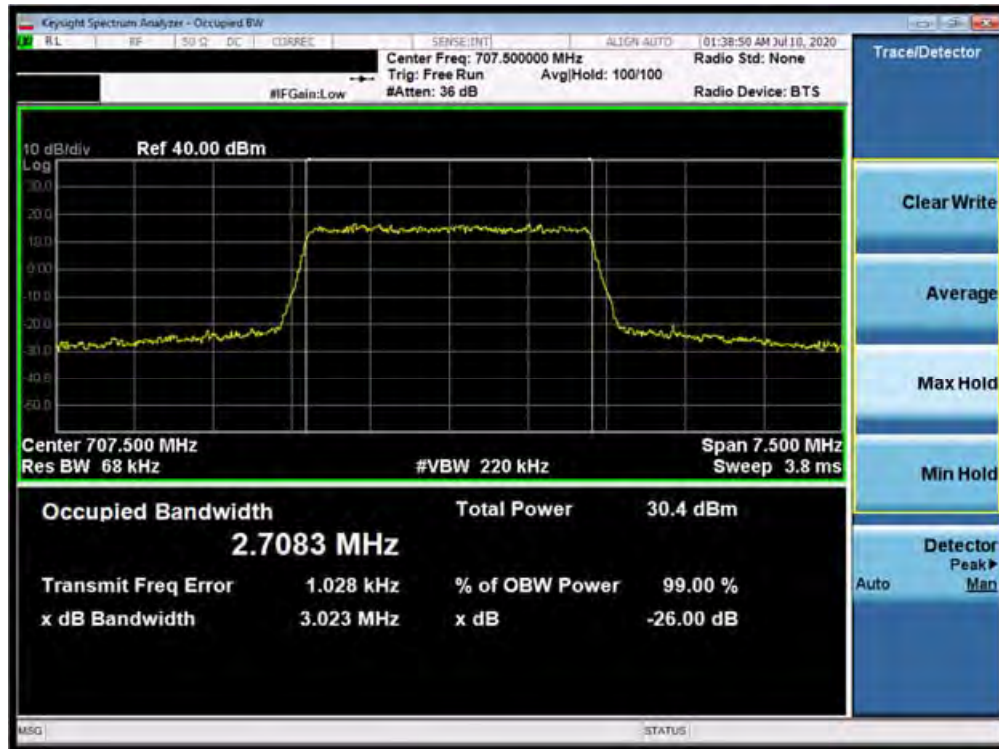
Plot 7-11. Occupied Bandwidth Plot (Band 12 - 3.0MHz 64-QAM - Full RB Configuration)
