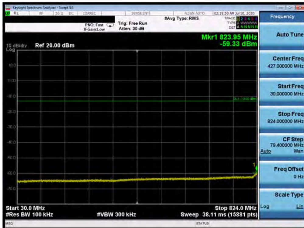
Plot 7-72. Conducted Spurious Plot (Band 5 - 10.0MHz QPSK - RB Size 1, RB Offset 0 - Mid Channel)
