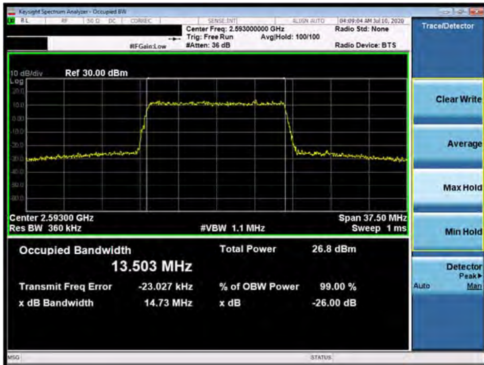
Plot 7-48. Occupied Bandwidth Plot (Band 41 (PC3) - 15.0MHz 256-QAM - Full RB Configuration)
