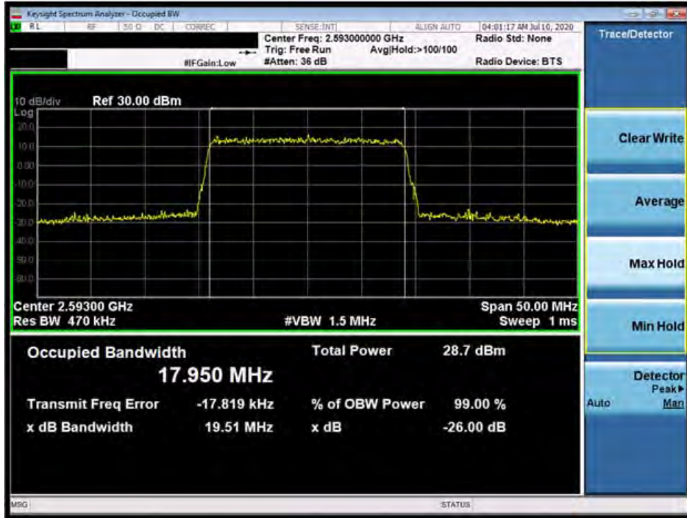
Plot 7-43. Occupied Bandwidth Plot (Band 41 (PC3) - 20.0MHz 64-QAM - Full RB Configuration)
