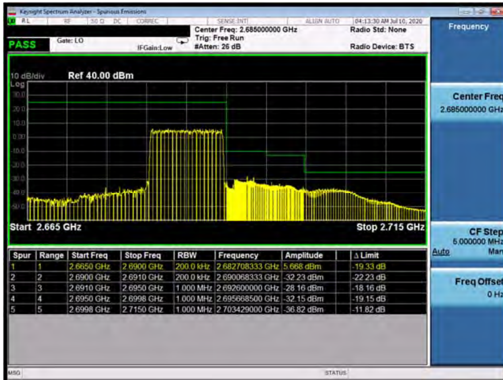
Plot 7-112. Upper ACP Plot (Band 41 PC3- 10.0MHz QPSK - Full RB Configuration)
