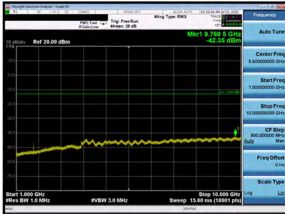
Plot 7-77. Conducted Spurious Plot (Band 5 - 10.0MHz QPSK - RB Size 1, RB Offset 0 - High Channel)
