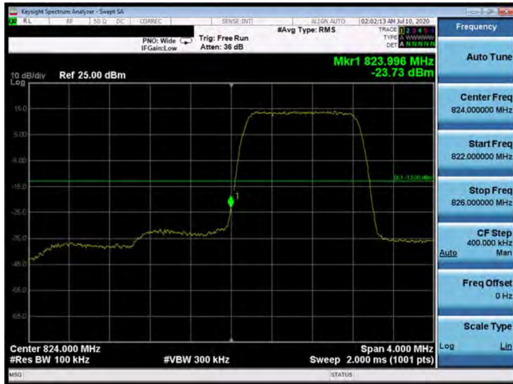
Plot 7-103. Lower Band Edge Plot (Band 5 - 1.4MHz QPSK - Full RB Configuration)
