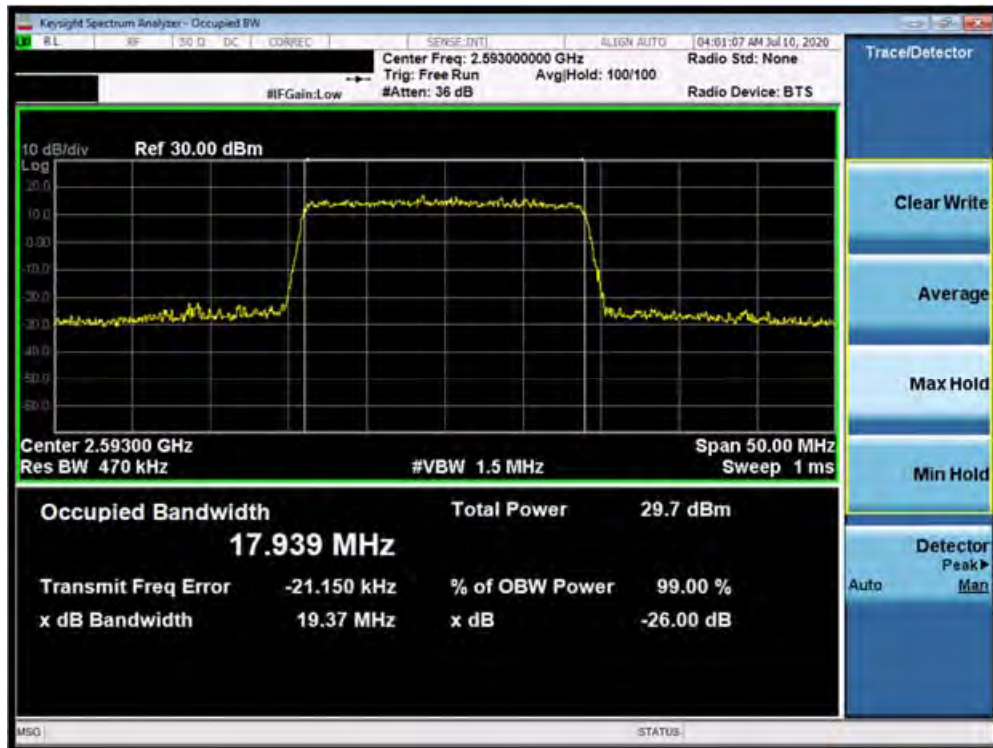
Plot 7-42. Occupied Bandwidth Plot (Band 41 (PC3) - 20.0MHz 16-QAM - Full RB Configuration)
