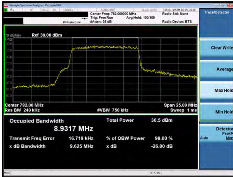
Plot 7-17. Occupied Bandwidth Plot (Band 13 - 10.0MHz QPSK - Full RB Configuration)
