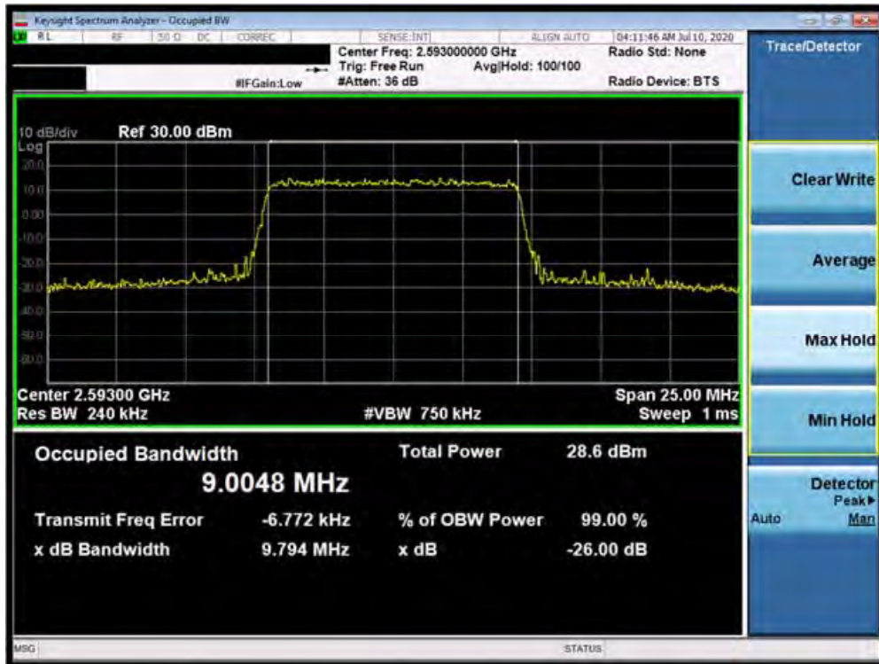
Plot 7-51. Occupied Bandwidth Plot (Band 41 (PC3) - 10.0MHz 64-QAM - Full RB Configuration)
