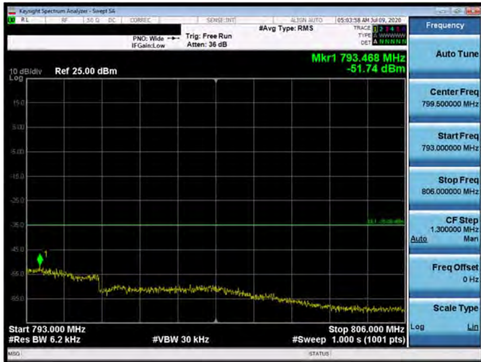
Plot 7-102. Upper Emission Mask Plot (Band 13 - 10.0MHz QPSK - Full RB Configuration)
