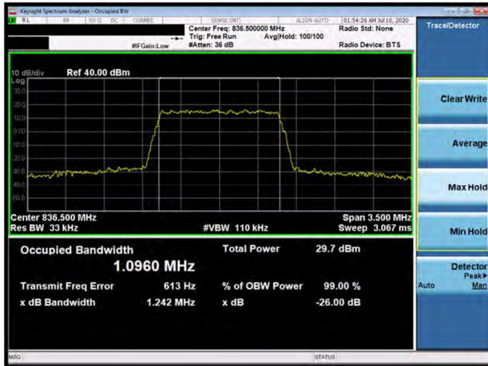
Plot 7-39. Occupied Bandwidth Plot (Band 5 - 1.4MHz 64-QAM - Full RB Configuration)
