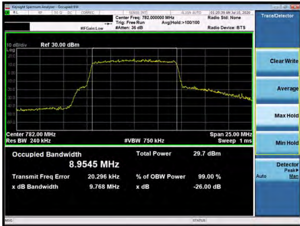
Plot 7-19. Occupied Bandwidth Plot (Band 13 - 10.0MHz 64-QAM - Full RB Configuration)
