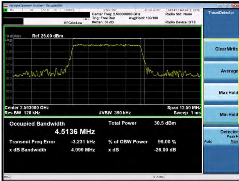
Plot 7-53. Occupied Bandwidth Plot (Band 41 (PC3) - 5.0MHz QPSK - Full RB Configuration)
