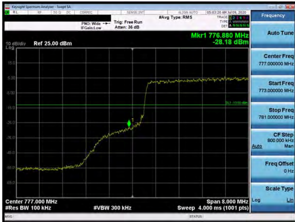
Plot 7-99. Lower Band Edge Plot (Band 13 - 10.0MHz QPSK - Full RB Configuration)
