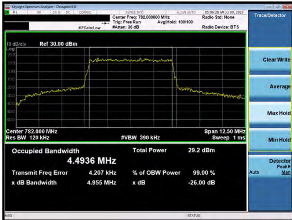
Plot 7-22. Occupied Bandwidth Plot (Band 13 - 5.0MHz 16-QAM - Full RB Configuration)
