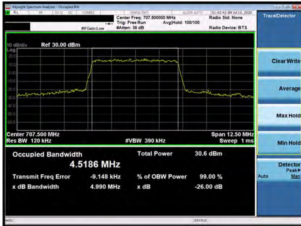
Plot 7-7. Occupied Bandwidth Plot (Band 12 - 5.0MHz 64-QAM - Full RB Configuration)
