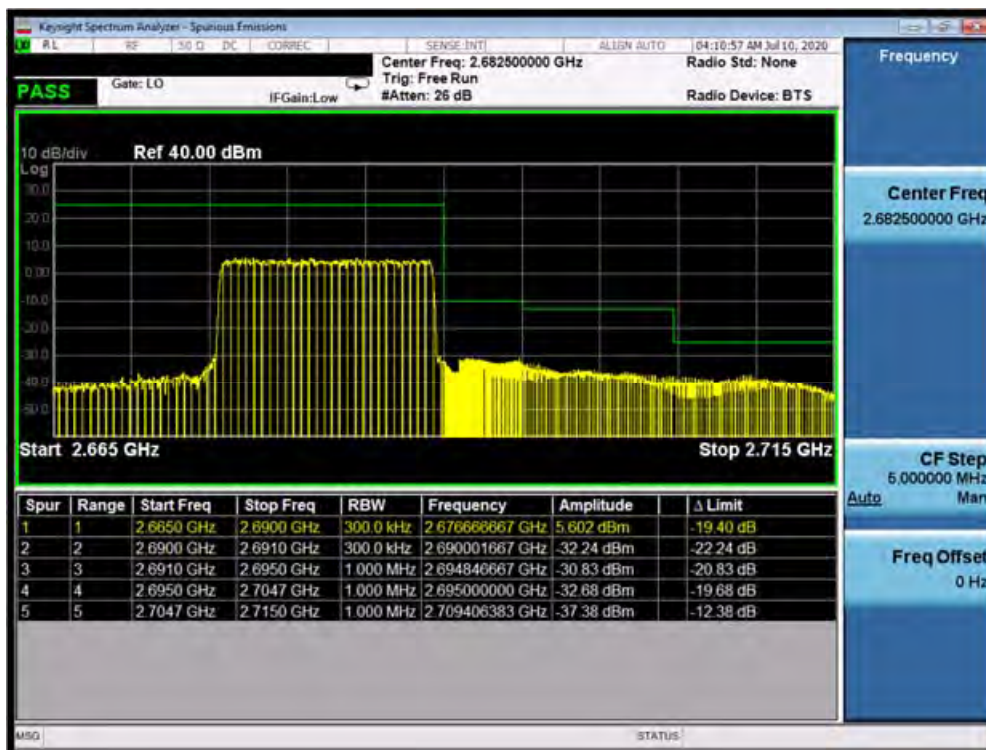
Plot 7-114. Upper ACP Plot (Band 41 PC3- 15.0MHz QPSK - Full RB Configuration)
