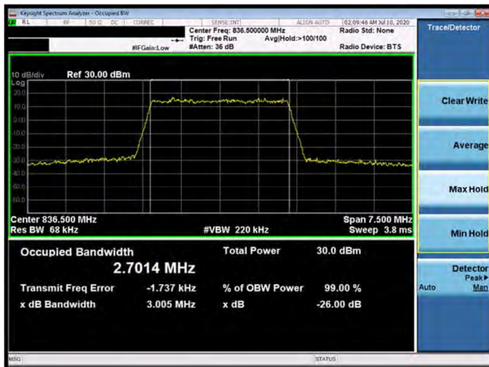
Plot 7-35. Occupied Bandwidth Plot (Band 5 - 3.0MHz 64-QAM - Full RB Configuration)
