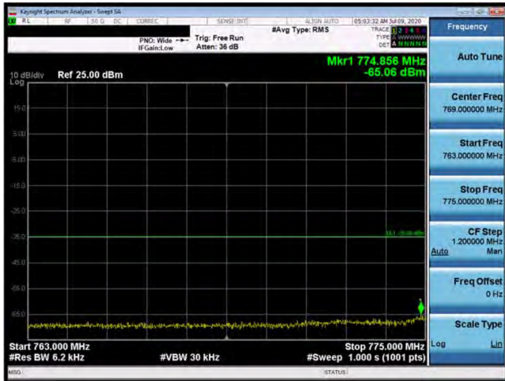
Plot 7-100. Lower Emission Mask Plot (Band 13 - 10.0MHz QPSK - Full RB Configuration)
