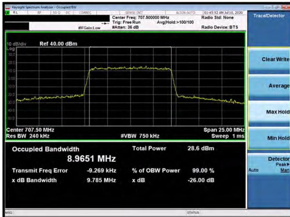
Plot 7-4. Occupied Bandwidth Plot (Band 12 - 10.0MHz 256-QAM - Full RB Configuration)
