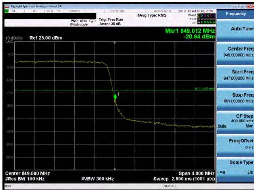
Plot 7-106. Upper Band Edge Plot (Band 5 - 3.0MHz QPSK - Full RB Configuration)
