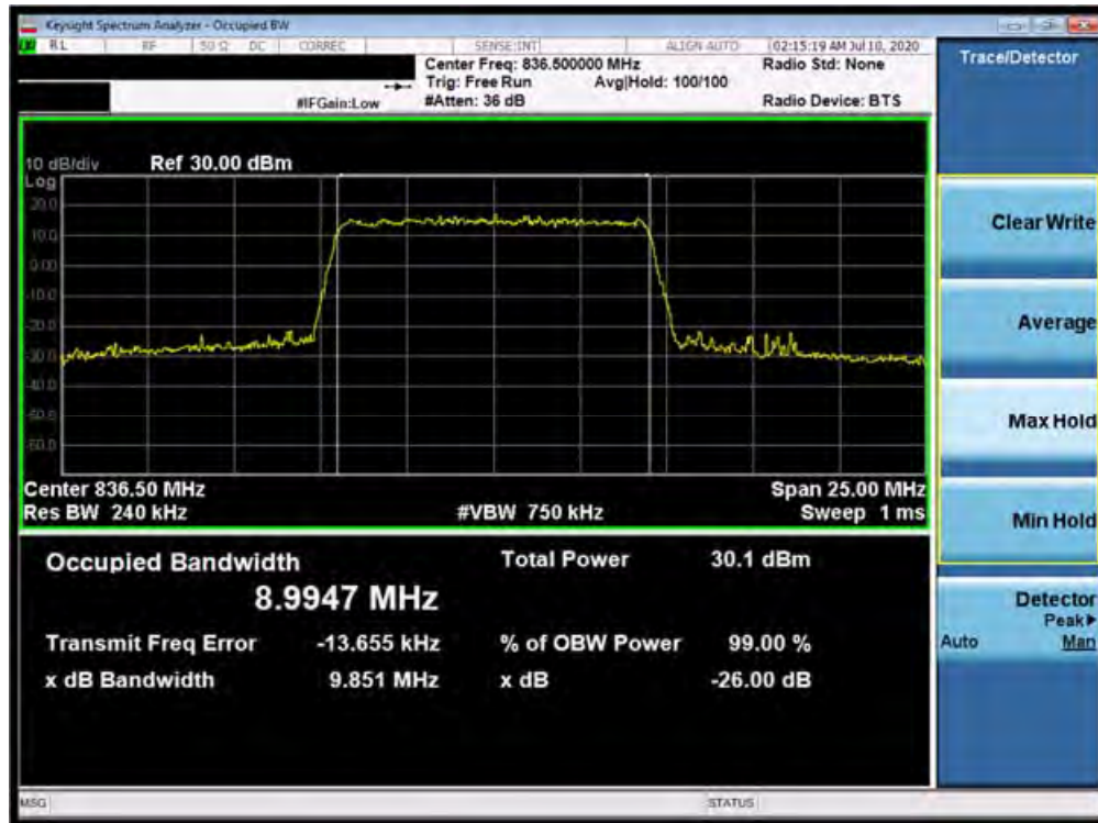
Plot 7-27. Occupied Bandwidth Plot (Band 5 - 10.0MHz 64-QAM - Full RB Configuration)
