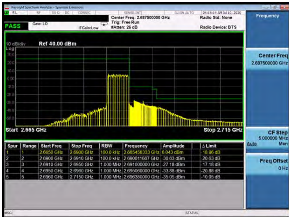
Plot 7-110. Upper ACP Plot (Band 41 PC3- 5.0MHz QPSK - Full RB Configuration)
