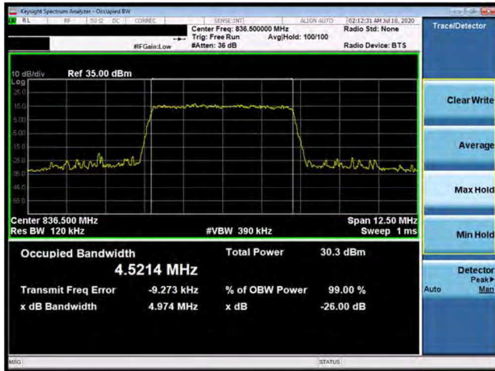
Plot 7-31. Occupied Bandwidth Plot (Band 5 - 5.0MHz 64-QAM - Full RB Configuration)
