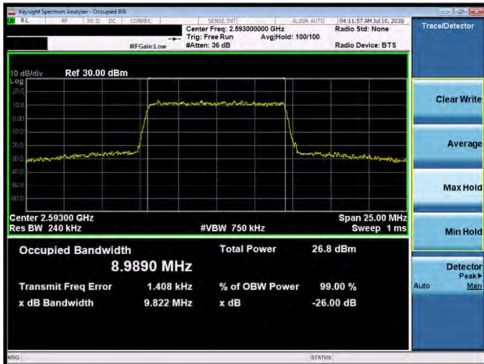
Plot 7-52. Occupied Bandwidth Plot (Band 41 (PC3) - 10.0MHz 256-QAM - Full RB Configuration)
