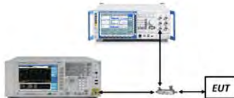
Figure 7-2. Test Instrument & Measurement Setup
