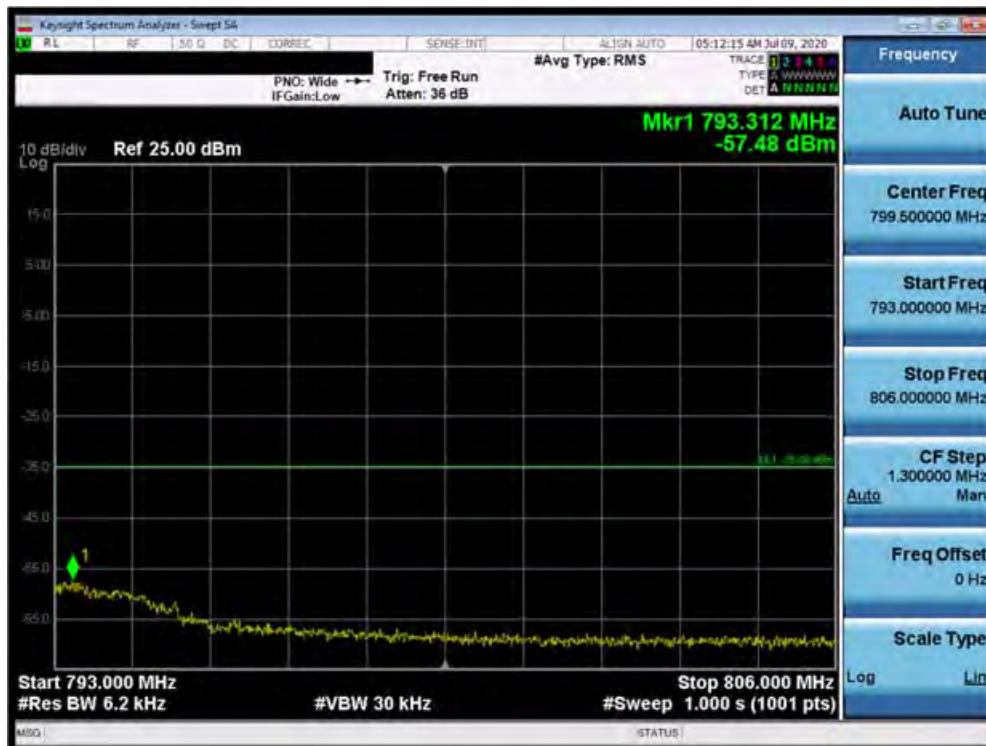
Plot 7-98. Upper Emission Mask Plot (Band 13 - 5.0MHz QPSK - Full RB Configuration)
