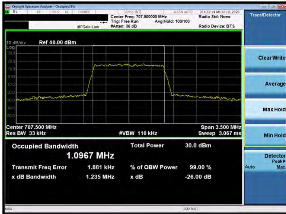
Plot 7-15. Occupied Bandwidth Plot (Band 12 - 1.4MHz 64-QAM - Full RB Configuration)
