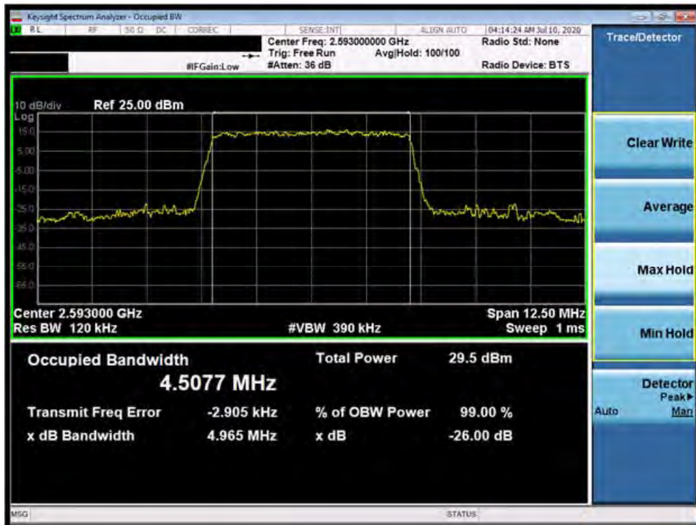
Plot 7-54. Occupied Bandwidth Plot (Band 41 (PC3) - 5.0MHz 16-QAM - Full RB Configuration)
