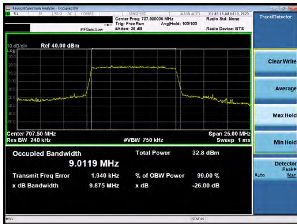
Plot 7-1. Occupied Bandwidth Plot (Band 12 - 10.0MHz QPSK - Full RB Configuration)
