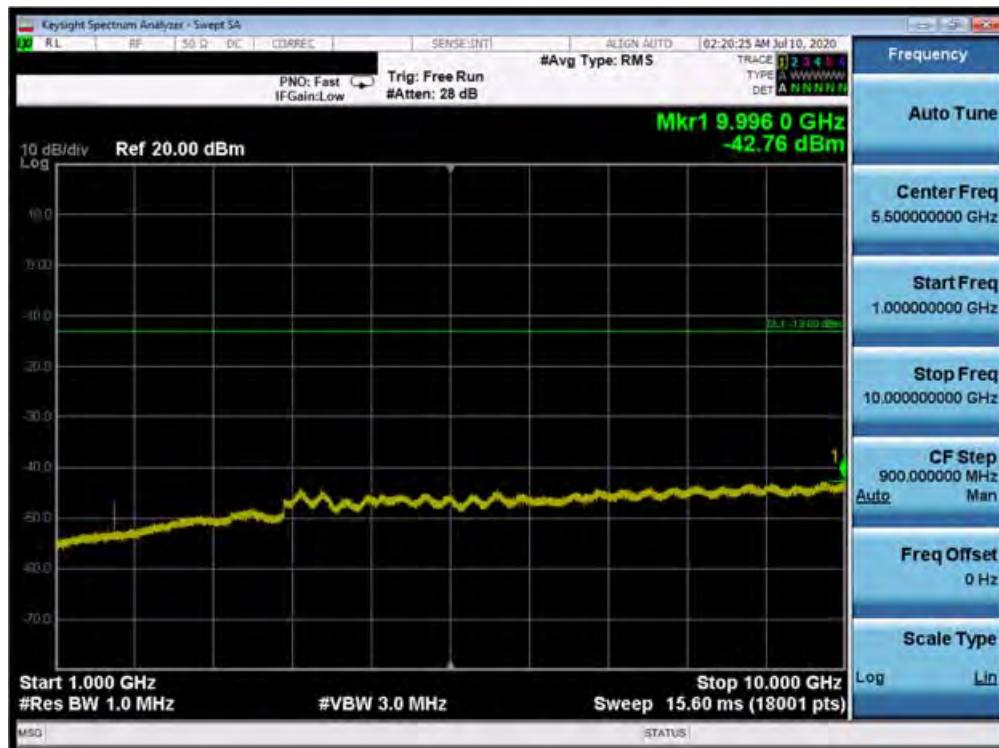
Plot 7-74. Conducted Spurious Plot (Band 5 - 10.0MHz QPSK - RB Size 1, RB Offset 0 - Mid Channel)
