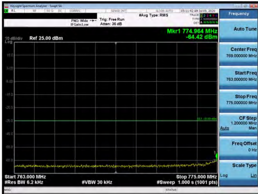
Plot 7-96. Lower Emission Mask Plot (Band 13 - 5.0MHz QPSK - Full RB Configuration)
