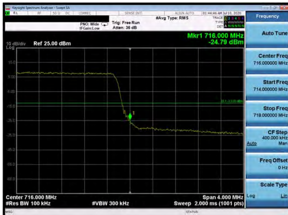
Plot 7-92. Upper Band Edge Plot (Band 12 - 5.0MHz QPSK - Full RB Configuration)
