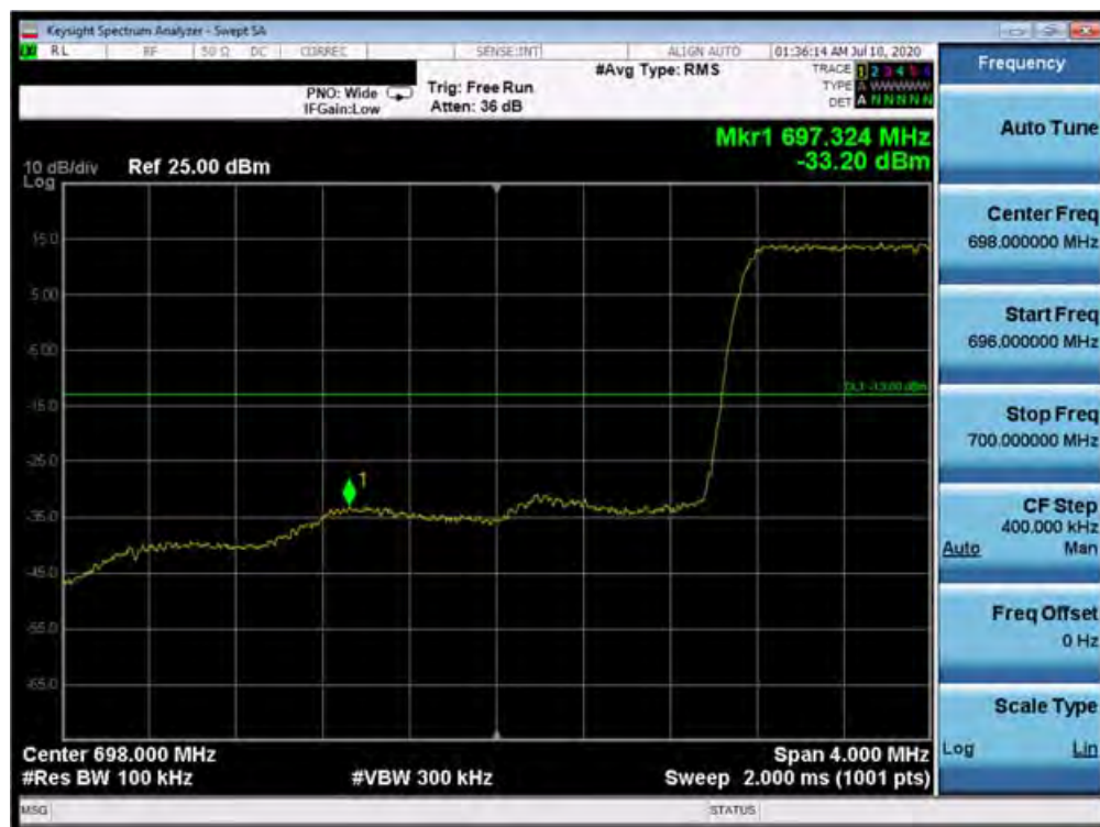
Plot 7-87. Lower Band Edge Plot (Band 12 - 1.4MHz QPSK - Full RB Configuration)
