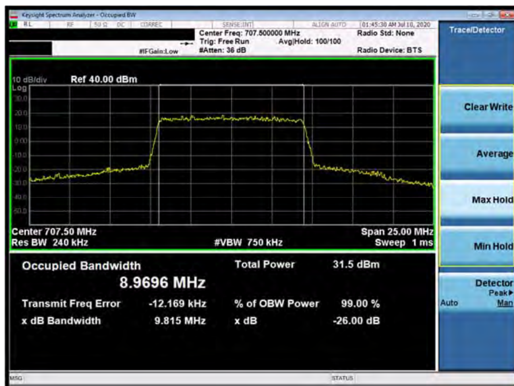
Plot 7-2. Occupied Bandwidth Plot (Band 12 - 10.0MHz 16-QAM - Full RB Configuration)
