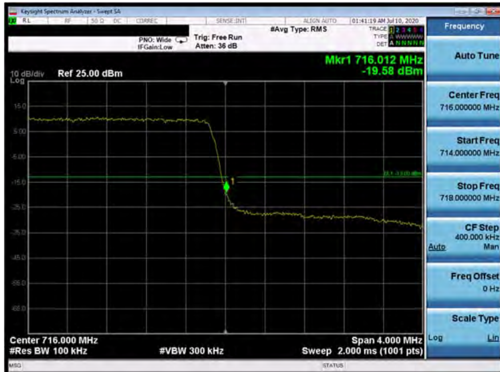
Plot 7-90. Upper Band Edge Plot (Band 12 - 3.0MHz QPSK - Full RB Configuration)
