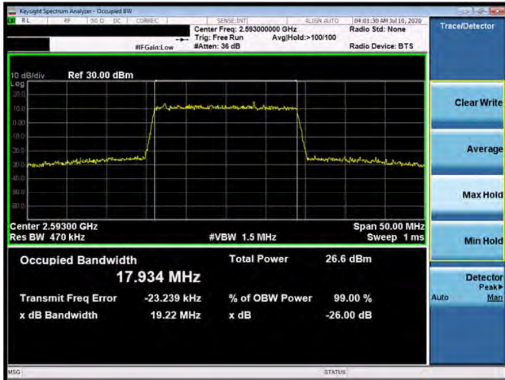
Plot 7-44. Occupied Bandwidth Plot (Band 41 (PC3) - 20.0MHz 256-QAM - Full RB Configuration)
