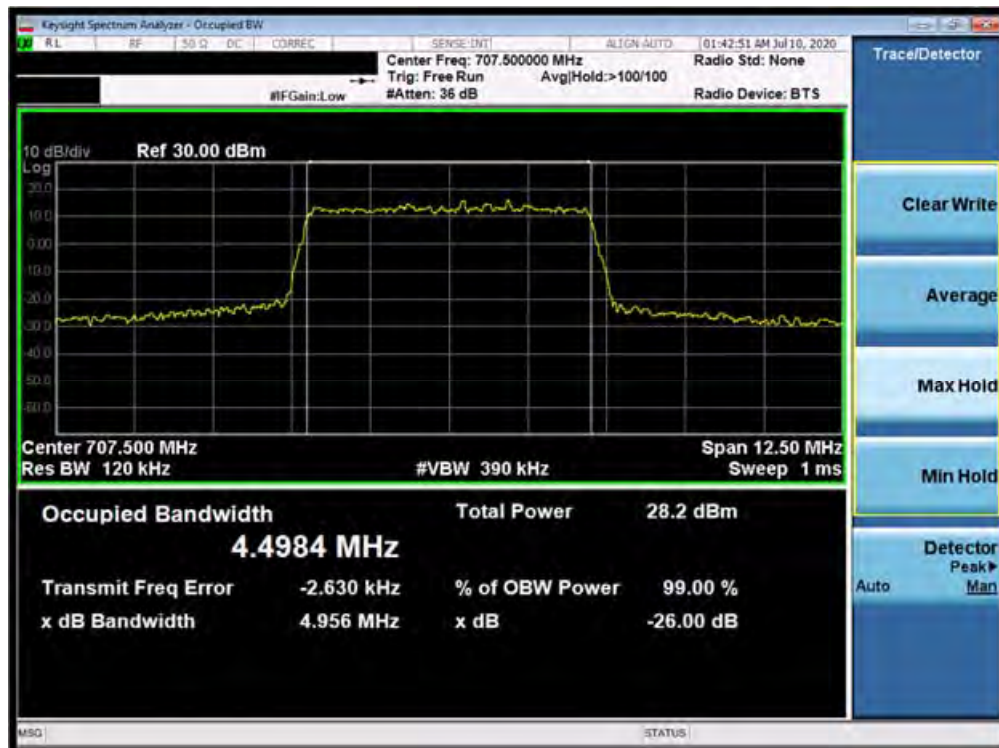
Plot 7-8. Occupied Bandwidth Plot (Band 12 - 5.0MHz 256-QAM - Full RB Configuration)
