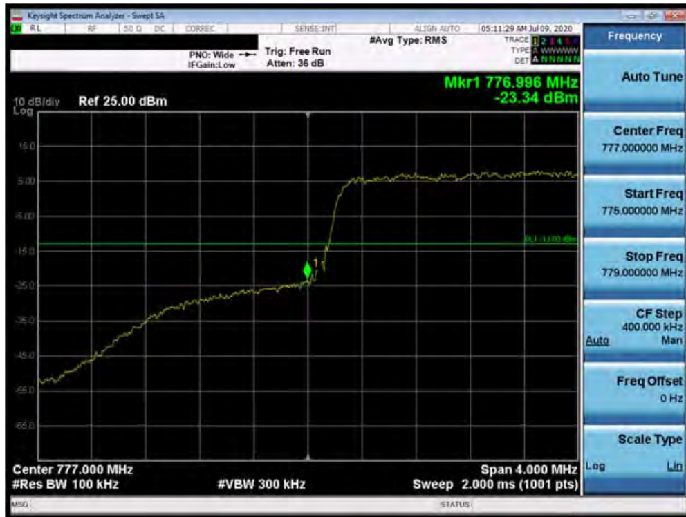
Plot 7-95. Lower Band Edge Plot (Band 13 - 5.0MHz QPSK - Full RB Configuration)
