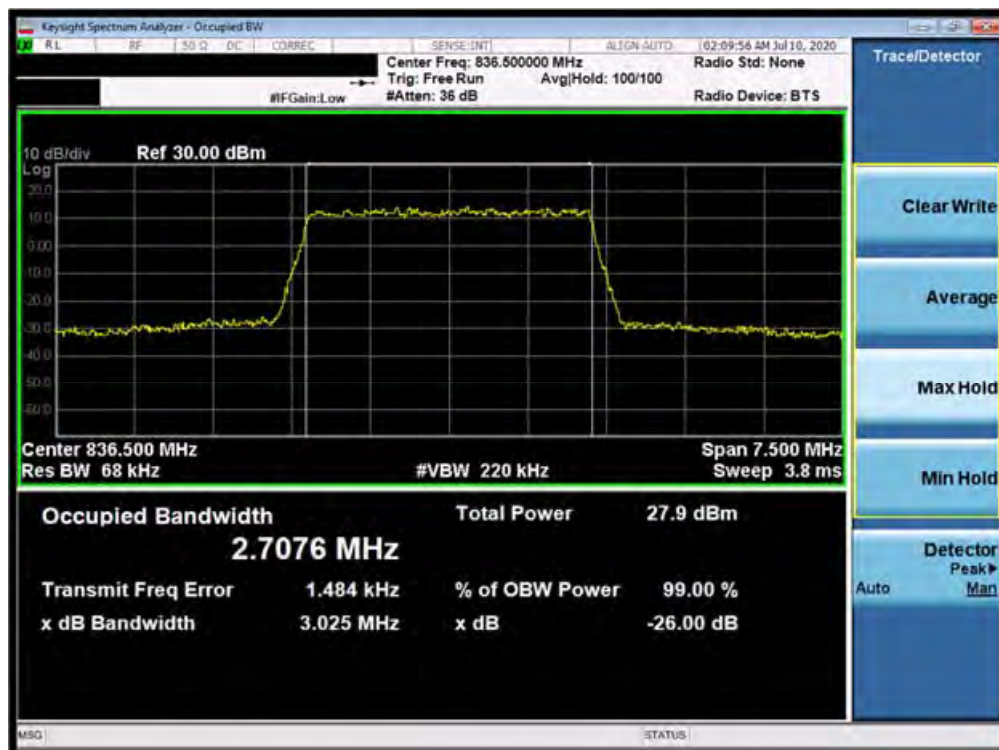
Plot 7-36. Occupied Bandwidth Plot (Band 5 - 3.0MHz 256-QAM - Full RB Configuration)
