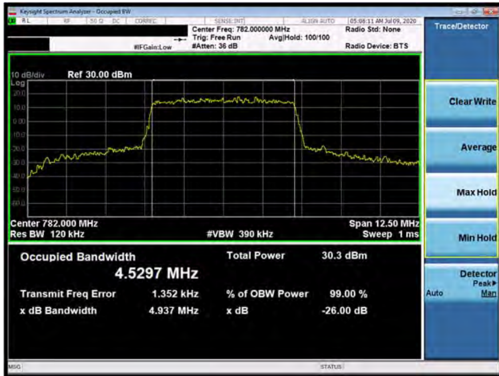
Plot 7-21. Occupied Bandwidth Plot (Band 13 - 5.0MHz QPSK - Full RB Configuration)
