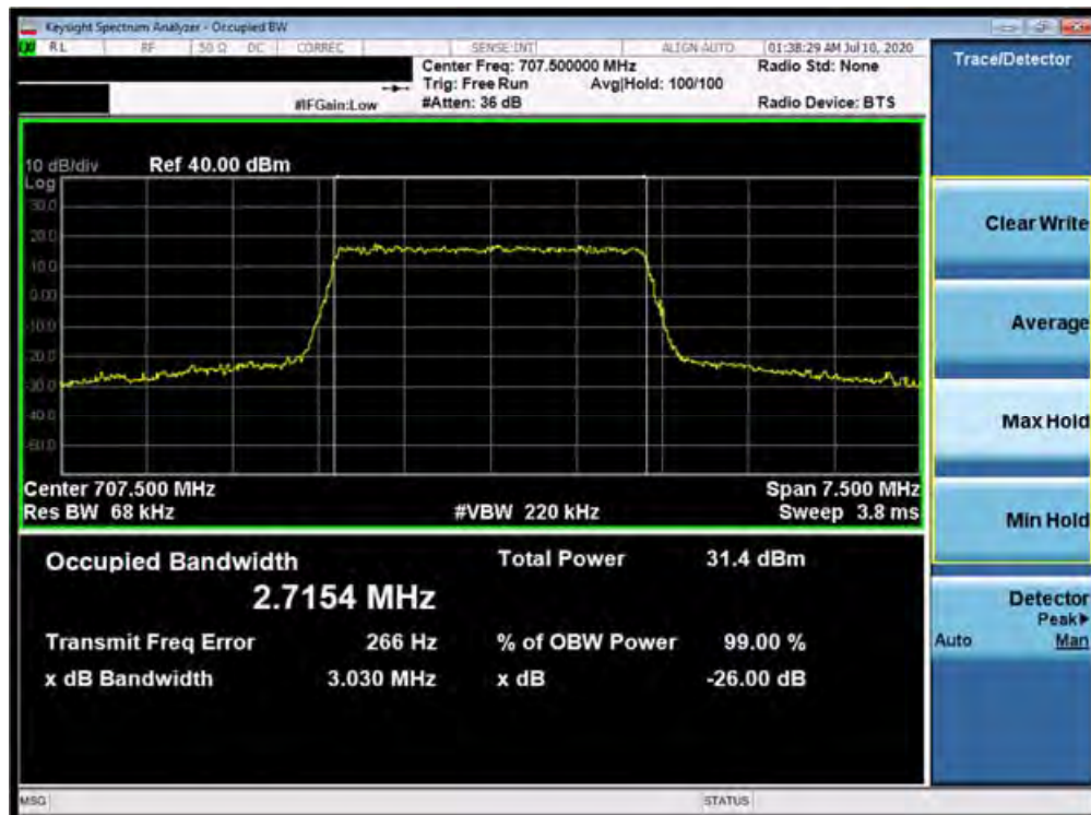
Plot 7-10. Occupied Bandwidth Plot (Band 12 - 3.0MHz 16-QAM - Full RB Configuration)
