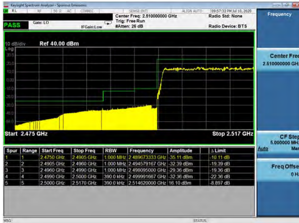
Plot 7-115. Lower ACP Plot at 2496 MHz (Band 41 PC3 - 20.0MHz QPSK - Full RB Configuration)
