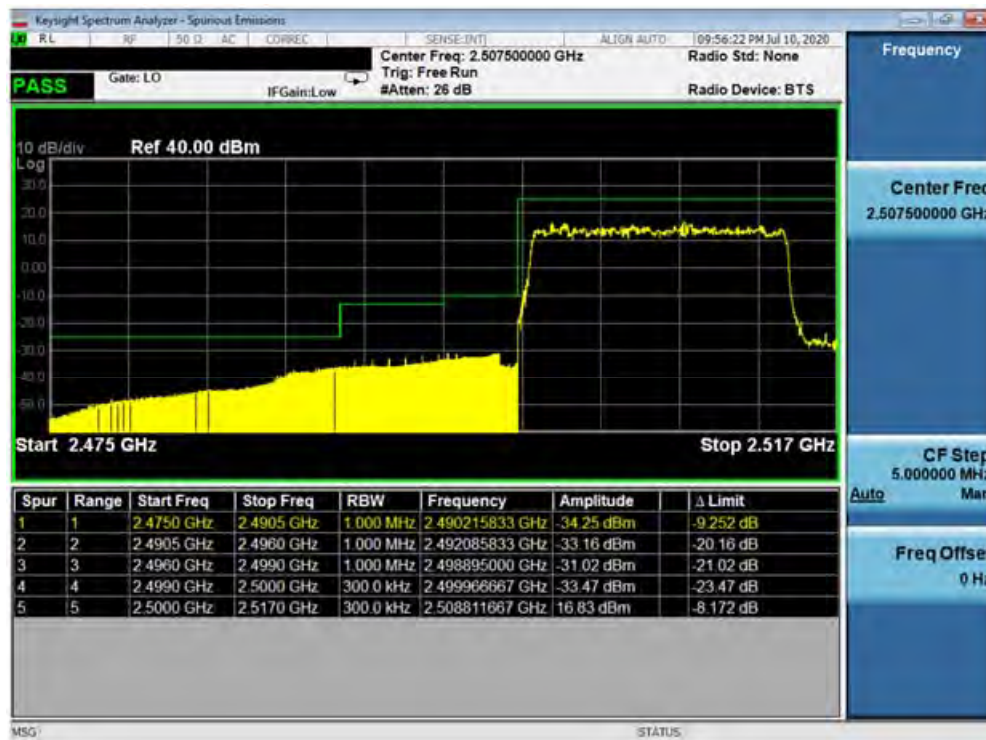
Plot 7-113. Lower ACP Plot at 2500 MHz (Band 41 PC3- 15.0MHz QPSK - Full RB Configuration)
