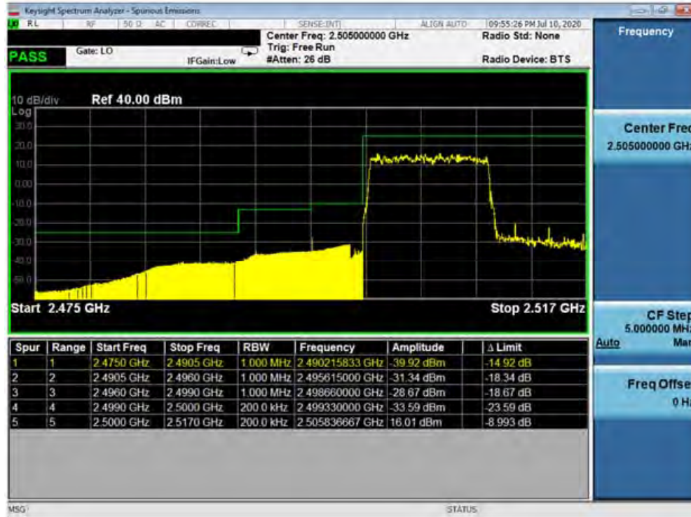
Plot 7-111. Lower ACP Plot at 2500 MHz (Band 41 PC3- 10.0MHz QPSK - Full RB Configuration)
