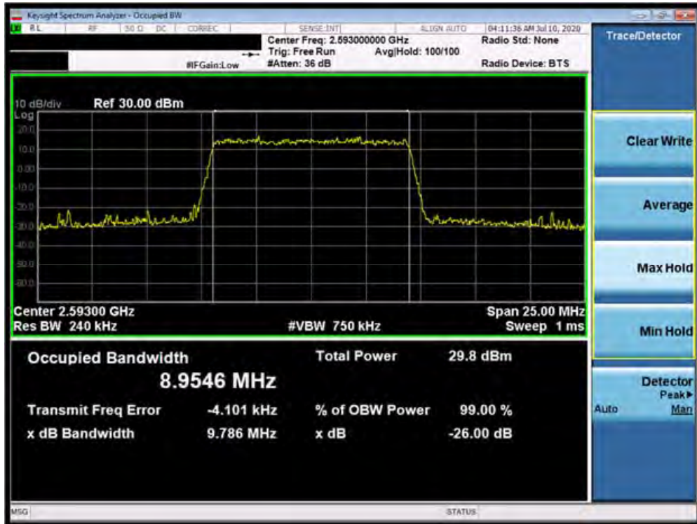
Plot 7-50. Occupied Bandwidth Plot (Band 41 (PC3) - 10.0MHz 16-QAM - Full RB Configuration)
