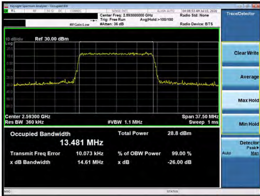
Plot 7-47. Occupied Bandwidth Plot (Band 41 (PC3) - 15.0MHz 64-QAM - Full RB Configuration)
