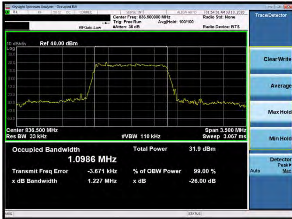
Plot 7-37. Occupied Bandwidth Plot (Band 5 - 1.4MHz QPSK - Full RB Configuration)
