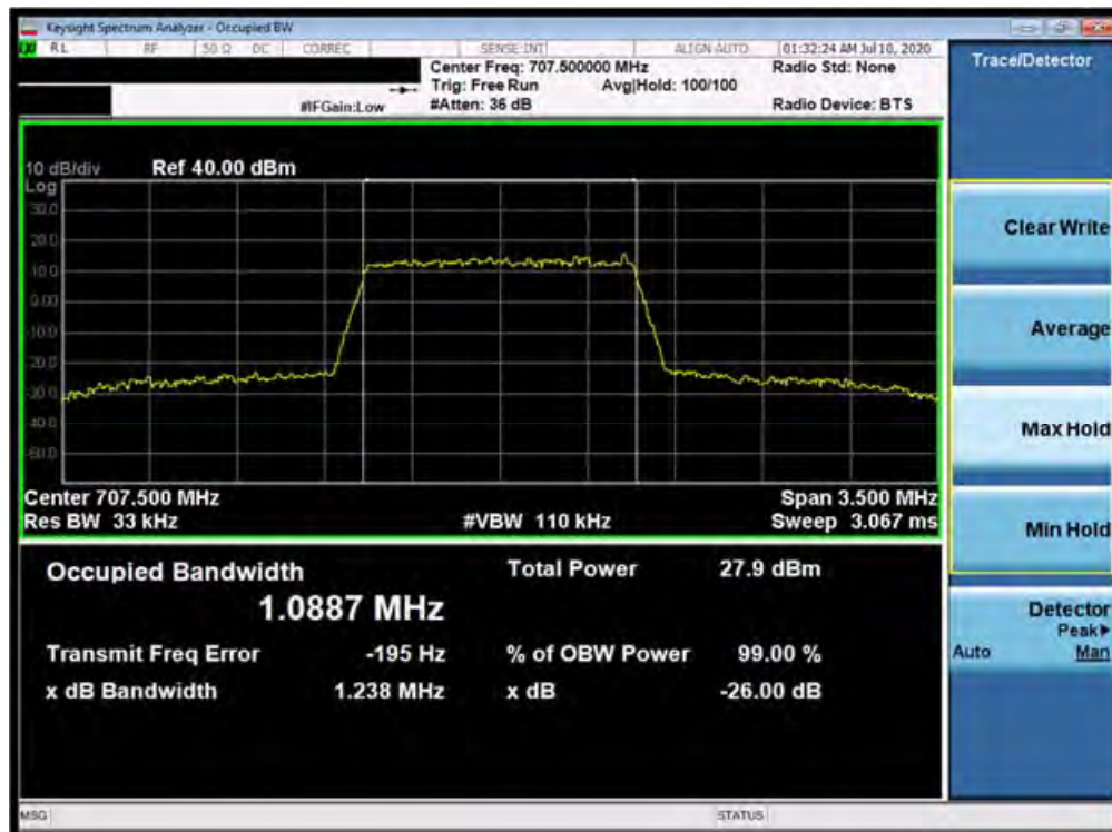
Plot 7-16. Occupied Bandwidth Plot (Band 12 - 1.4MHz 256-QAM - Full RB Configuration)
