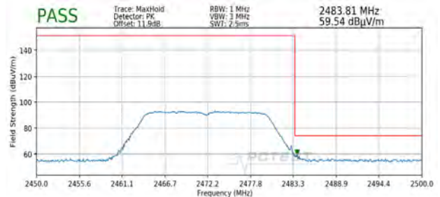
Plot 7-112. Radiated Restricted Upper Band Edge Measurement SISO ANT1 (Peak)
