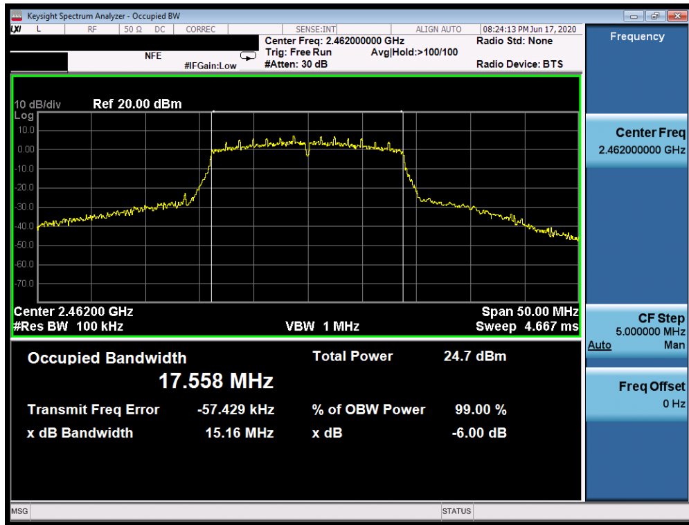
Plot 7-21. 6dB Bandwidth Plot SISO ANT1 (802.11n (2.4GHz) – Ch. 11)
