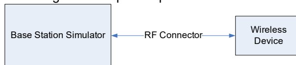
Figure 9-3 Power Measurement Setup
