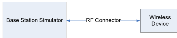
Figure 9-2 Power Measurement Setup
