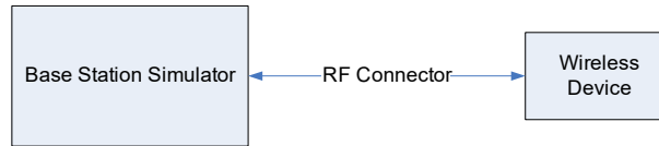
Figure 9-4 Power Measurement Setup
