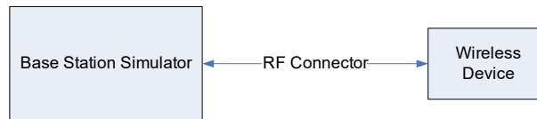
Figure 9-4 Power Measurement Setup
