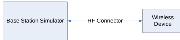
Figure 9-1 Power Measurement Setup
