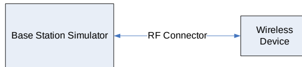
Figure 9-4 Power Measurement Setup
