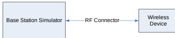
Figure 9-2 Power Measurement Setup
