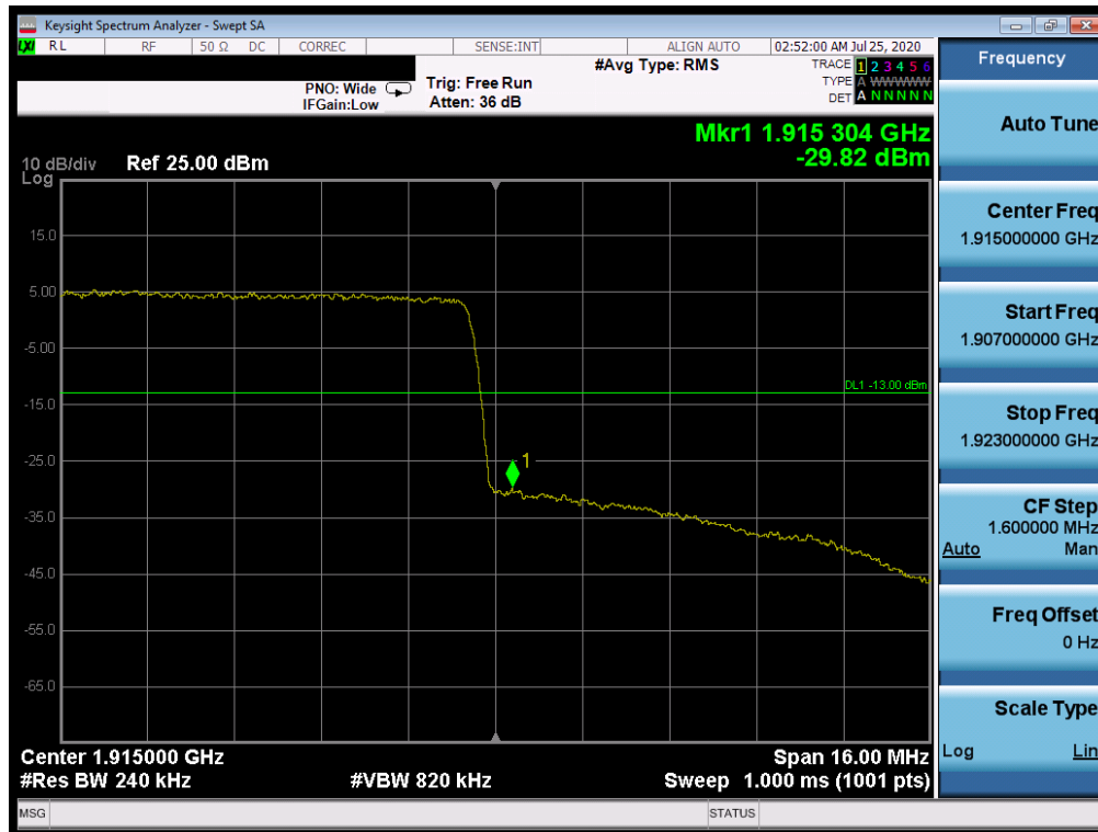
Plot 7-536. Upper Band Edge Plot (NR Band n25 – 20.0MHz - Full RB)
