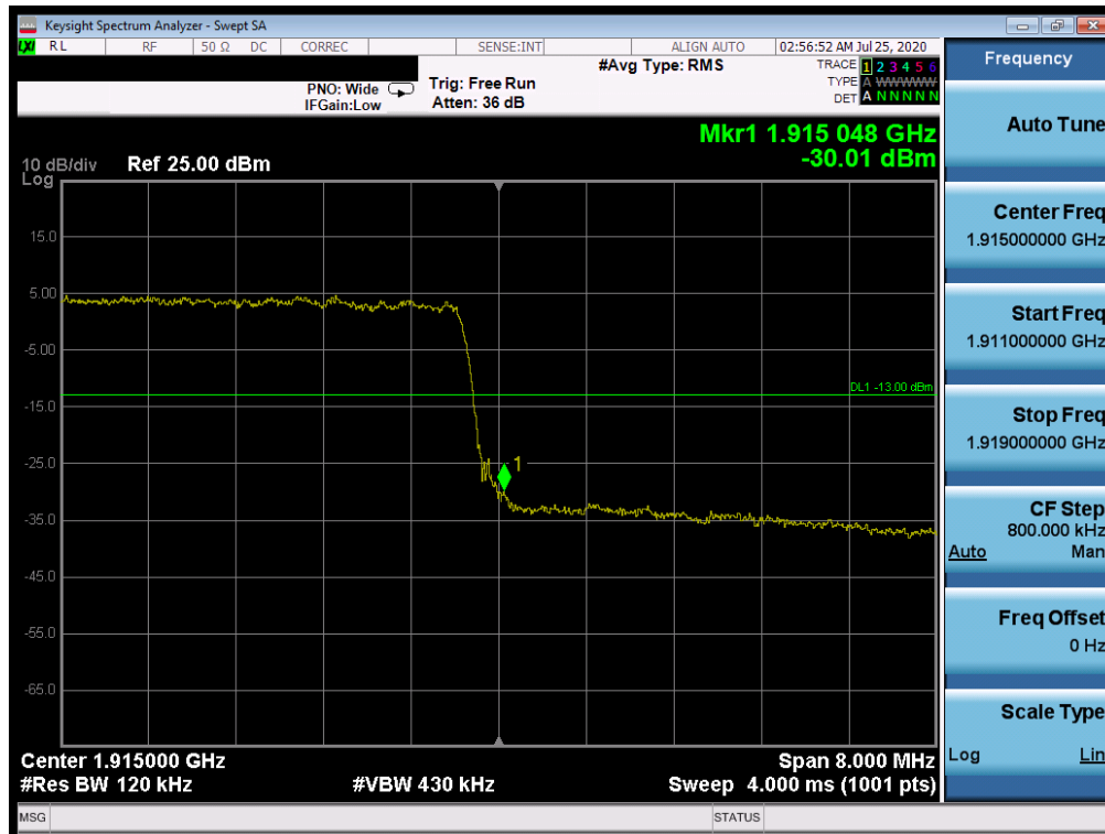
Plot 7-524. Upper Band Edge Plot (NR Band n25 – 10.0MHz - Full RB)
