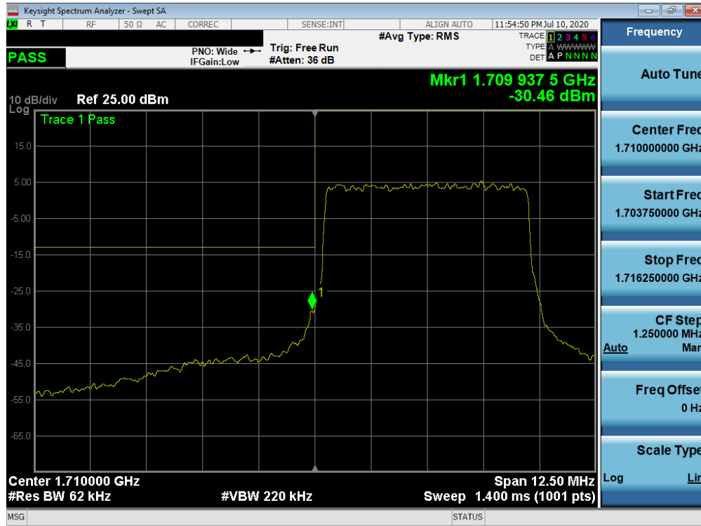
Plot 7-462. Lower Band Edge Plot (NR Band n66 - 5.0MHz - Full RB)
