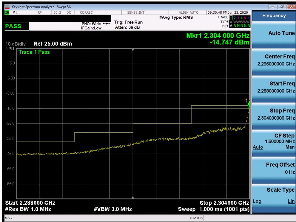
Plot 7-539. Lower Extended Band Edge Plot (Band 30 - 5.0MHz QPSK - Full RB Configuration)
