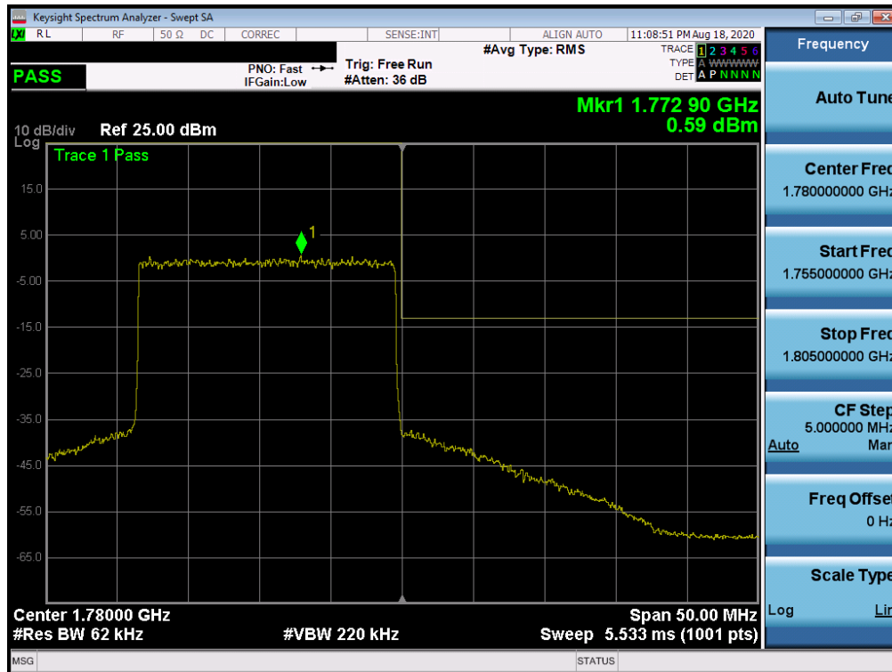
Plot 7-476. Upper Band Edge Plot (NR Band n66 – 20.0MHz - Full RB)
