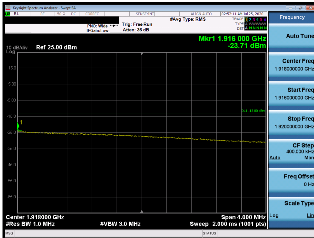
Plot 7-537. Upper Extended Band Edge Plot (NR Band n25 – 20.0MHz - Full RB)
