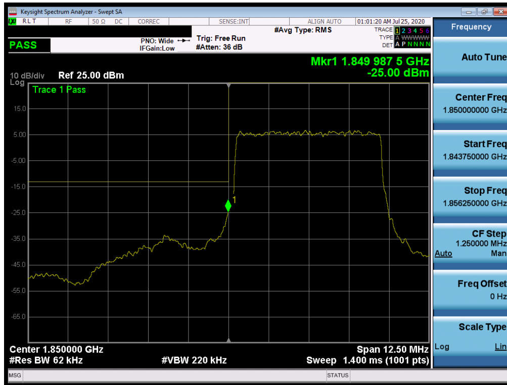
Plot 7-514. Lower Band Edge Plot (NR Band n25/2 – 5.0MHz - Full RB)
