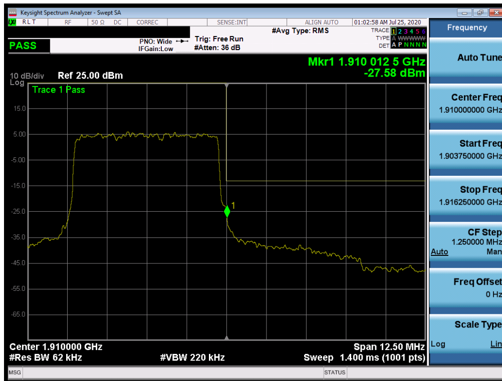
Plot 7-516. Upper Band Edge Plot (NR Band n2 - 5.0MHz - Full RB)
