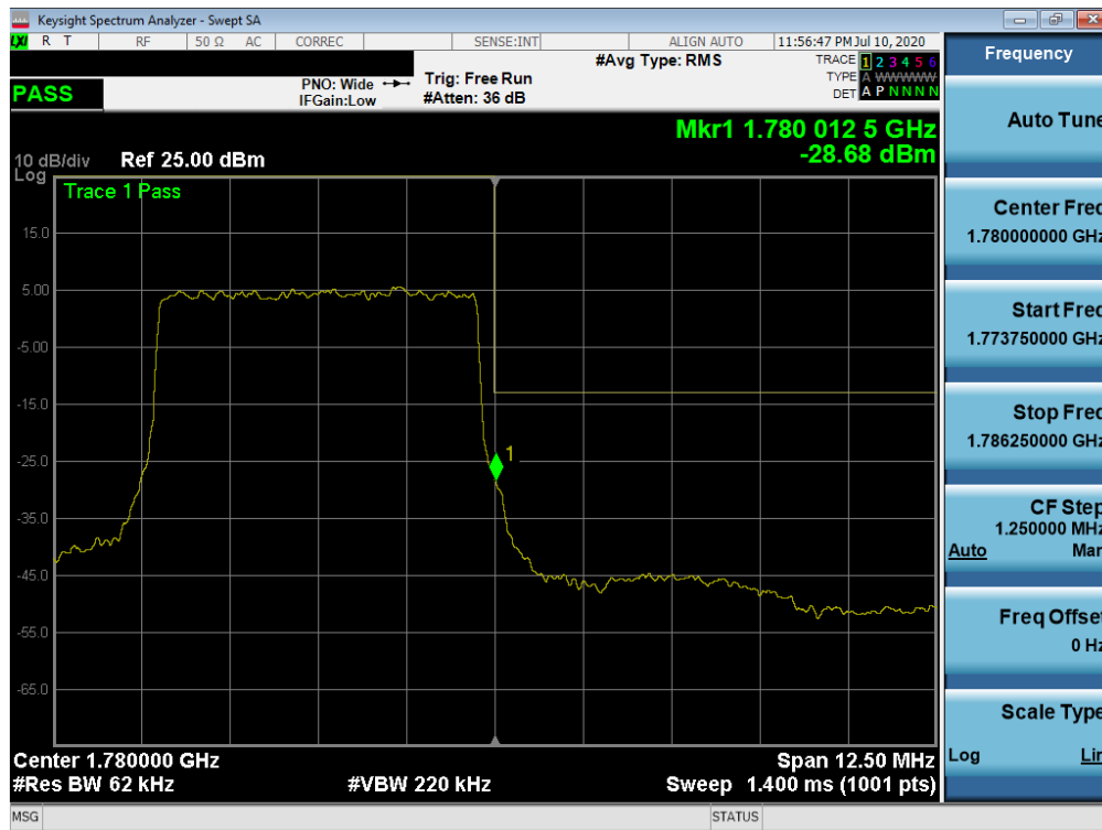
Plot 7-464. Upper Band Edge Plot (NR Band n66 – 5.0MHz - Full RB)
