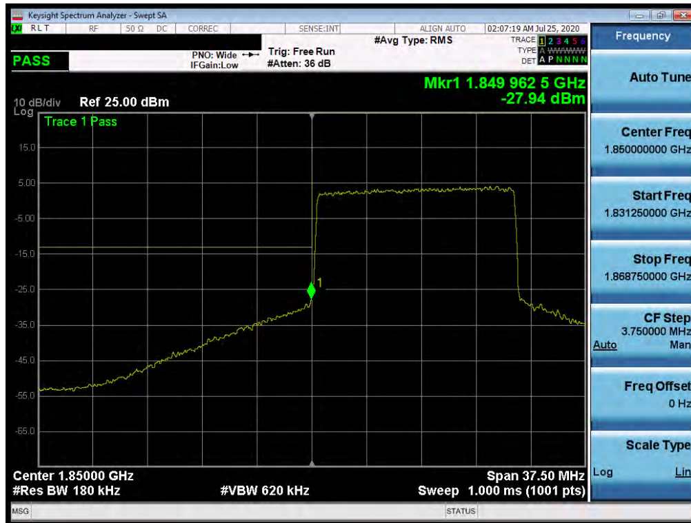
Plot 7-526. Lower Band Edge Plot (NR Band n25/2 – 15.0MHz - Full RB)
