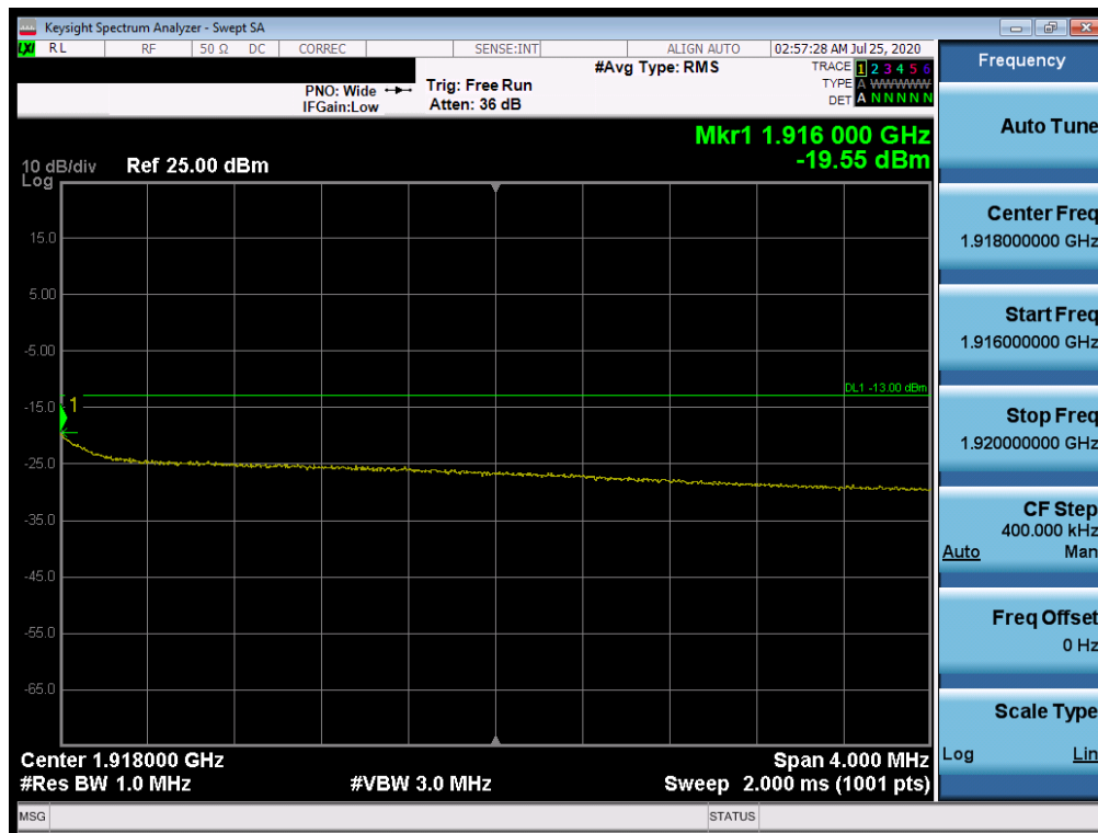
Plot 7-525. Upper Extended Band Edge Plot (NR Band n25 – 10.0MHz - Full RB)
