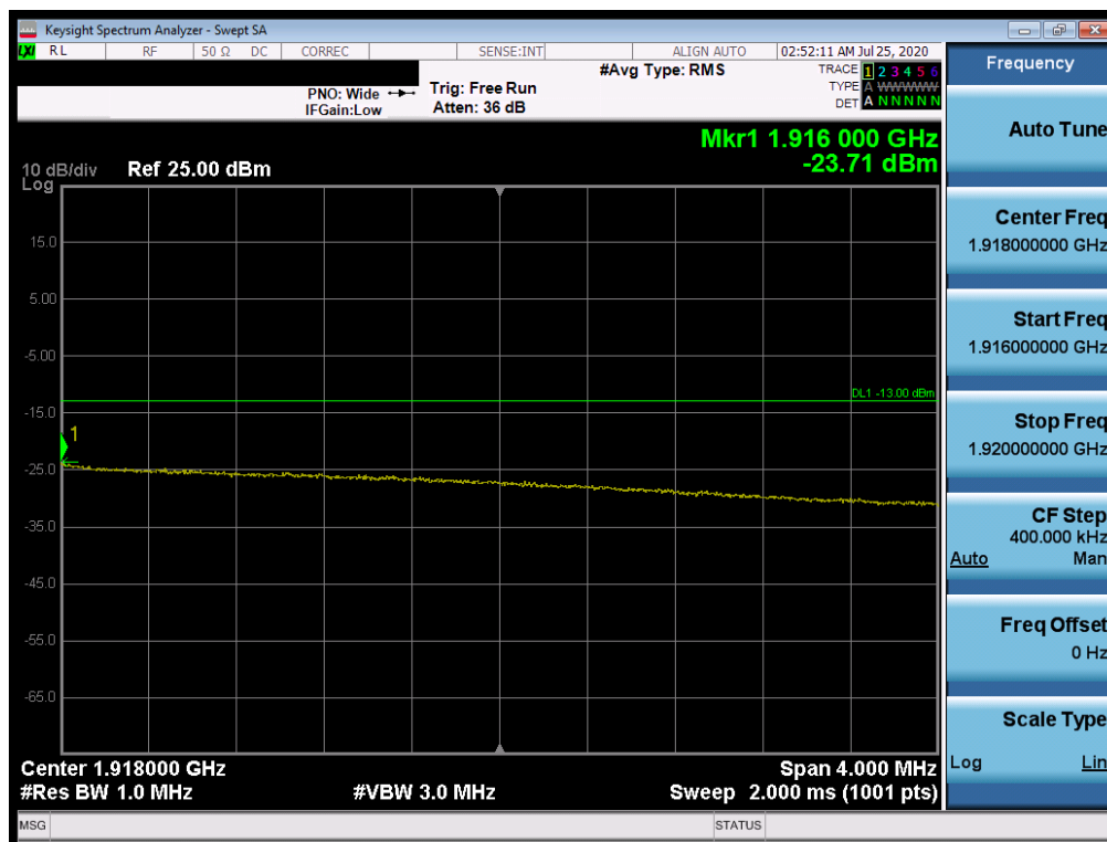
Plot 7-519. Upper Extended Band Edge Plot (NR Band n25 - 5.0MHz - Full RB)
