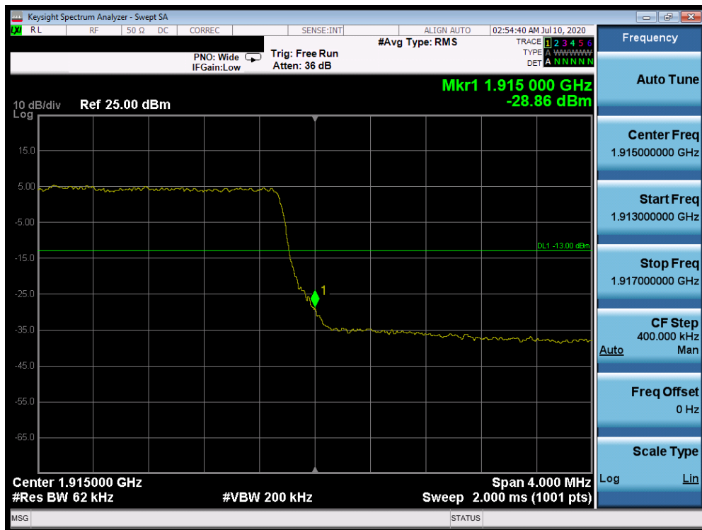
Plot 7-494. Upper Band Edge Plot (Band 25 - 5.0MHz QPSK - Full RB Configuration)
