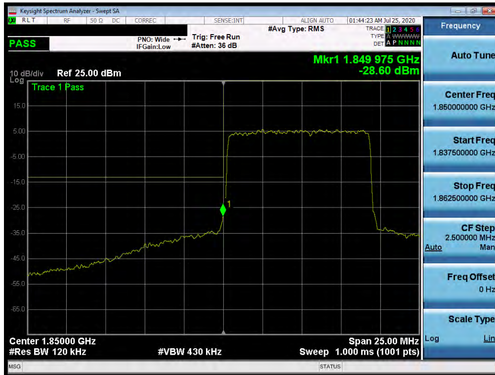
Plot 7-520. Lower Band Edge Plot (NR Band n25/2 – 10.0MHz - Full RB)
