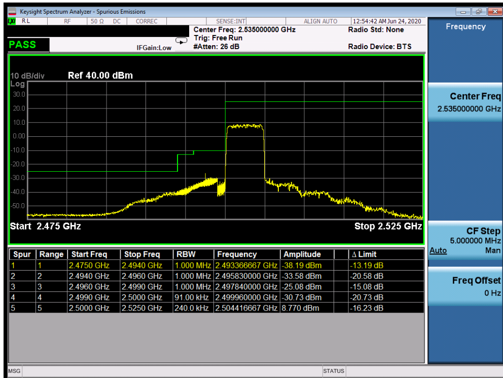
Plot 7-554. Lower Band Edge Plot (Band 7 - 5.0MHz QPSK - Full RB Configuration)
