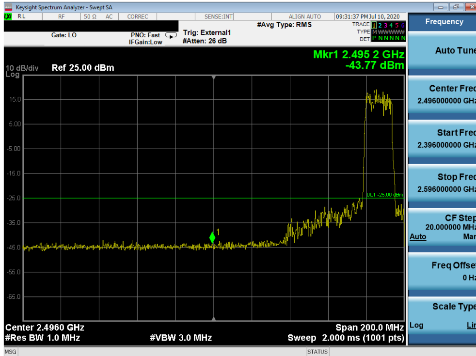
Plot 7-566. Lower Band Edge Plot (Band 38 - 15.0MHz QPSK - Full RB Configuration)
