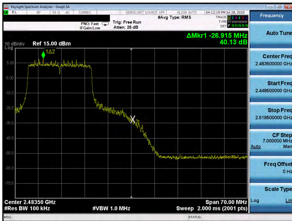
Plot 7-28. Band Edge Plot SISO ANT1 (802.11ax OFDMA - 242 Tones - Ch. 11)
