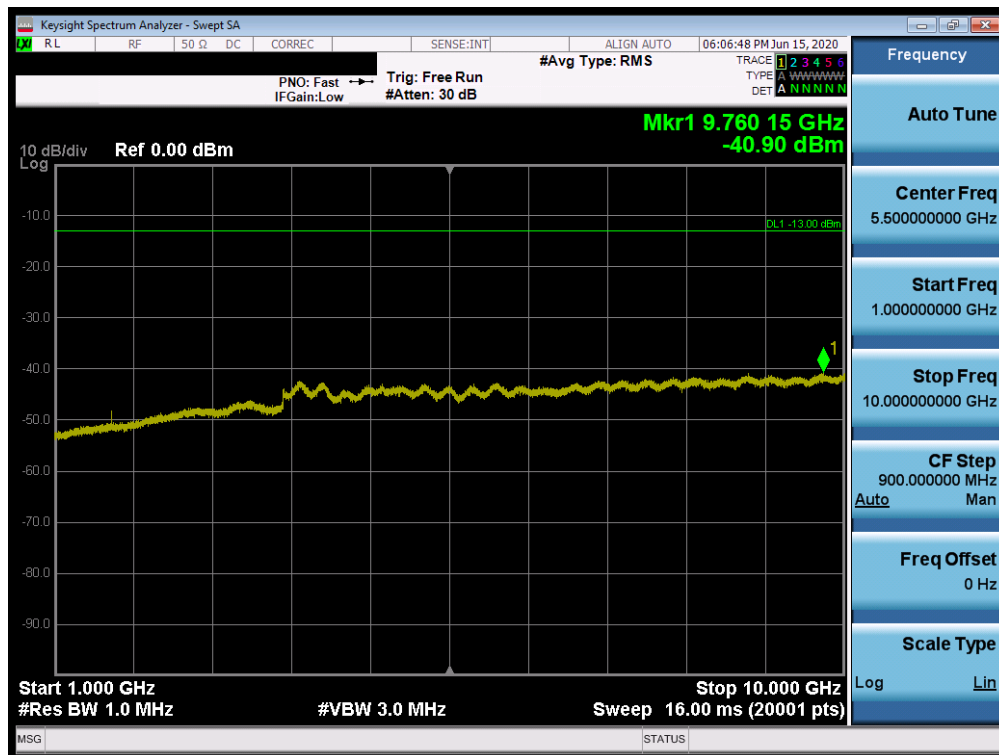
Plot 7-36. Conducted Spurious Plot (CDMA/EvDO, Ch. 684)
