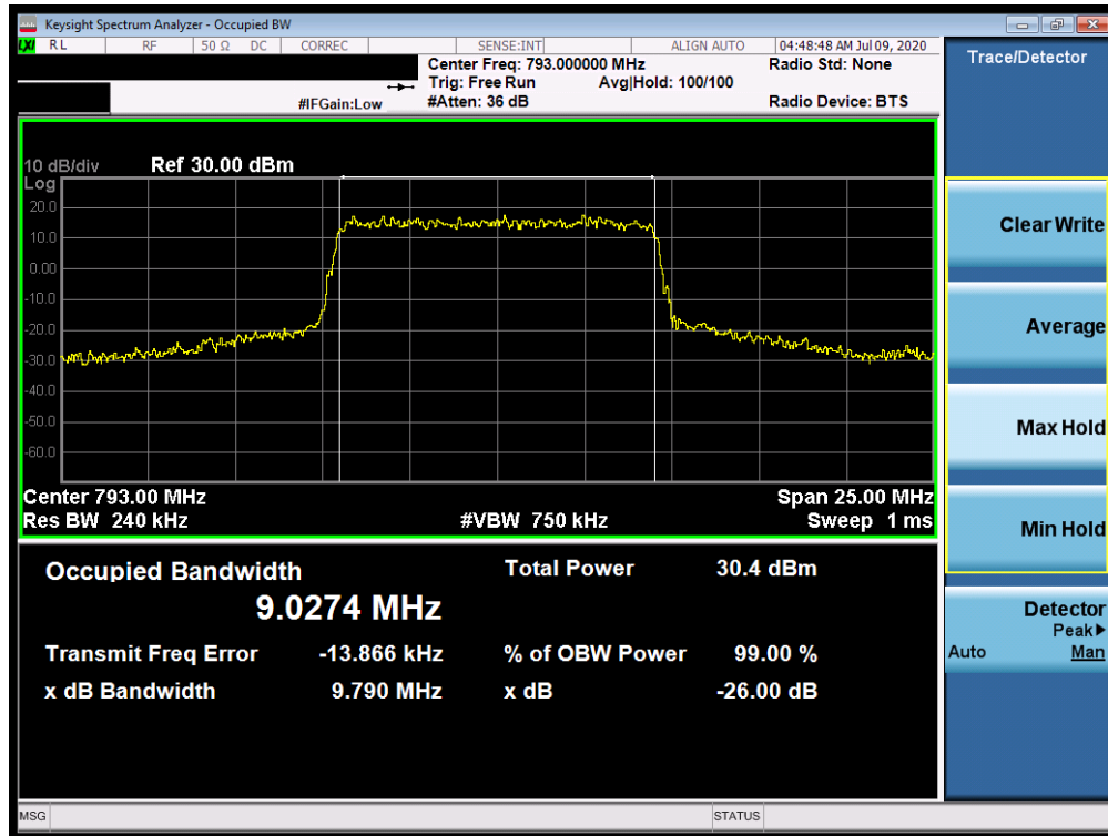
Plot 7-23. Occupied Bandwidth Plot (LTE Band 14 - 10MHz QPSK - Full RB Configuration)
