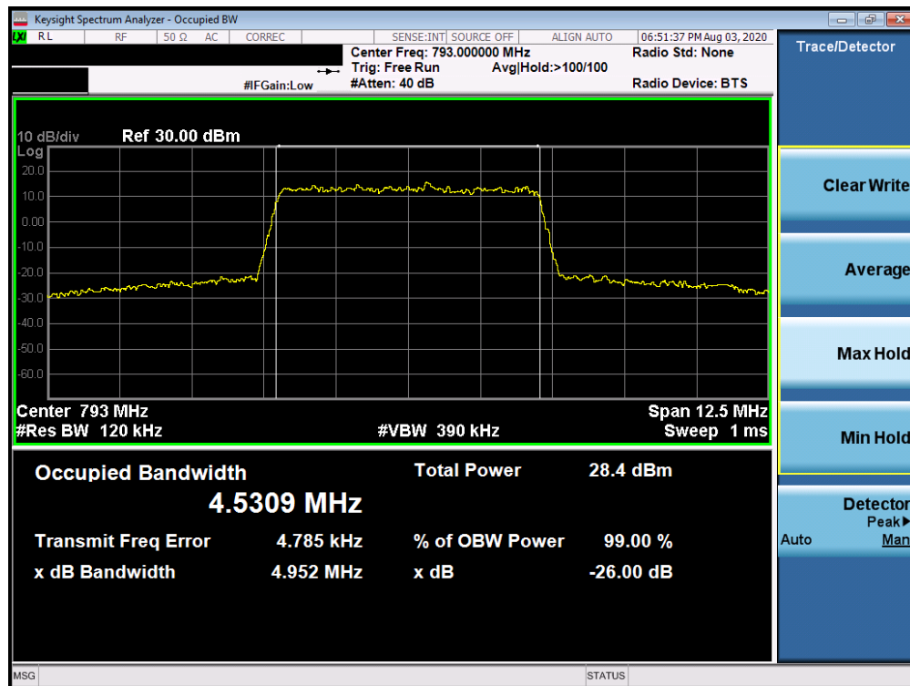
Plot 7-30. Occupied Bandwidth Plot (LTE Band 14 - 5MHz 256-QAM - Full RB Configuration)
