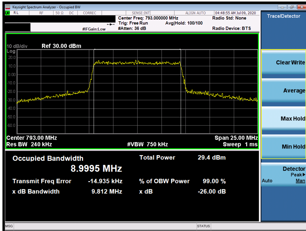
Plot 7-24. Occupied Bandwidth Plot (LTE Band 14 - 10MHz 16-QAM - Full RB Configuration)
