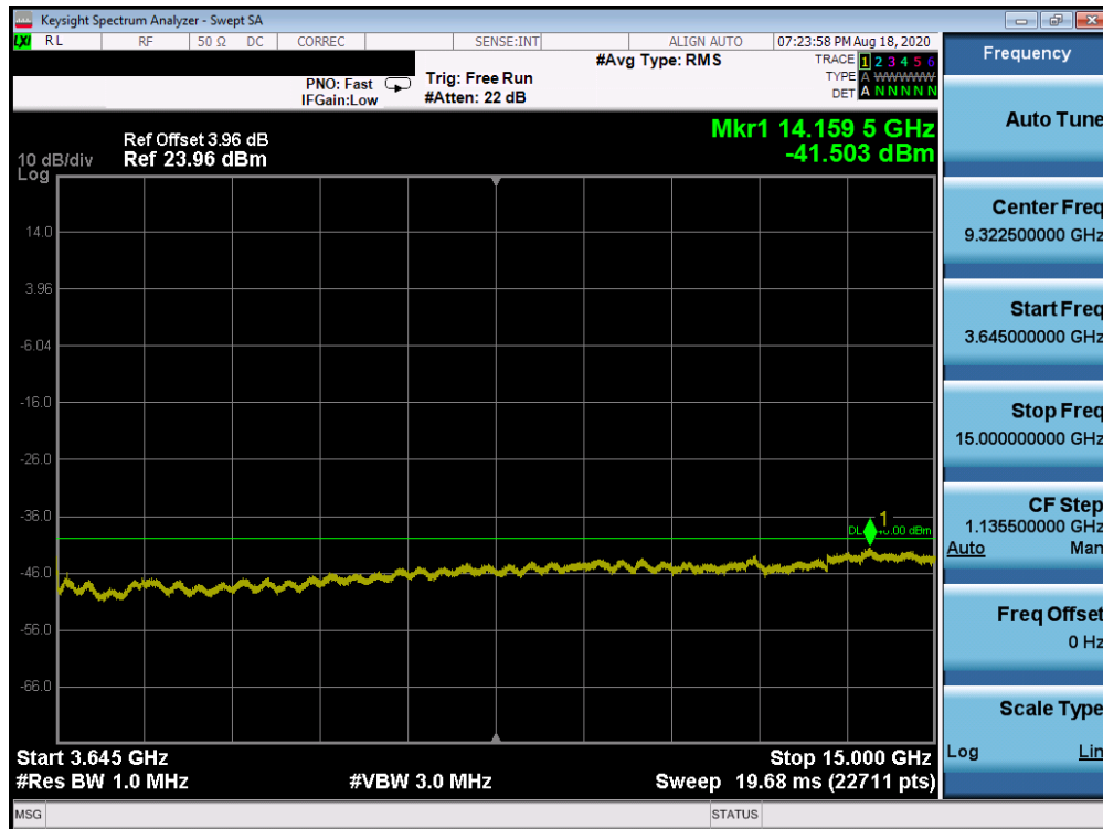
Plot 7-37. Conducted Spurious Plot (LTE Band 48 - 20.0MHz QPSK - RB Size 1, RB Offset 0 - Mid Channel)
