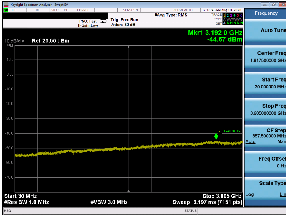
Plot 7-33. Conducted Spurious Plot (LTE Band 48 - 20.0MHz QPSK - RB Size 1, RB Offset 0 - Low Channel)
