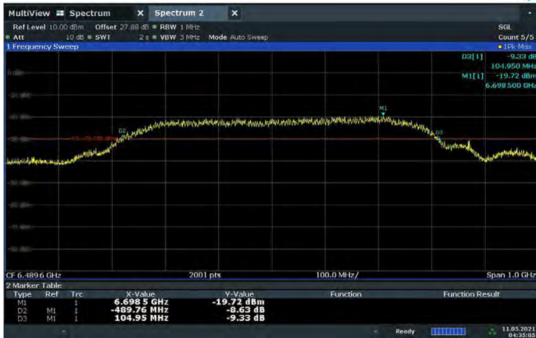
Plot 7-6. BANDWIDTH Plot – CH.5 – SP3 – Preamble 11
