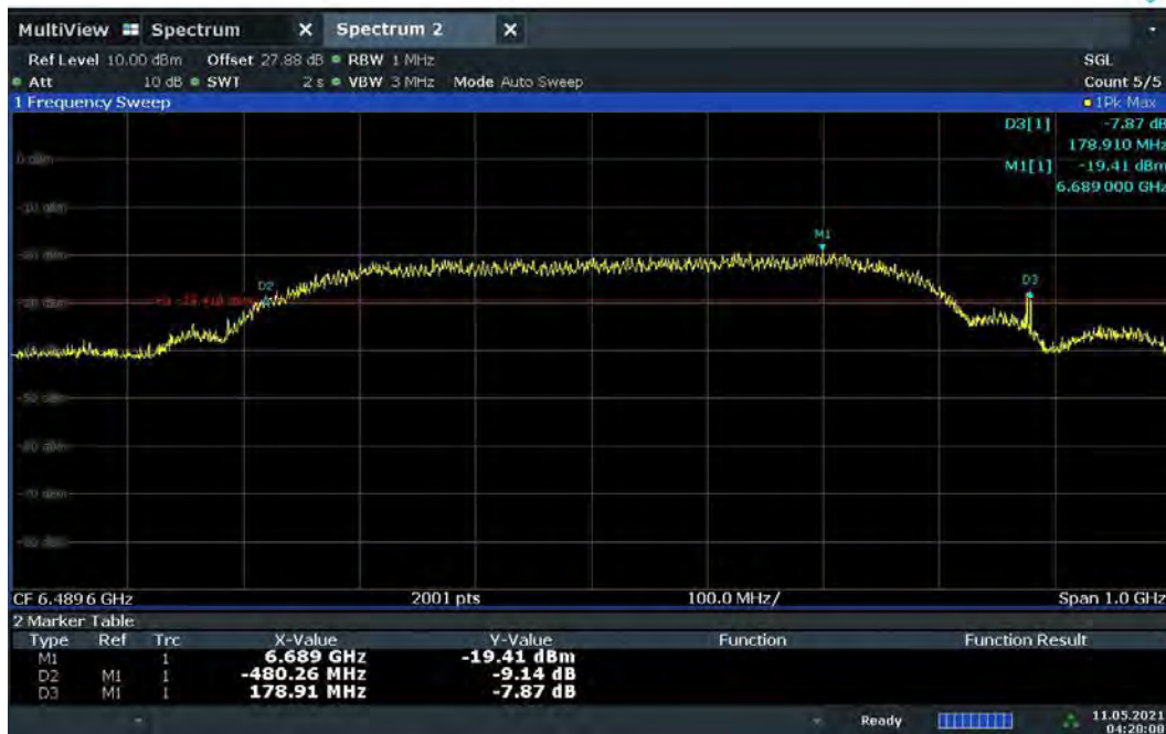
Plot 7-6. BANDWIDTH Plot – CH.5 – SP3 – Preamble 10
