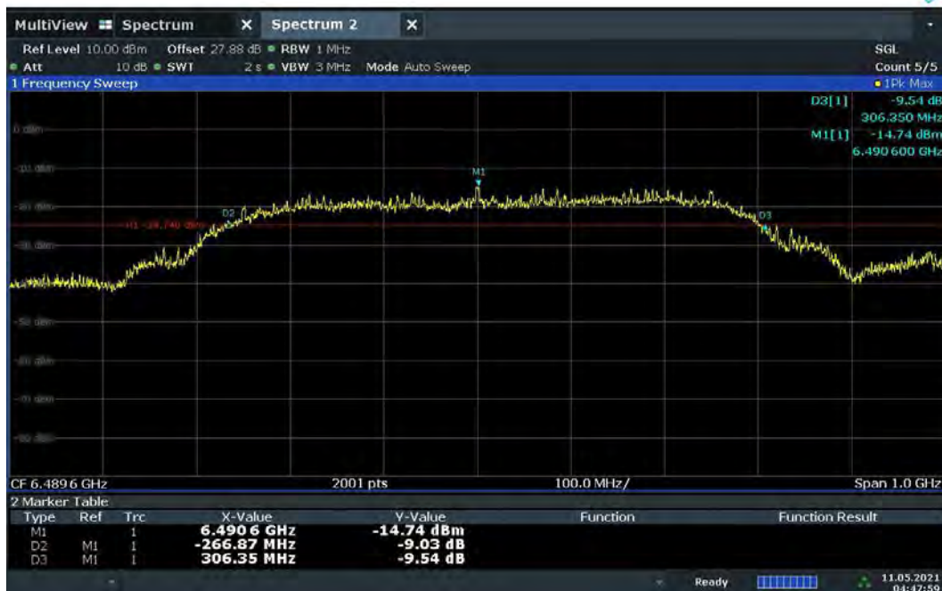
Plot 7-14. BANDWIDTH Plot – CH.5 – SP1 – Preamble 27
