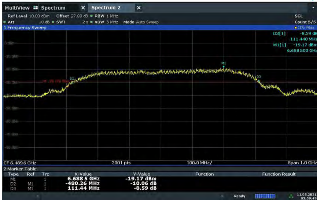
Plot 7-3. BANDWIDTH Plot – CH.5 – SP3 – Preamble 9
