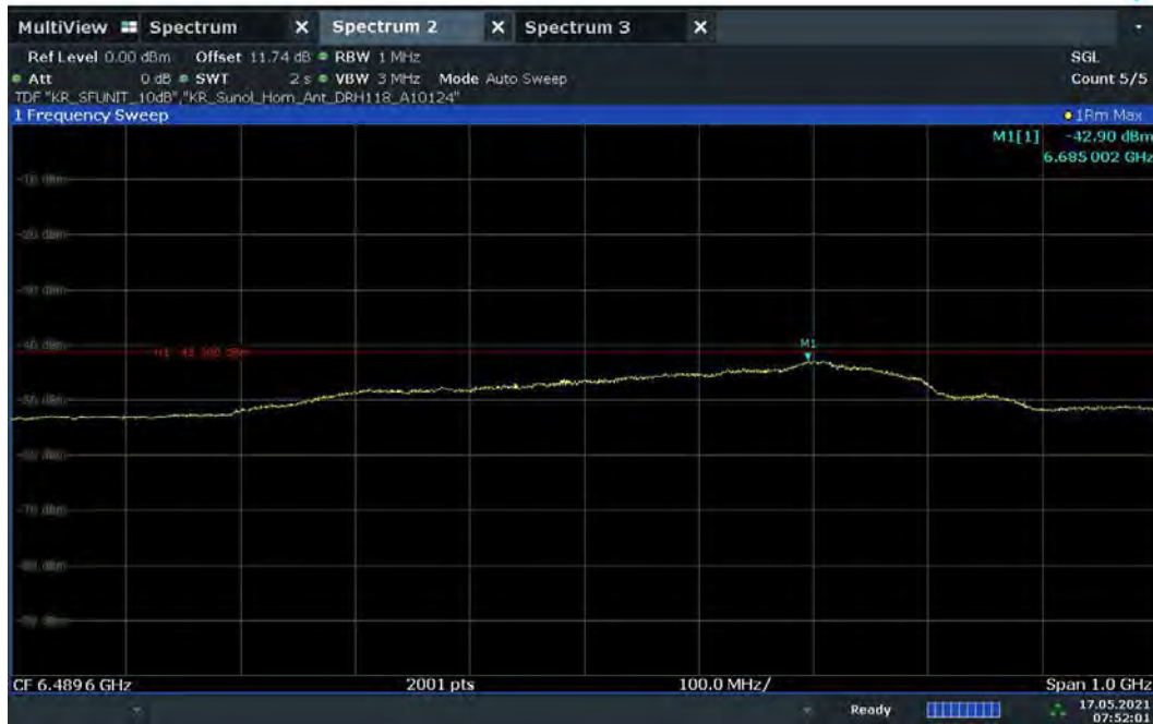
Plot 7-66. UWB Average Power Measurement - ANT 1 - CH.5 – BPRF
