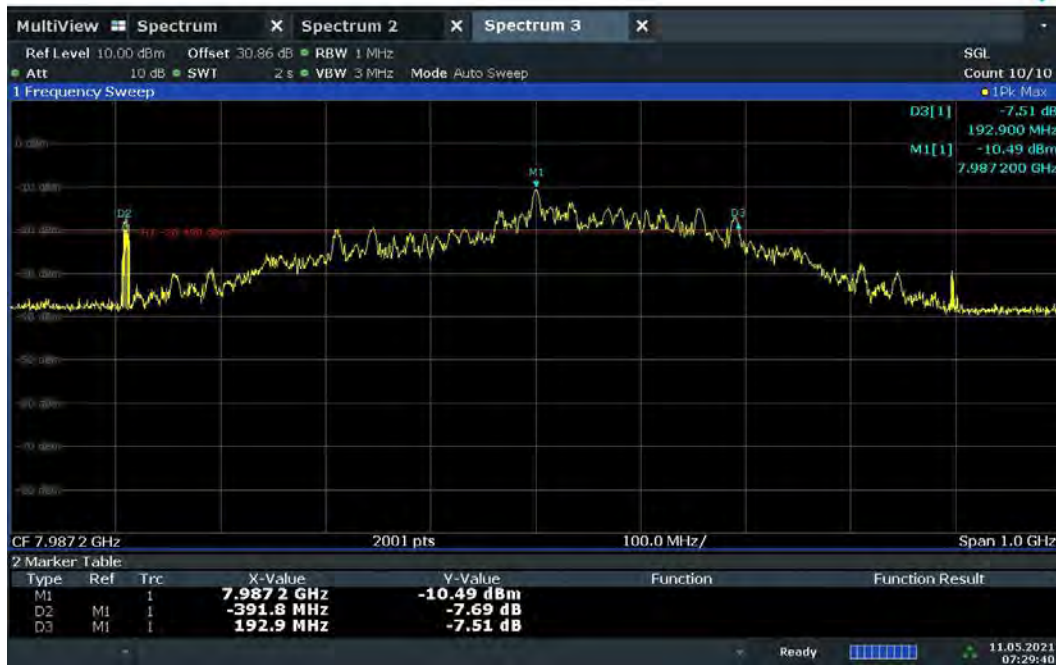
Plot 7-49. BANDWIDTH Plot – CH.9 - SP0 – Preamble 10
