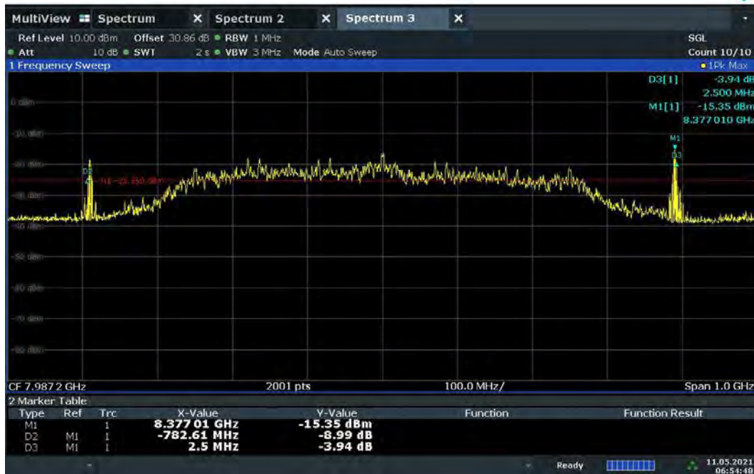
Plot 7-28. BANDWIDTH Plot – CH.9 - SP0 – Preamble 27
