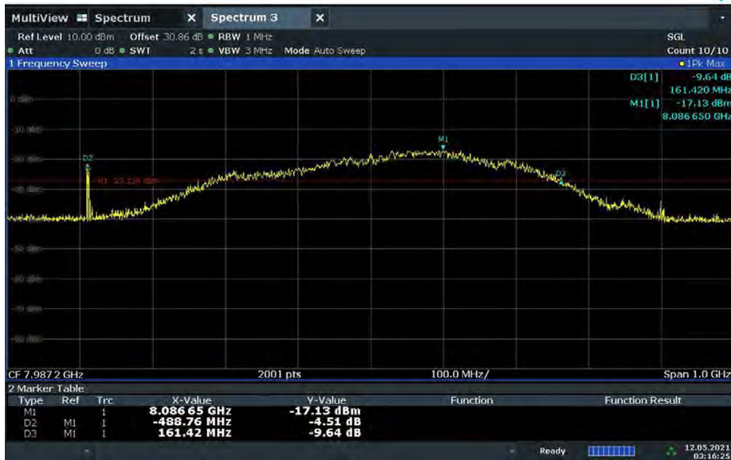
Plot 7-53. BANDWIDTH Plot – CH.9 – SP1 – Preamble 11
