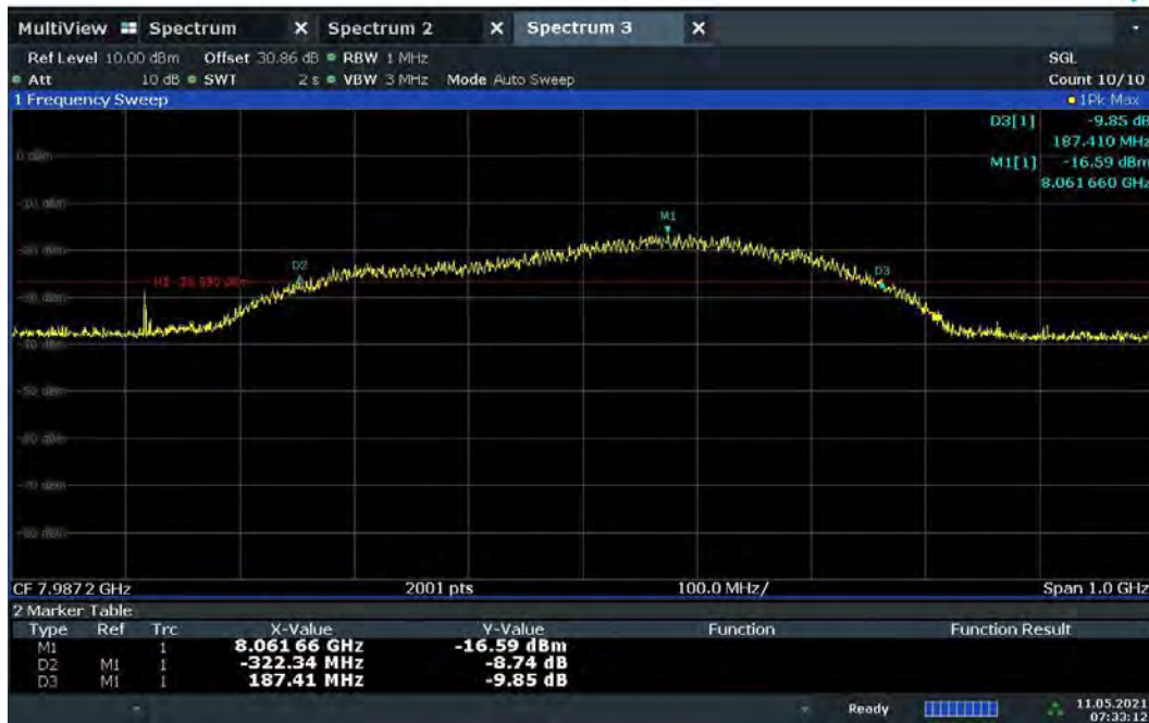
Plot 7-51. BANDWIDTH Plot – CH.9 – SP3 – Preamble 10
