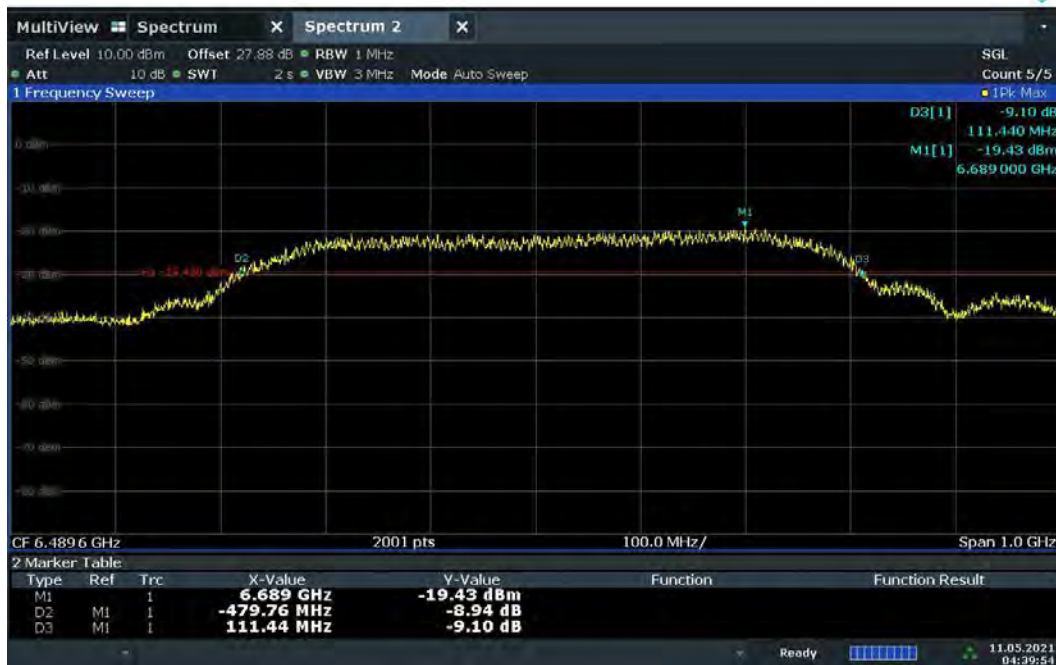
Plot 7-12. BANDWIDTH Plot – CH.5 – SP3 – Preamble 12
