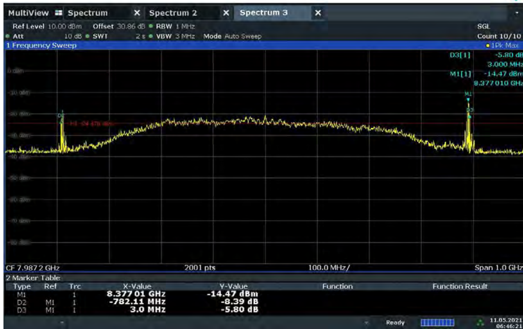
Plot 7-23. BANDWIDTH Plot – CH.9 – SP1 – Preamble 11
