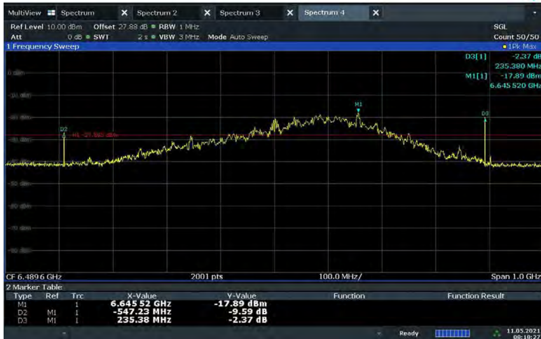
Plot 7-31. BANDWIDTH Plot – CH.5 - SP0 – Preamble 9
