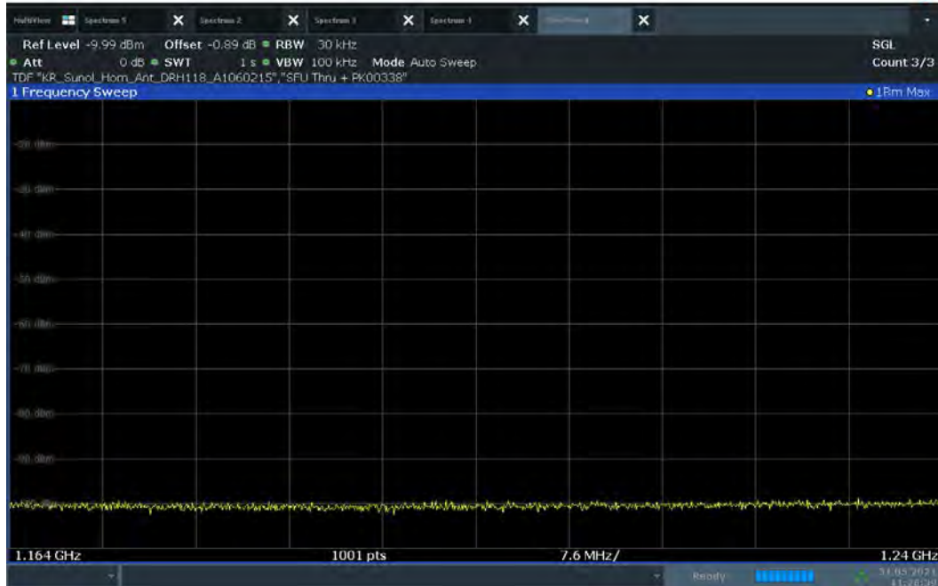
Plot 7-90. Radiated Spurious Pre-Scan 1164 - 1240 MHz - CH.9 - ANT 1 – GPS band
