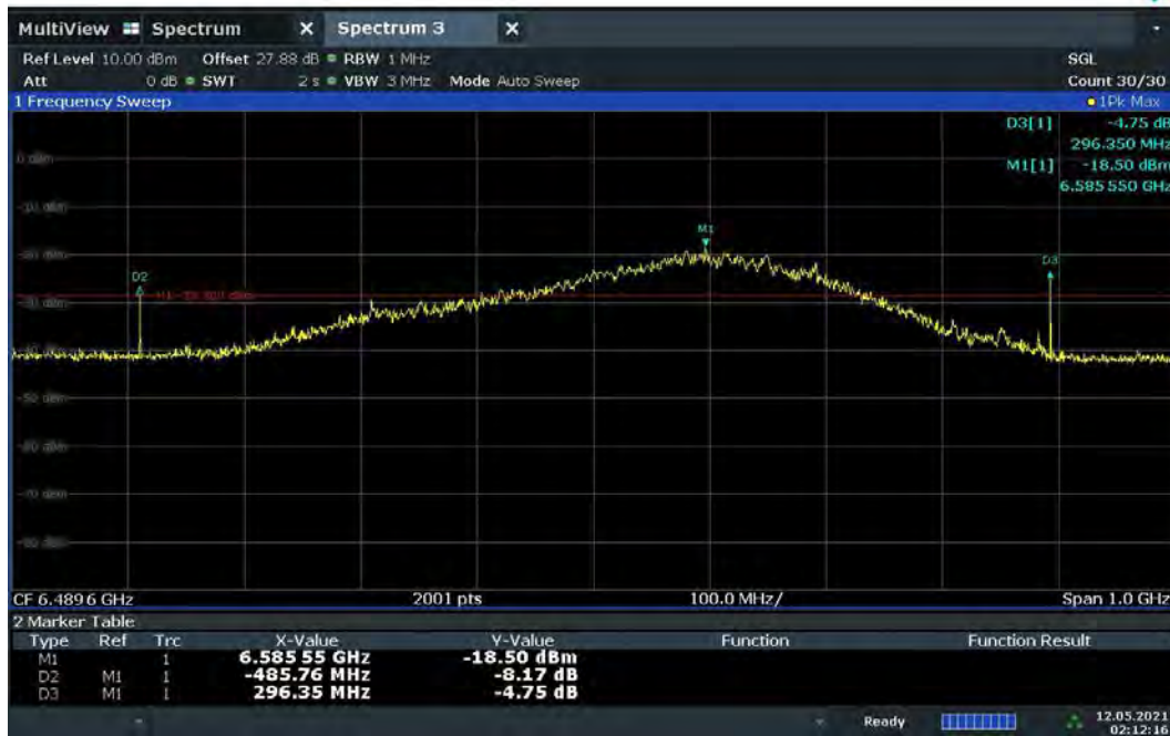
Plot 7-41. BANDWIDTH Plot – CH.5 – SP1 – Preamble 12
