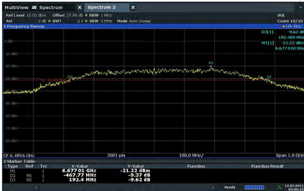
Plot 7-74. BANDWIDTH Plot – CH.5 - SP0 – Preamble 11
