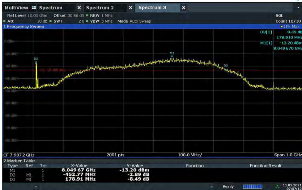
Plot 7-60. BANDWIDTH Plot – CH.9 – SP3 – Preamble 27
