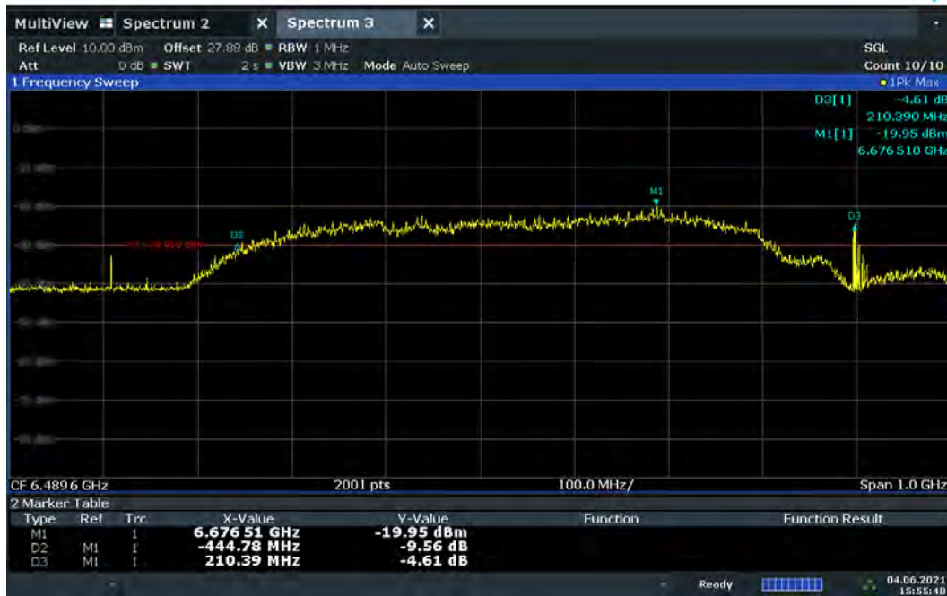
Plot 7-45. BANDWIDTH Plot – CH.5 – SP3 – Preamble 27
