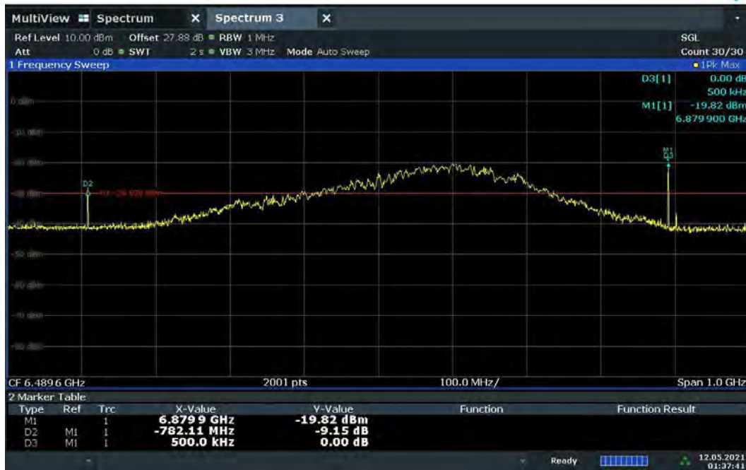
Plot 7-37. BANDWIDTH Plot – CH.5 - SP0 – Preamble 11
