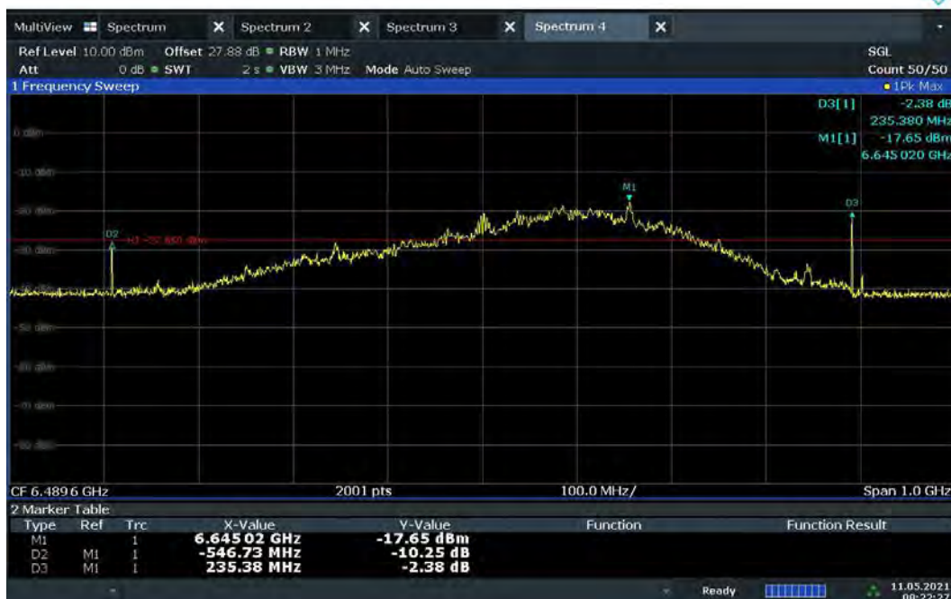
Plot 7-32. BANDWIDTH Plot – CH.5 – SP1 – Preamble 9
