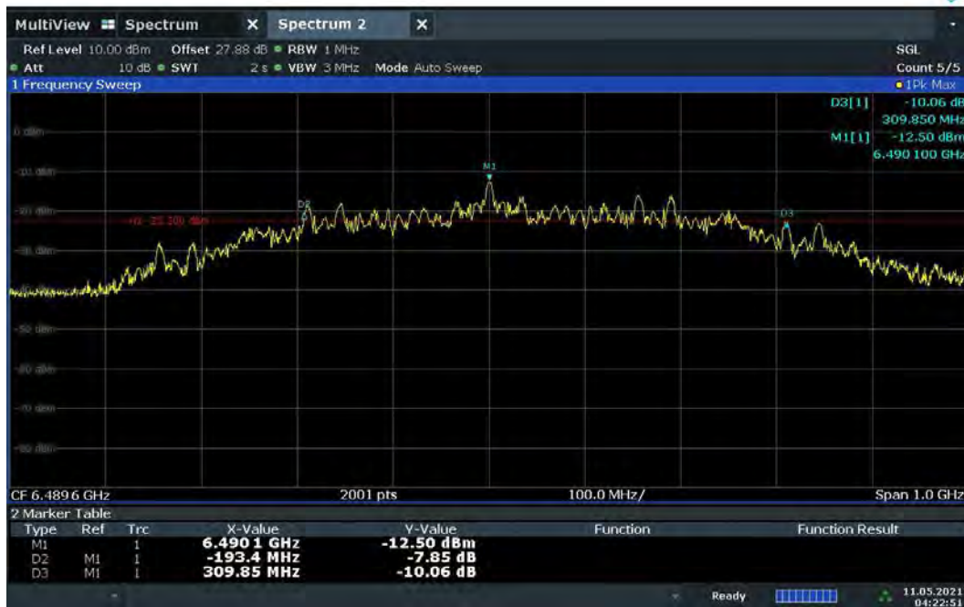
Plot 7-4. BANDWIDTH Plot – CH.5 - SP0 – Preamble 10
