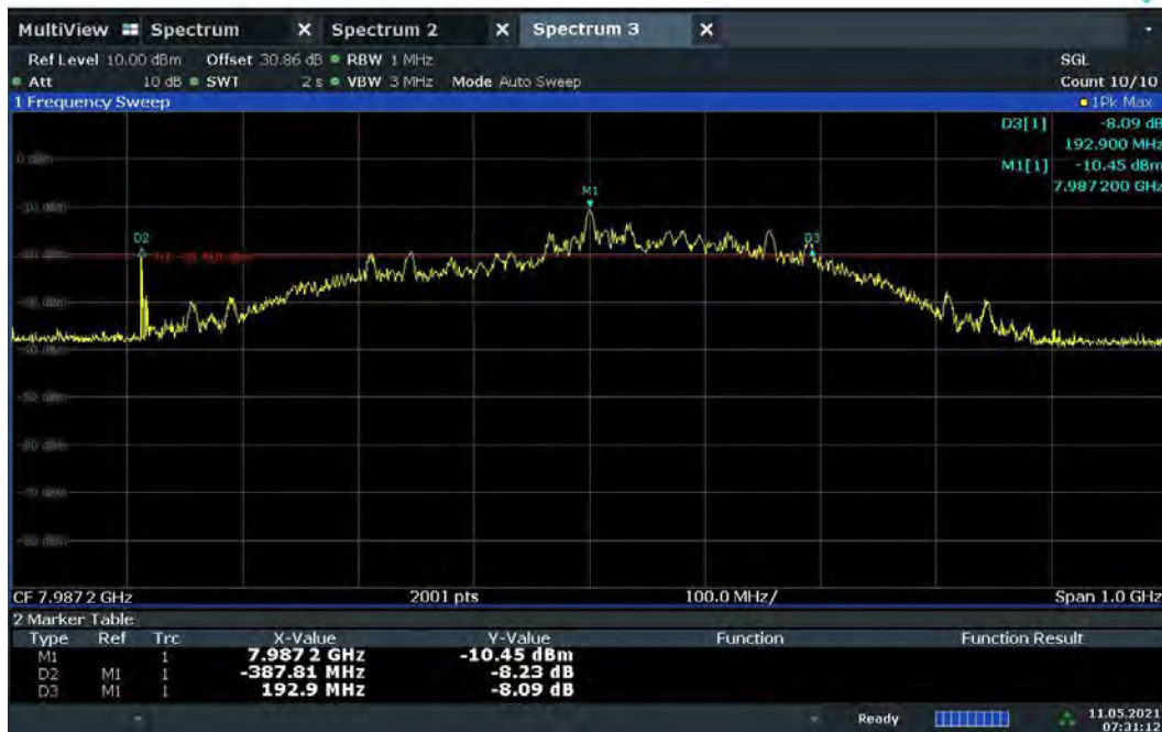
Plot 7-50. BANDWIDTH Plot – CH.9 – SP1 – Preamble 10
