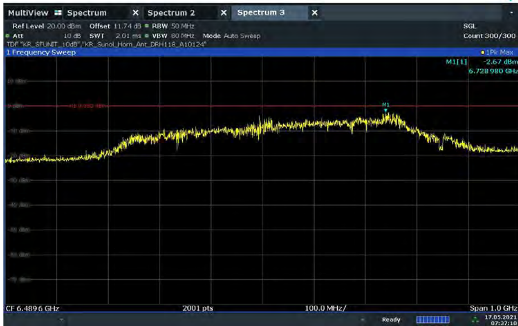
Plot 7-62. UWB Peak Power Measurement - ANT 1 - CH.5 – BPRF
