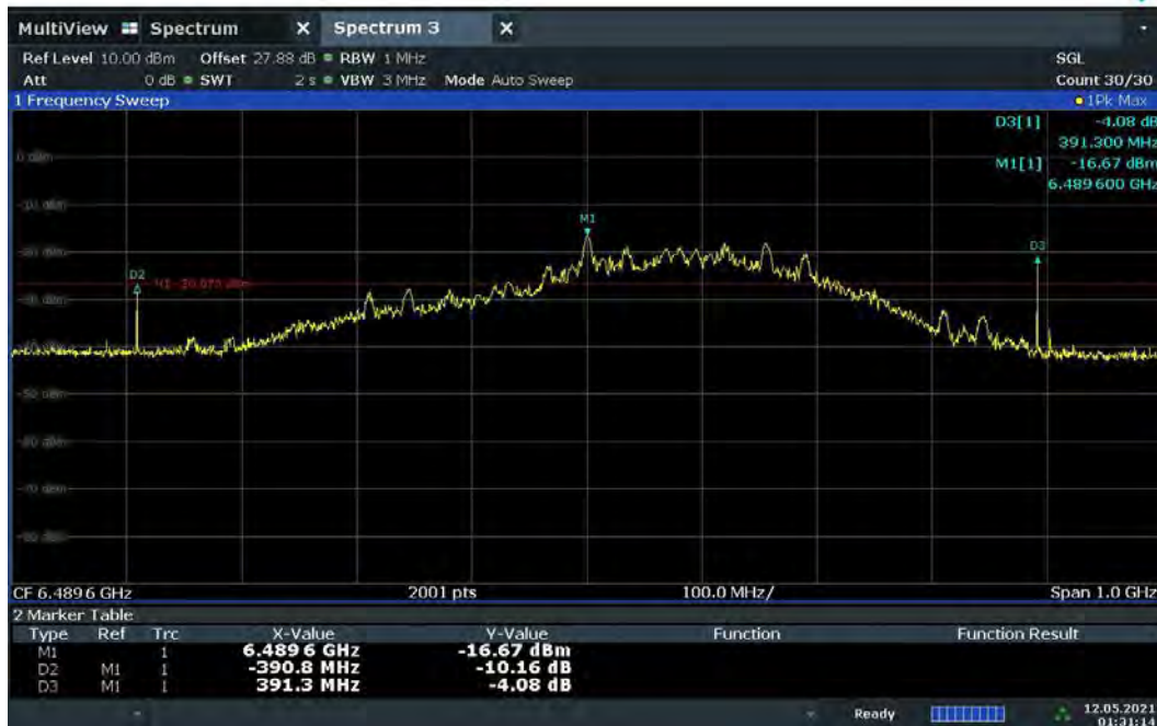
Plot 7-35. BANDWIDTH Plot – CH.5 – SP1 – Preamble 10
