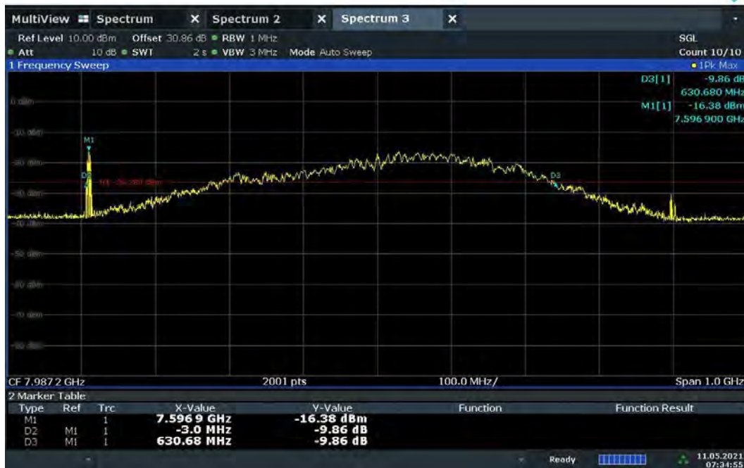
Plot 7-52. BANDWIDTH Plot – CH.9 - SP0 – Preamble 11
