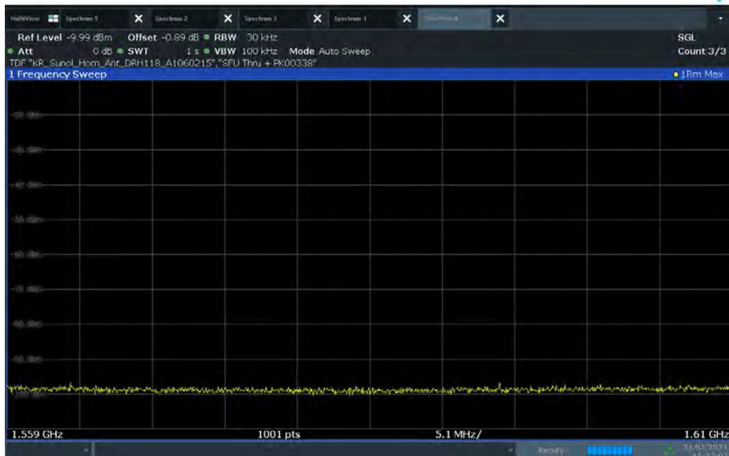
Plot 7-91. Radiated Spurious Pre-Scan 1559 - 1610 MHz - CH.9 - ANT 1 – GPS band
