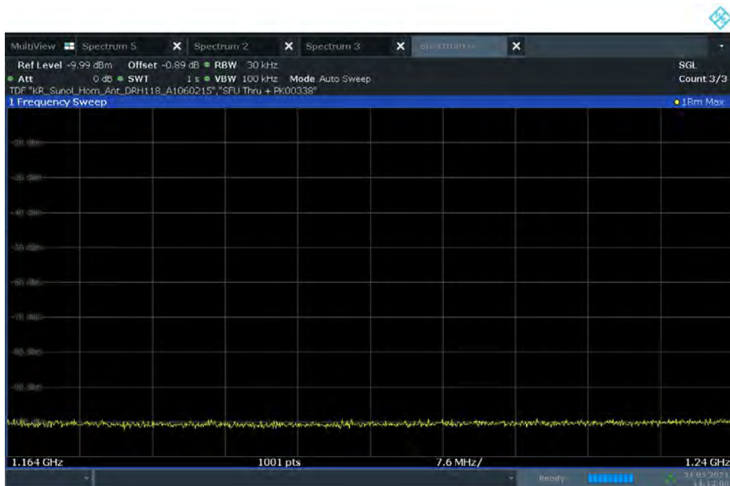
Plot 7-80. Radiated Spurious Pre-Scan 1164 - 1240 MHz - CH.5 - ANT 1 – GPS band
