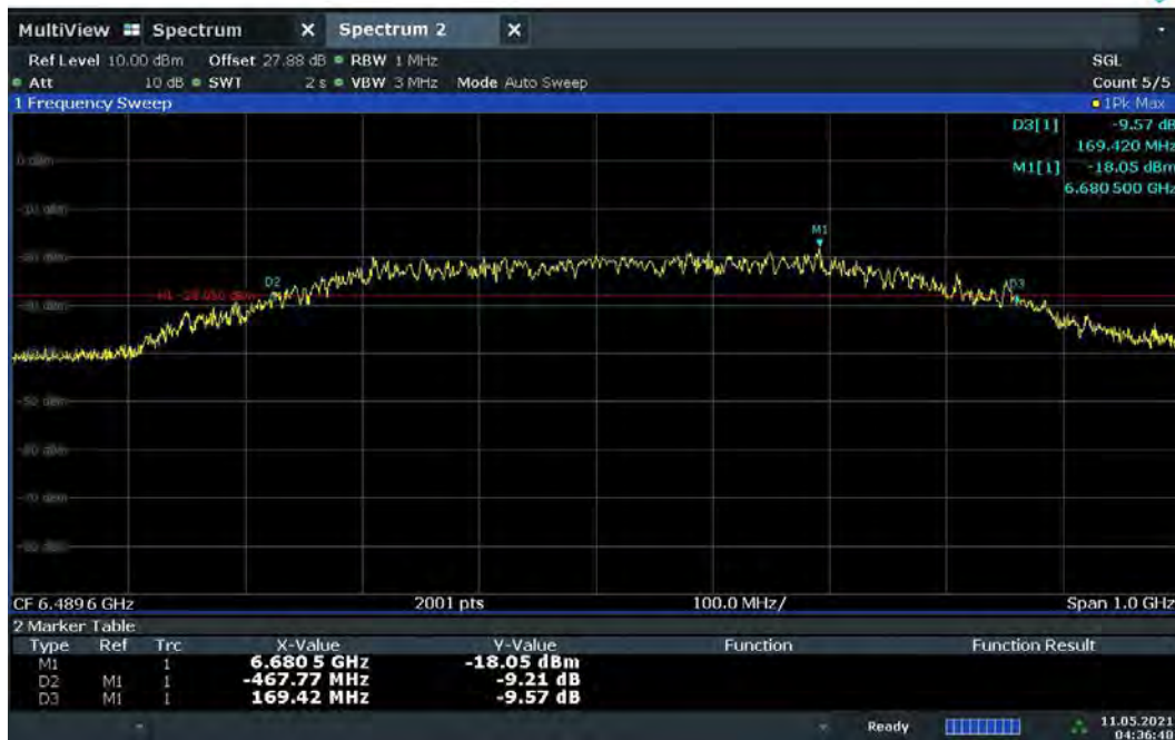
Plot 7-10. BANDWIDTH Plot – CH.5 - SP0 – Preamble 12
