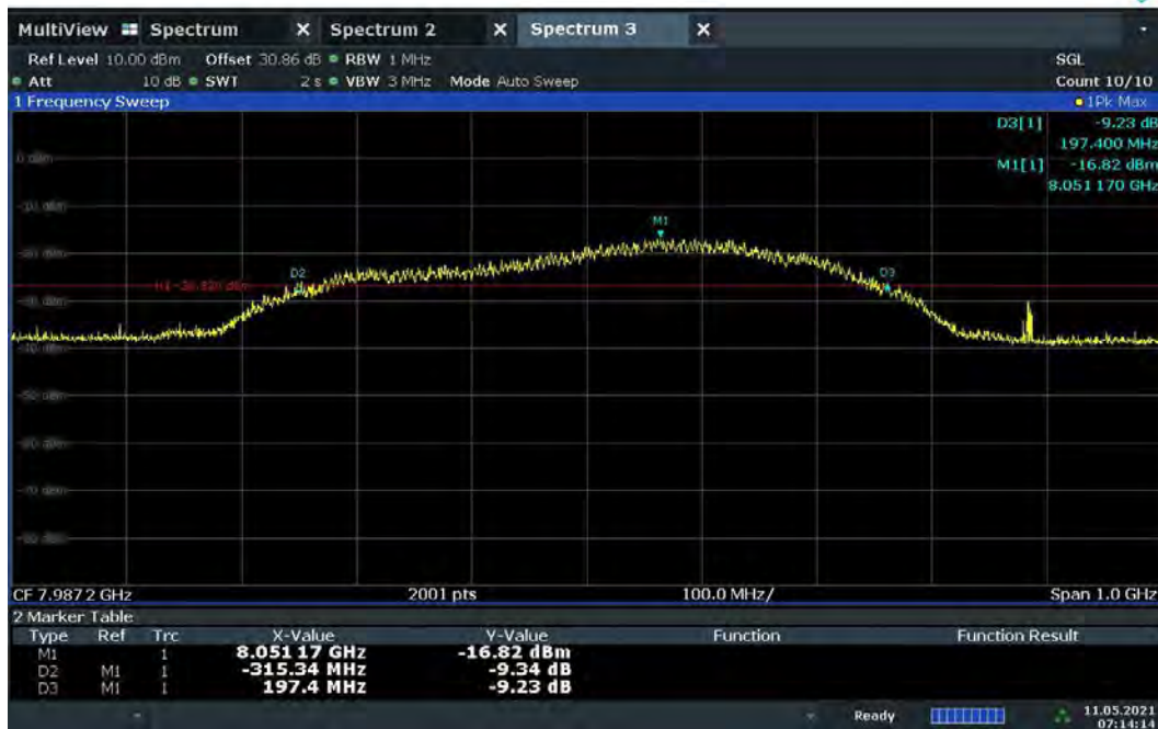
Plot 7-48. BANDWIDTH Plot – CH.9 – SP3 – Preamble 9
