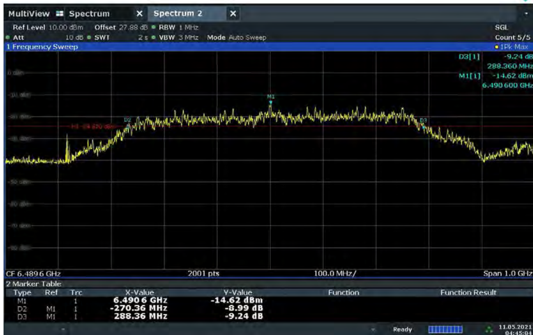
Plot 7-13. BANDWIDTH Plot – CH.5 - SP0 – Preamble 27
