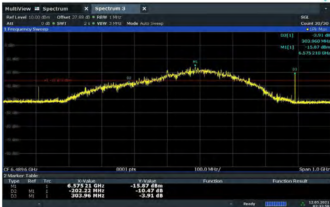
Plot 7-44. BANDWIDTH Plot – CH.5 – SP1 – Preamble 27
