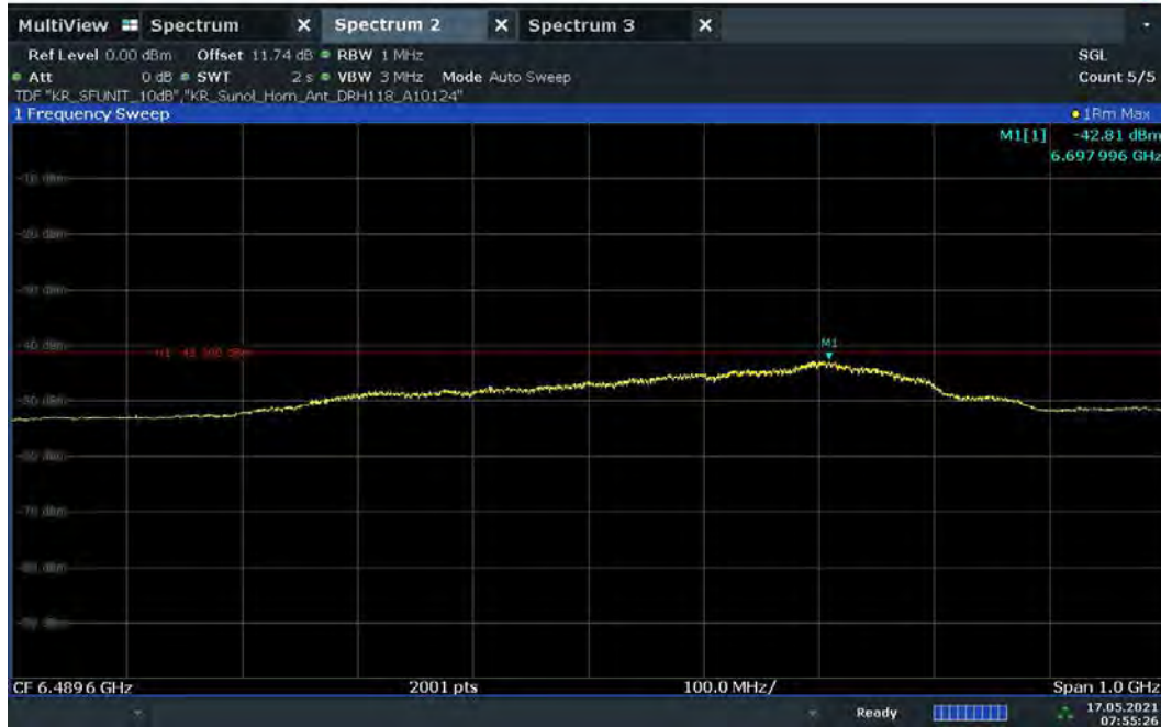
Plot 7-74. UWB Average Power Measurement - ANT 1 - CH.5 – HPRF
