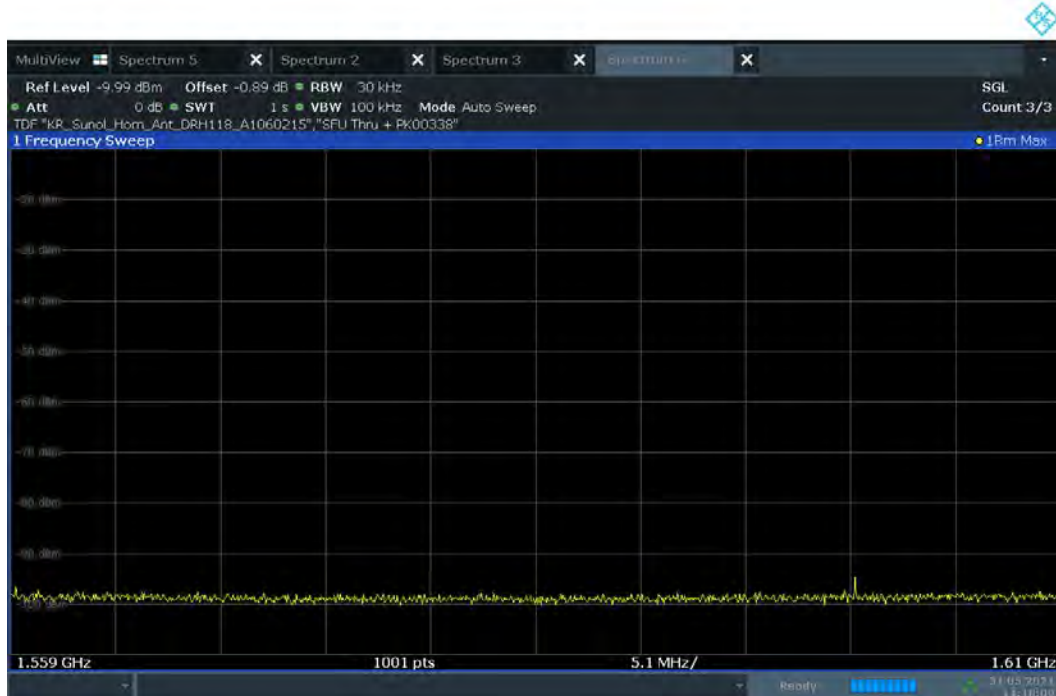
Plot 7-81. Radiated Spurious Pre-Scan 1559 - 1610 MHz - CH.5 - ANT 1 – GPS band
