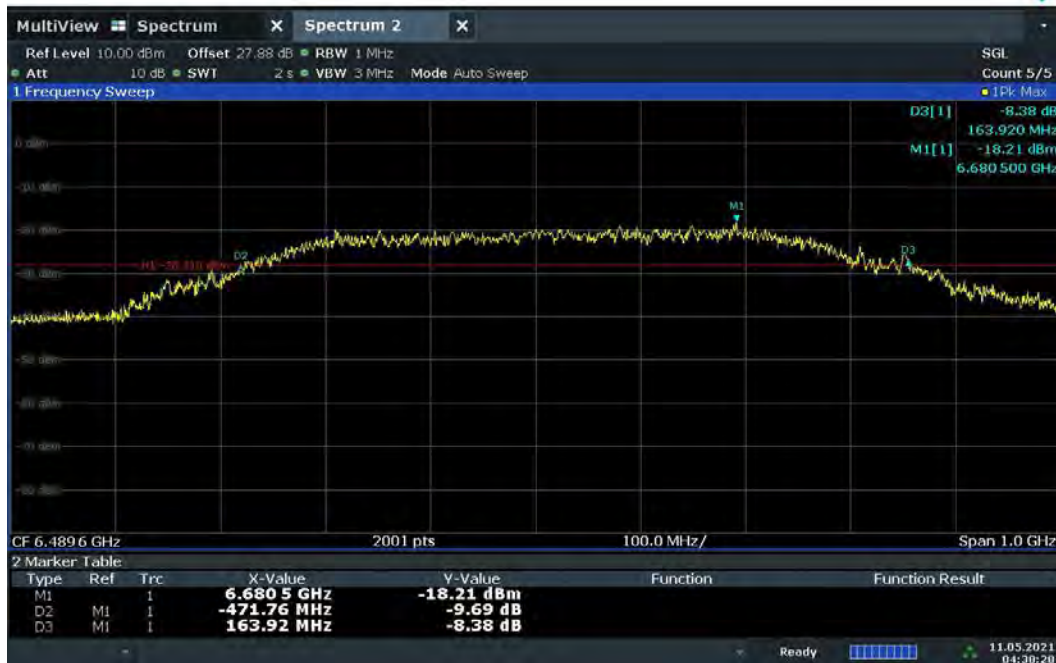
Plot 7-11. BANDWIDTH Plot – CH.5 – SP1 – Preamble 12
