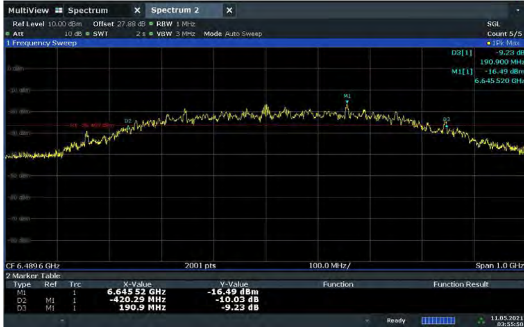
Plot 7-1. BANDWIDTH Plot – CH.5 - SP0 – Preamble 9
