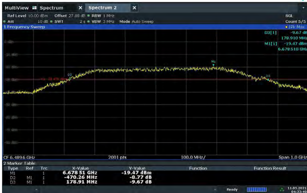
Plot 7-5. BANDWIDTH Plot – CH.5 – SP1 – Preamble 11
