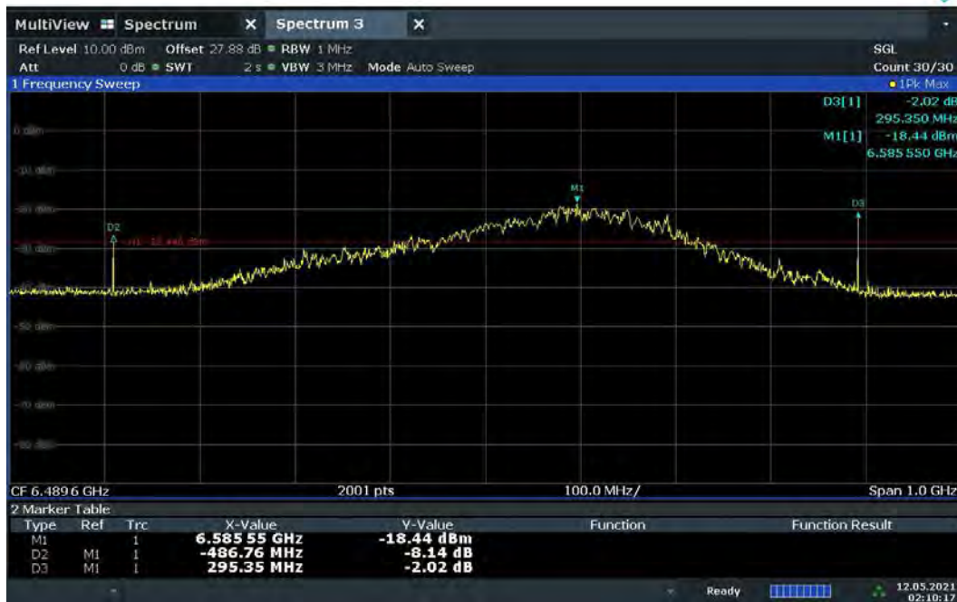
Plot 7-40. BANDWIDTH Plot – CH.5 - SP0 – Preamble 12
