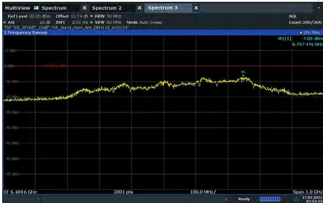
Plot 7-70. UWB Peak Power Measurement - ANT 1 - CH.5 – HPRF
