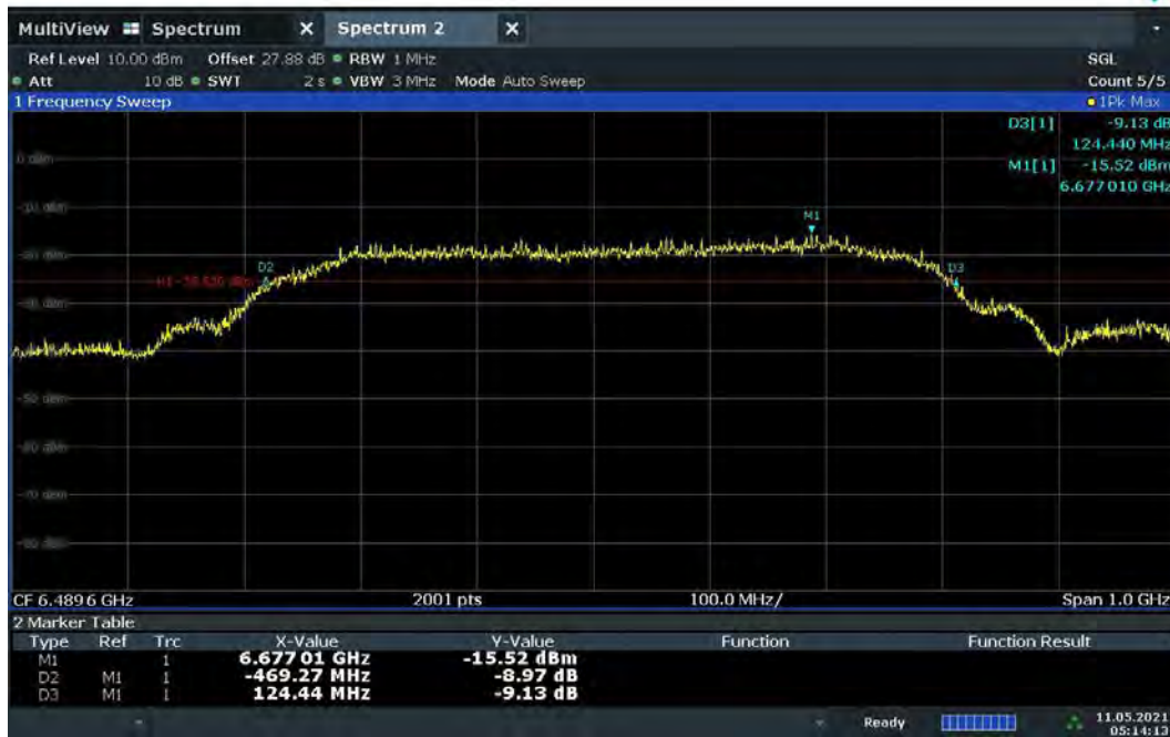
Plot 7-15. BANDWIDTH Plot – CH.5 – SP3 – Preamble 27
