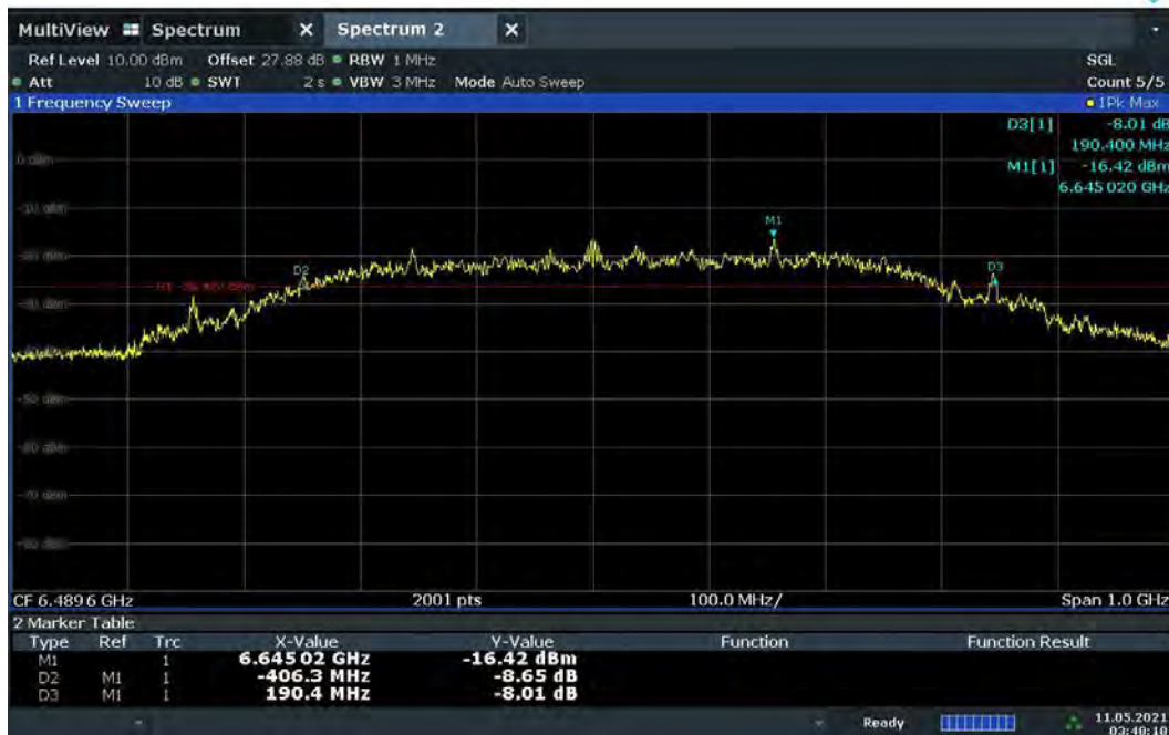
Plot 7-2. BANDWIDTH Plot – CH.5 – SP1 – Preamble 9
