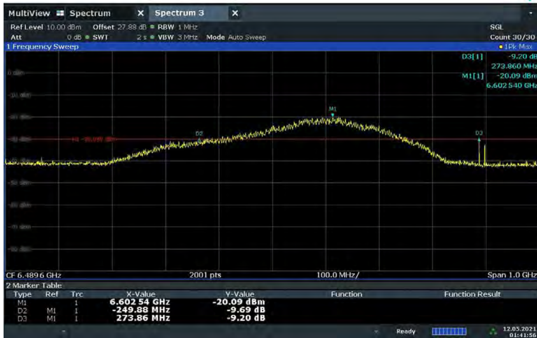
Plot 7-39. BANDWIDTH Plot – CH.5 – SP3 – Preamble 11
