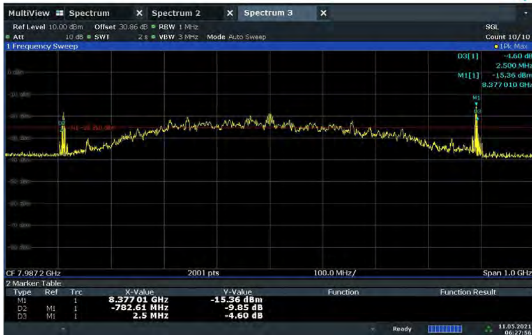
Plot 7-16. BANDWIDTH Plot – CH.9 - SP0 – Preamble 9
