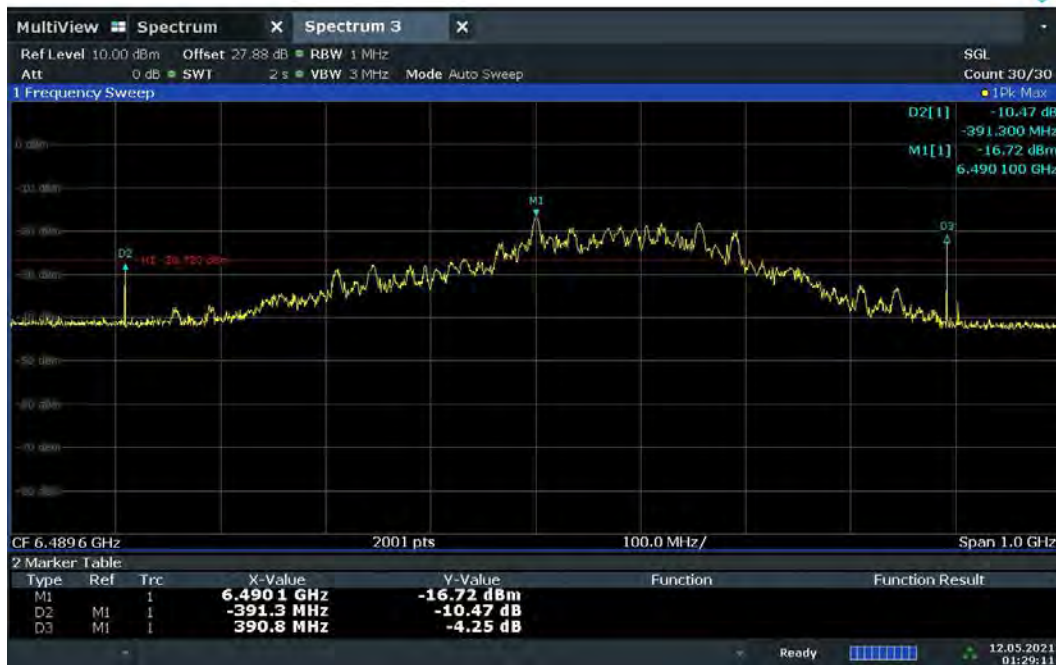
Plot 7-34. BANDWIDTH Plot – CH.5 - SP0 – Preamble 10
