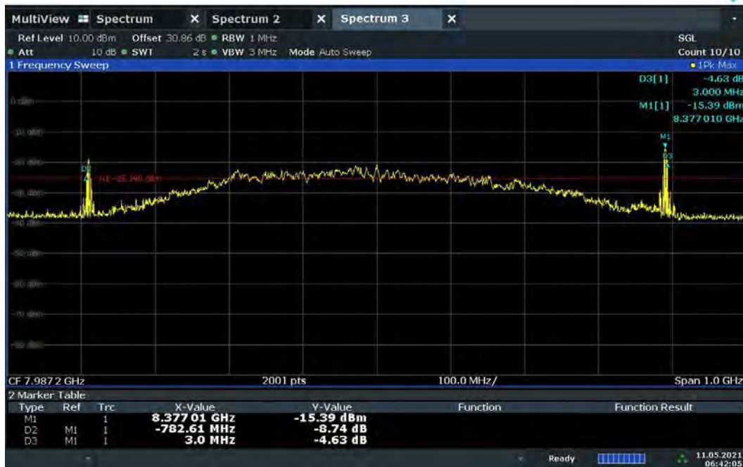
Plot 7-22. BANDWIDTH Plot – CH.9 - SP0 – Preamble 11
