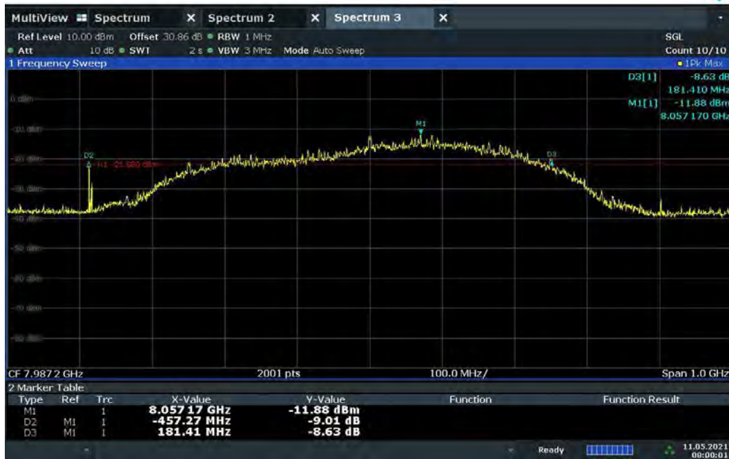
Plot 7-59. BANDWIDTH Plot – CH.9 – SP1 – Preamble 27
