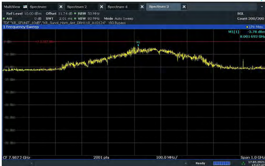
Plot 7-65. UWB Peak Power Measurement - ANT 2 - CH.9 – BPRF
