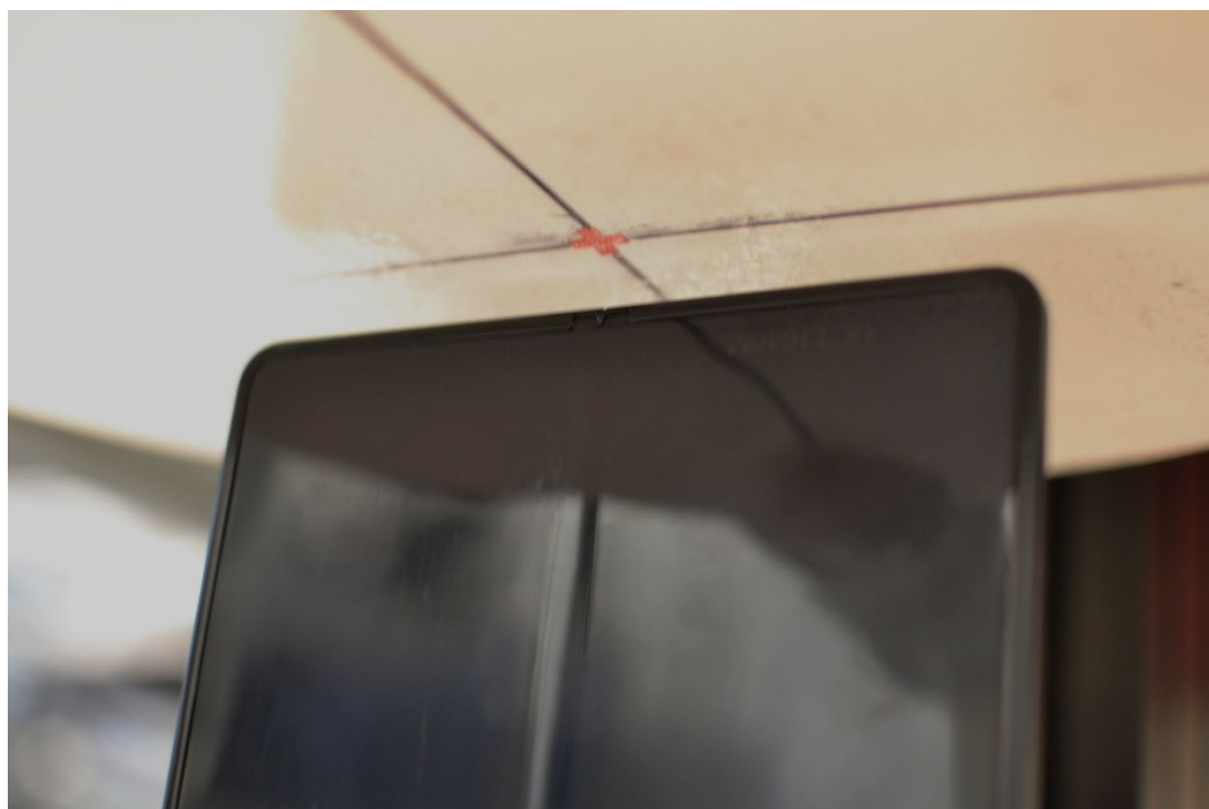
Figure C-17 SAR Test Setup Photo – UMPC Body, Bottom Edge at 10mm
