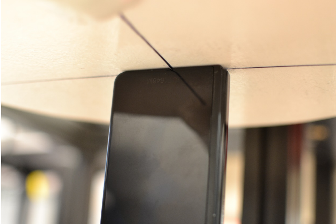
Figure C-12 SAR Test Setup Photo – Phablet, Bottom Edge at 0mm
