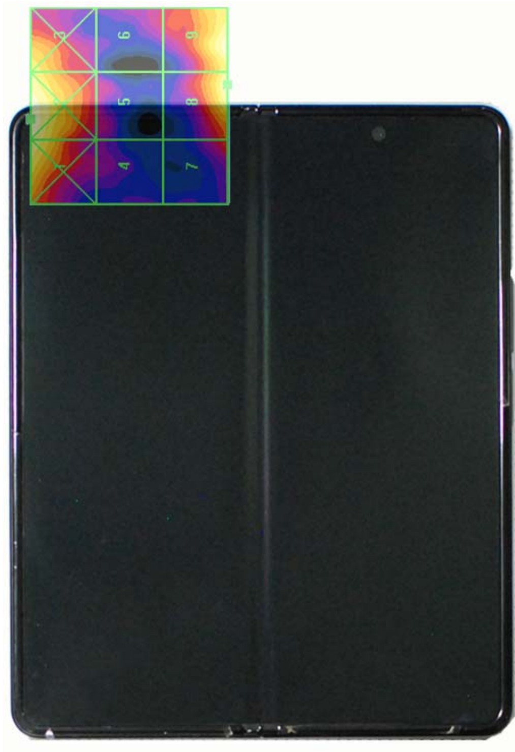
Figure 17-7 E-Field WD Scan overlay (FLAT – FRONT) (Acoustic Centered Scan Area pictured)
