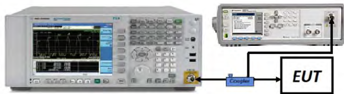
Figure 7-1. Test Instrument & Measurement Setup
