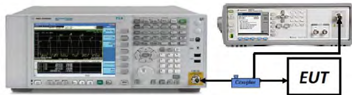
Figure 7-7. Test Instrument & Measurement Setup
