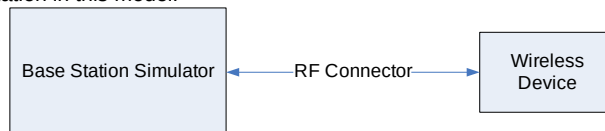
Figure 9-3 Power Measurement Setup
