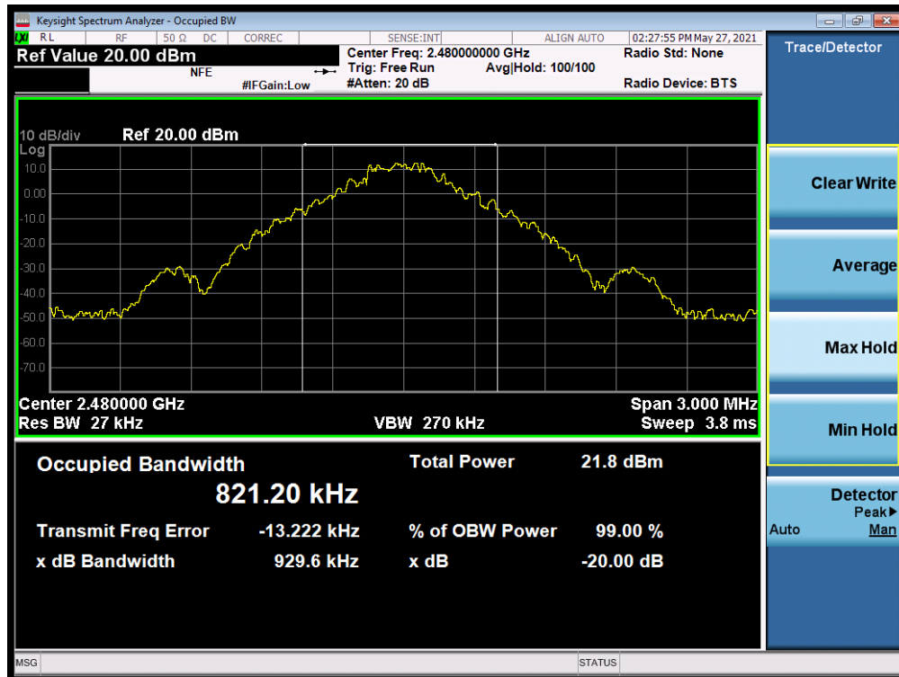
Plot 7-12. 20dB Bandwidth Plot (Bluetooth, 1Mbps – Ch. 78) Antenna 1
