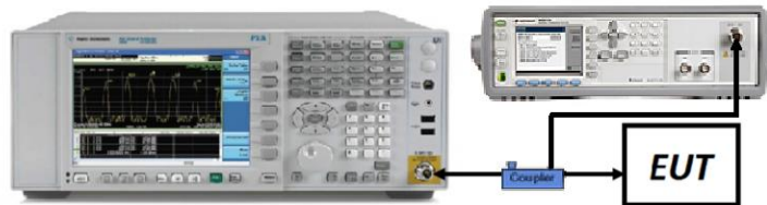
Figure 7-2. Test Instrument & Measurement Setup
