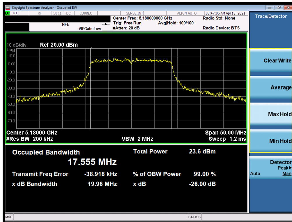
Plot 7-4. 26dB Bandwidth Plot SISO ANT1 (20MHz BW 802.11n (UNII Band 1) – Ch. 36)
