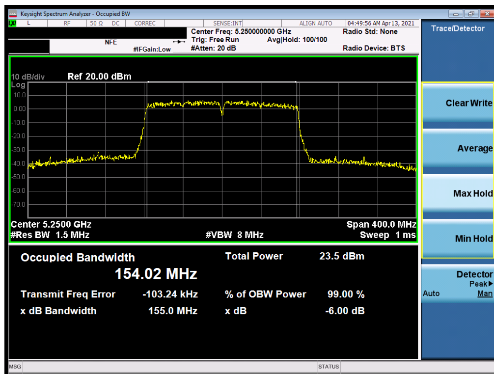
Plot 7-16. 26dB Bandwidth Plot SISO ANT1 (160MHz BW 802.11ac (UNII Band 1/2A) – Ch. 50)
