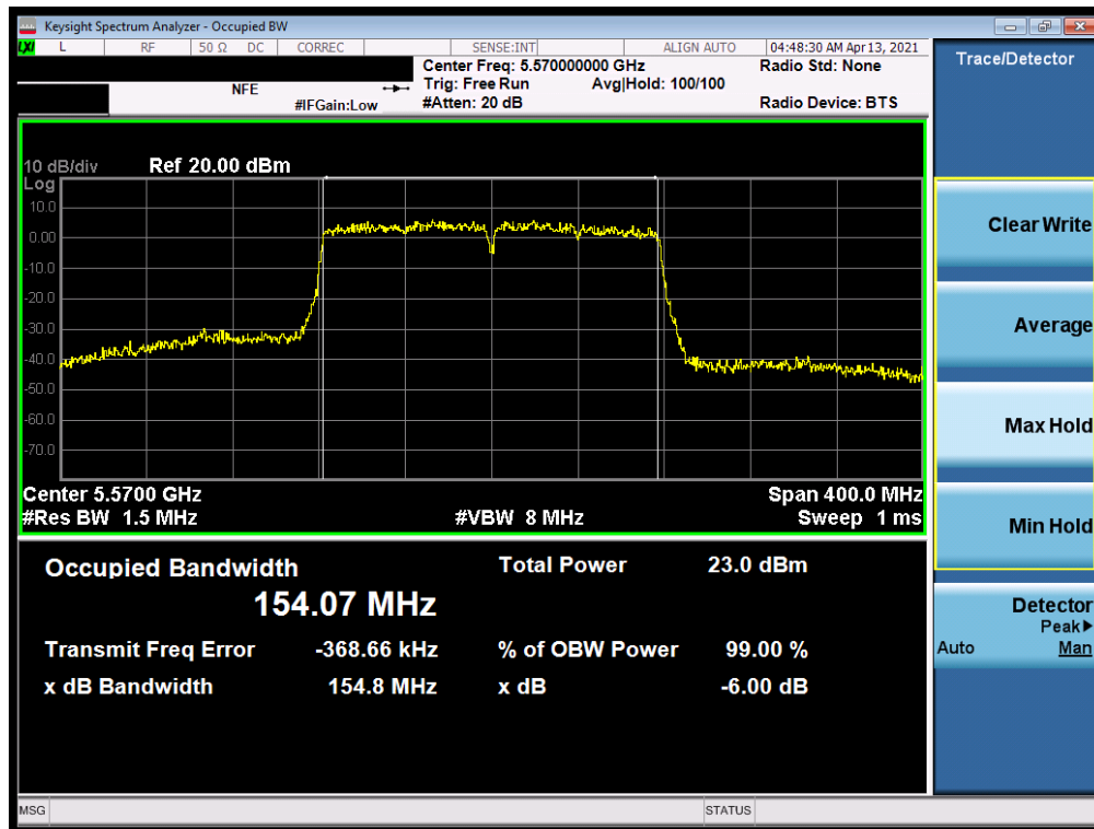
Plot 7-54. 26dB Bandwidth Plot SISO ANT1 (160MHz BW 802.11ac (UNII Band 2C) – Ch. 114)
