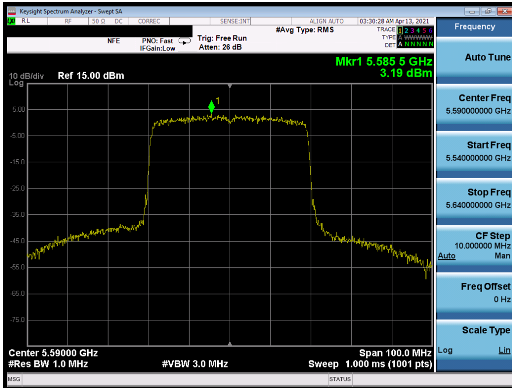
Plot 7-256. Power Spectral Density Plot SISO ANT1 (40MHz BW 802.11ax (UNII Band 2C) – Ch. 118)
