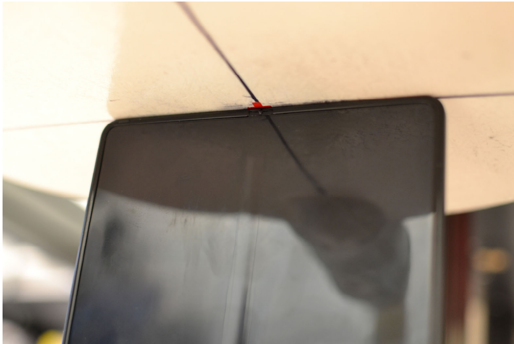
SAR Test Setup Photo 16– Open Configuration (UMPC), UMPC Extremity, Bottom Edge, 0 mm
