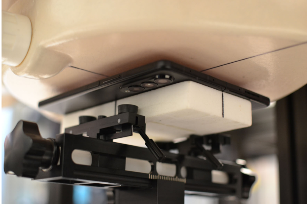
SAR Test Setup Photo 13– Open Configuration (UMPC), UMPC Body, Front Side, 10 mm
