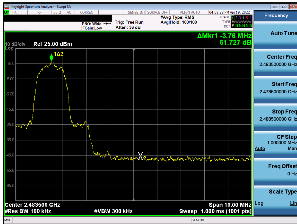
Plot 7-56. Band Edge Plot (Bluetooth with Hopping Disabled, 3 Mbps – Ch. 78) – Ant 1
