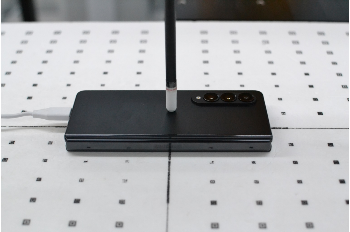
Figure F-25 Near Field Power Density Test Setup Photo – Back Side Closed at 2 mm
