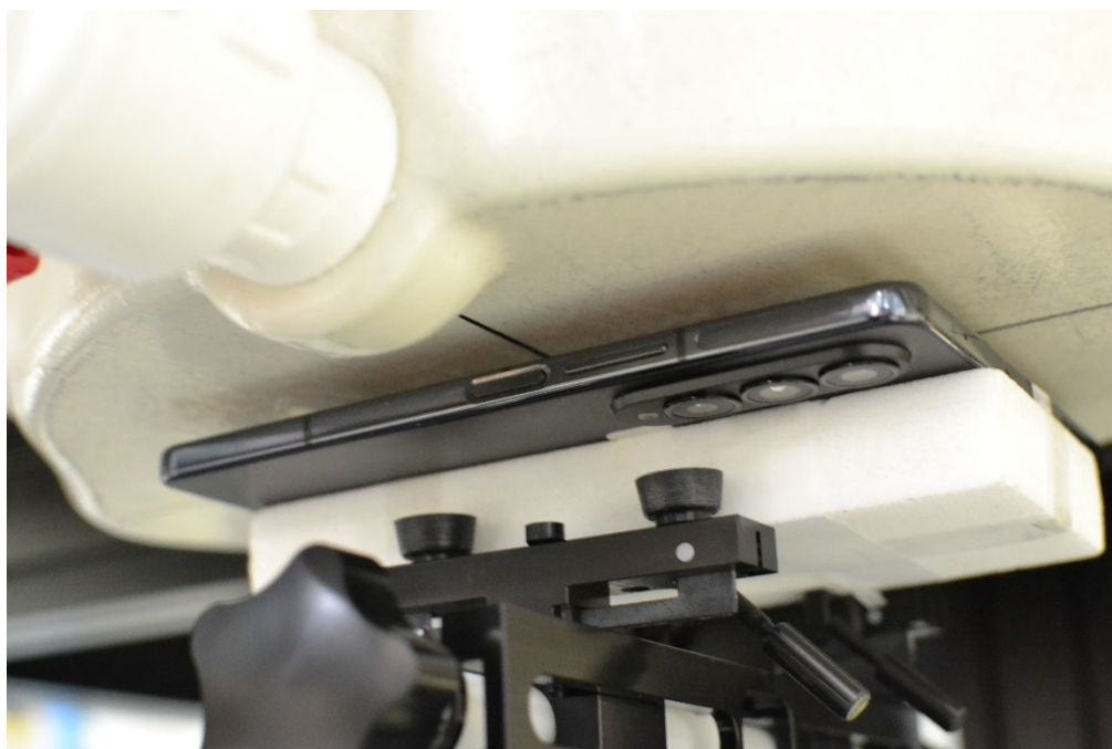
SAR Test Setup Photo 24– Open Configuration (UMPC), UMPC Body, Front Side, 10 mm
