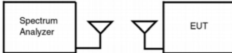
Figure 7-2. Test Instrument and Measurement Setup
