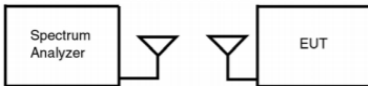
Figure 7-1. Test Instrument and Measurement Setup
