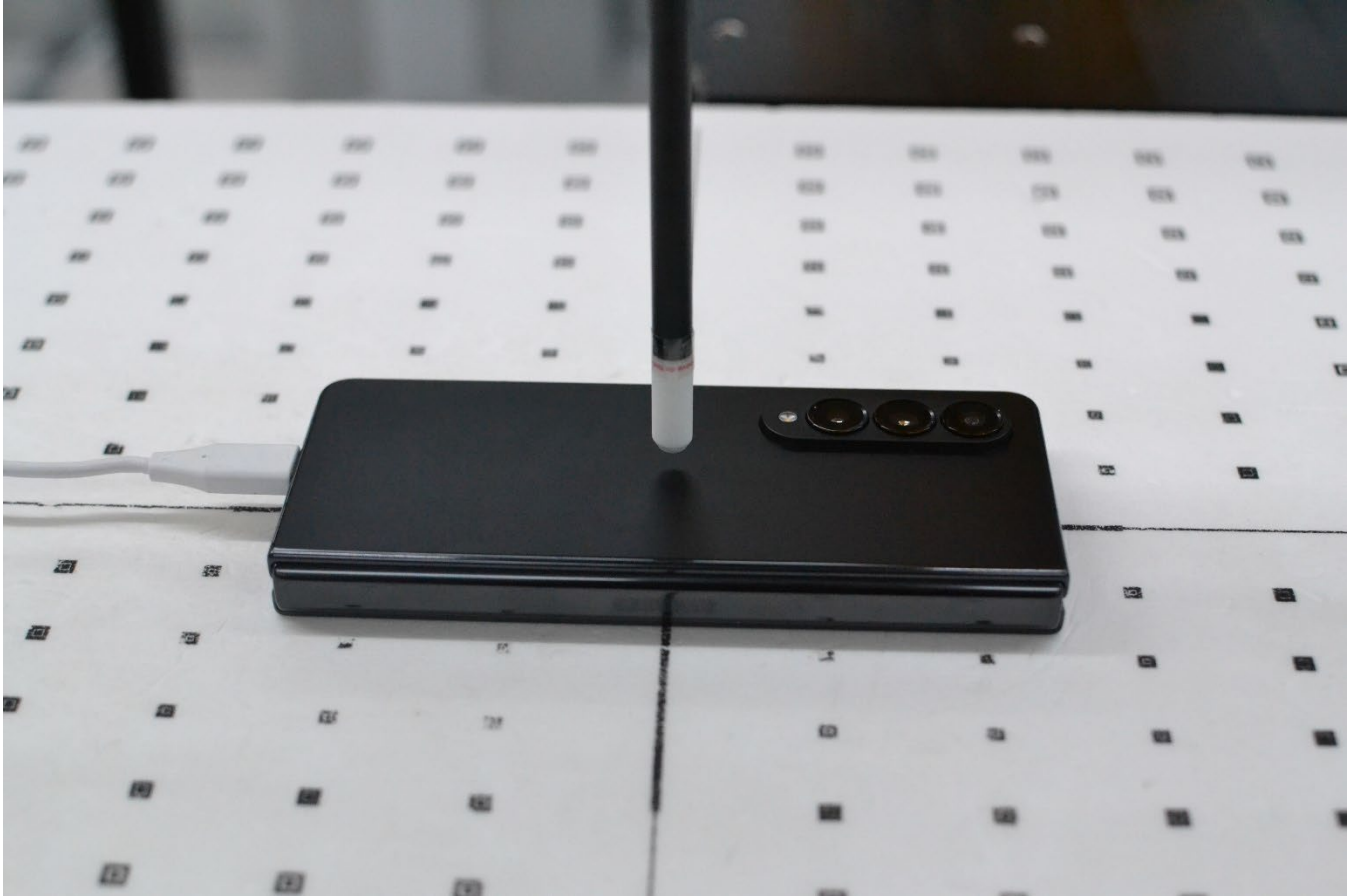
Figure F-27 Near Field Power Density Test Setup Photo – Back Side Closed at 10 mm
