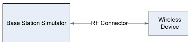
Figure 10-4 Power Measurement Setup – NR FDD
