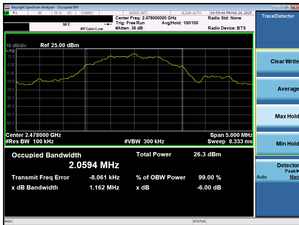
Plot 7-12. 6dB Bandwidth Plot (Bluetooth (LE), 2Mbps – Ch. 36) – Ant 1
