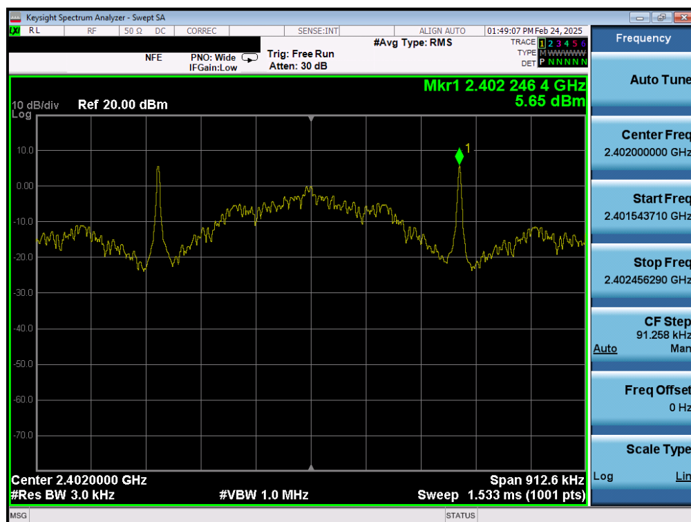
Plot 7-73. Power Spectral Density Plot (Bluetooth (LE), 125kbps – Ch. 37) – Ant 1
