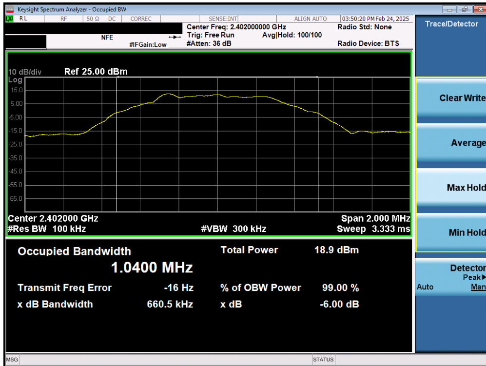
Plot 7-16. 6dB Bandwidth Plot (Bluetooth (LE), 500kbps – Ch. 37) – Ant 2
