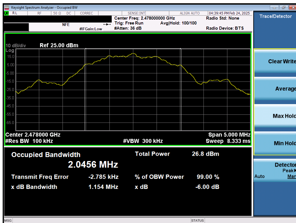
Plot 7-24. 6dB Bandwidth Plot (Bluetooth (LE), 2Mbps – Ch. 36) – Ant 2
