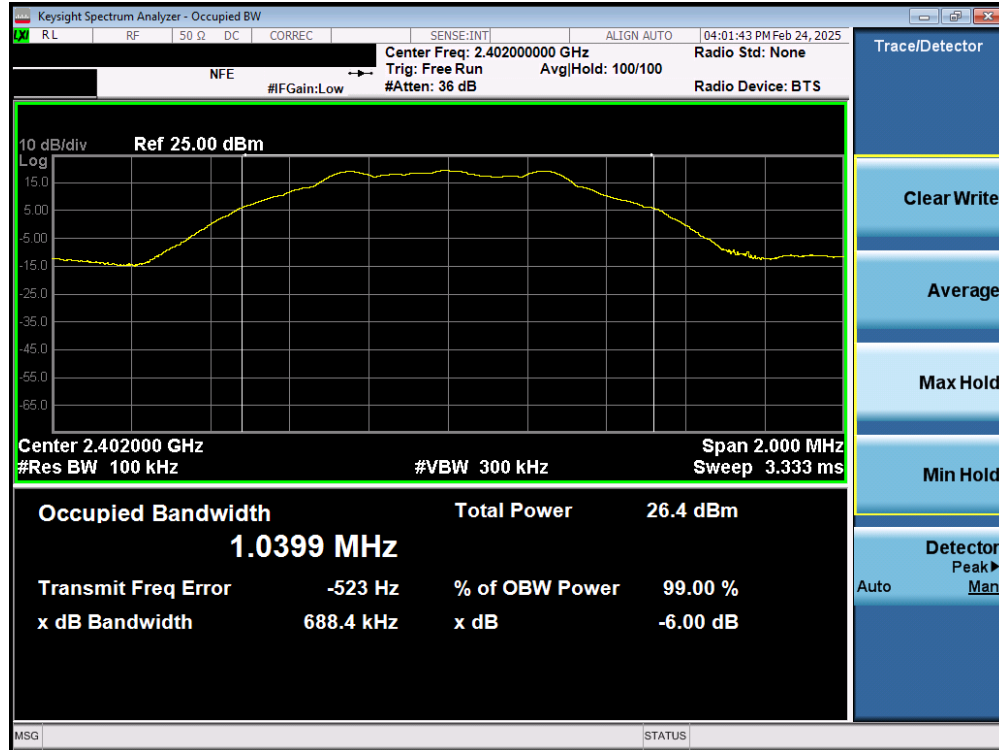
Plot 7-19. 6dB Bandwidth Plot (Bluetooth (LE), 1Mbps – Ch. 37) – Ant 2
