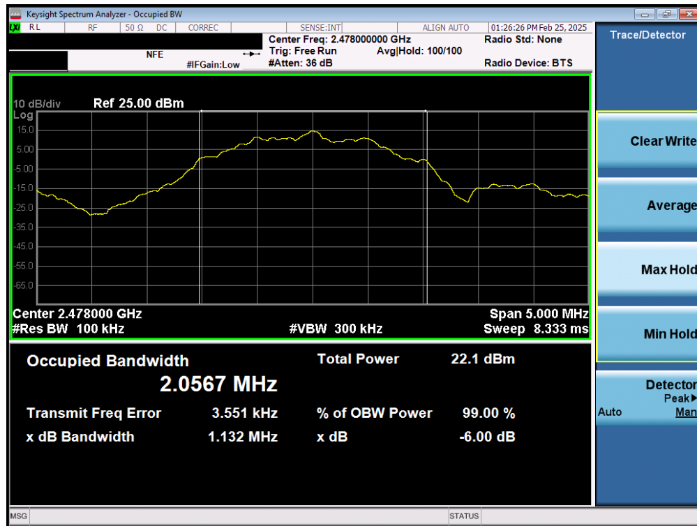
Plot 7-36. 6dB Bandwidth Plot (Bluetooth (LE), 2Mbps – Ch. 36) – Dual Ant 2
