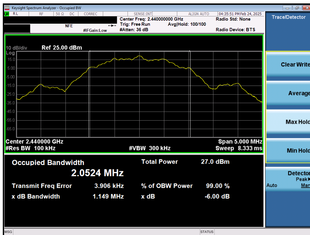
Plot 7-23. 6dB Bandwidth Plot (Bluetooth (LE), 2Mbps – Ch. 17) – Ant 2
