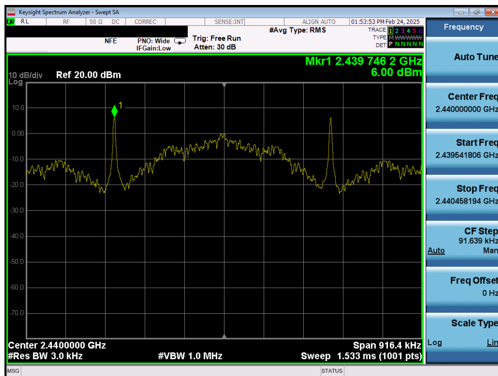
Plot 7-74. Power Spectral Density Plot (Bluetooth (LE), 125kbps – Ch. 17) – Ant 1
