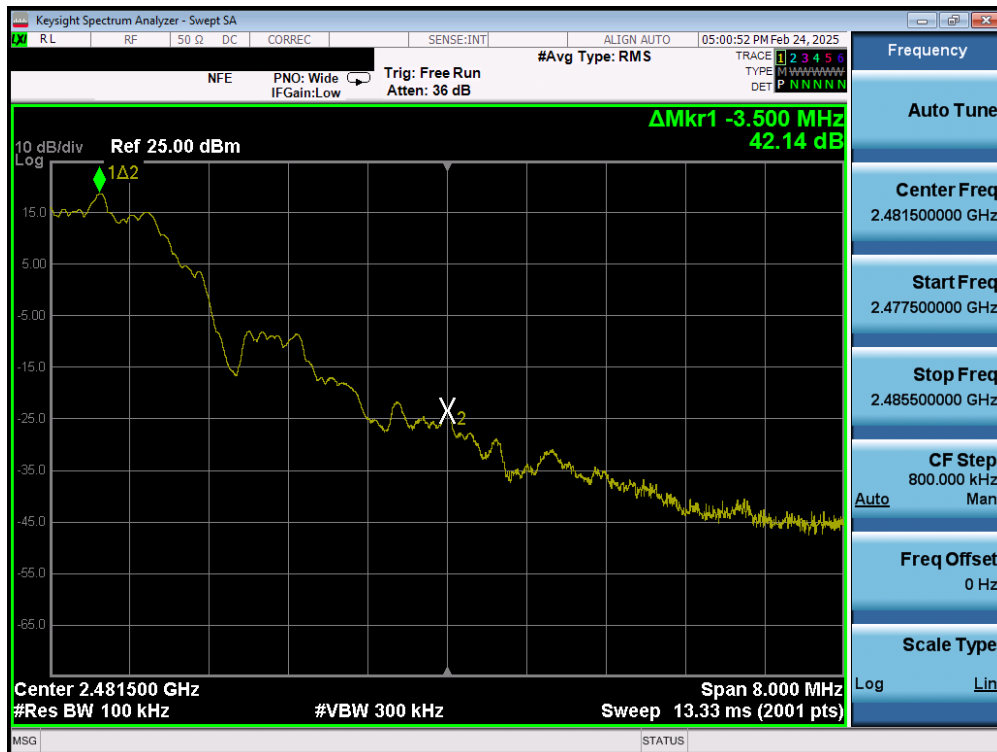
Plot 7-116. Band Edge Plot (Bluetooth (LE), 2Mbps – Ch. 36) – Ant 1
