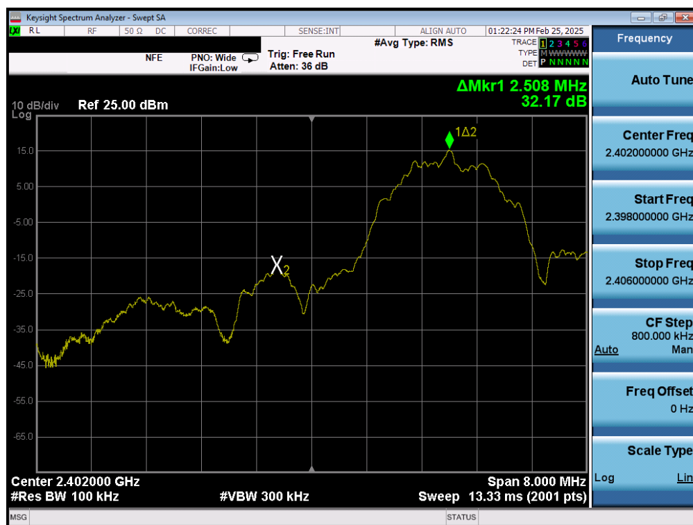
Plot 7-131. Band Edge Plot (Bluetooth (LE), 2Mbps – Ch. 0) – Dual Ant 2
