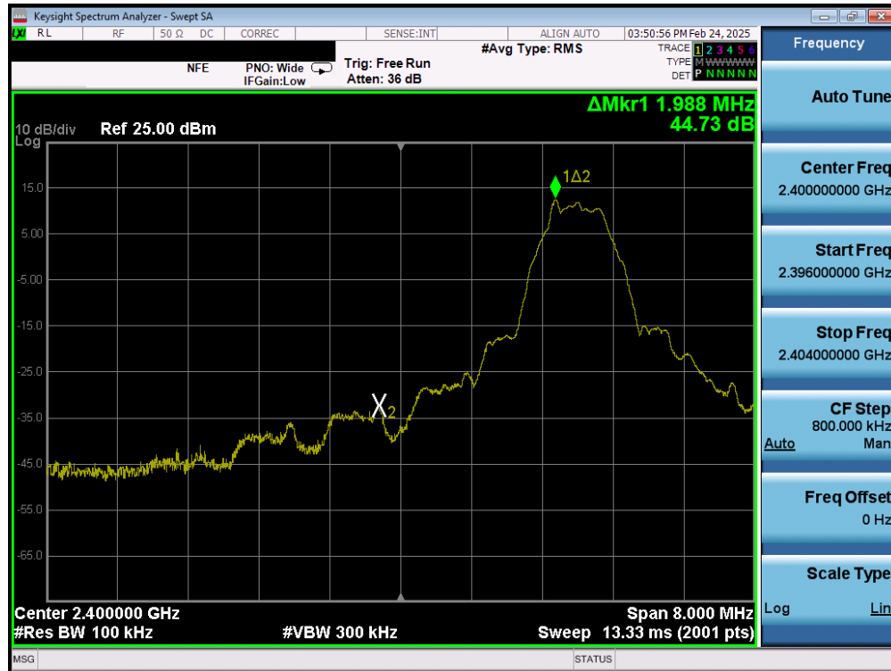
Plot 7-119. Band Edge Plot (Bluetooth (LE), 500kbps – Ch. 37) – Ant 2
