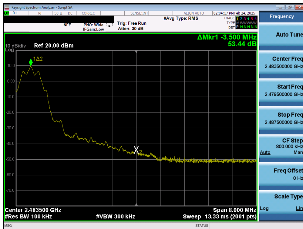
Plot 7-110. Band Edge Plot (Bluetooth (LE), 125kbps – Ch. 39) – Ant 1
