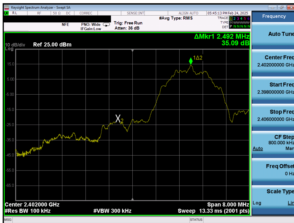
Plot 7-127. Band Edge Plot (Bluetooth (LE), 2Mbps – Ch. 37) – Dual Ant 1
