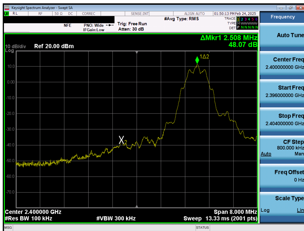
Plot 7-109. Band Edge Plot (Bluetooth (LE), 125kbps – Ch. 37) – Ant 1
