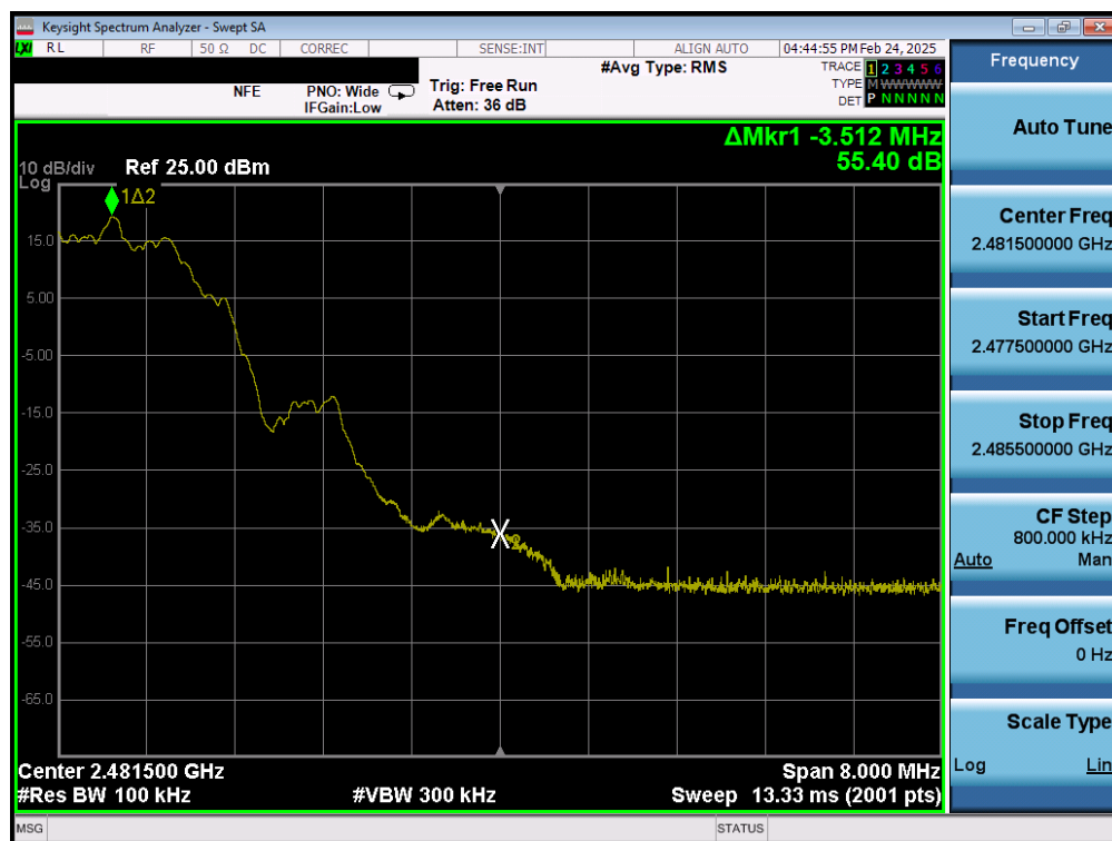
Plot 7-124. Band Edge Plot (Bluetooth (LE), 2Mbps – Ch. 36) – Ant 2
