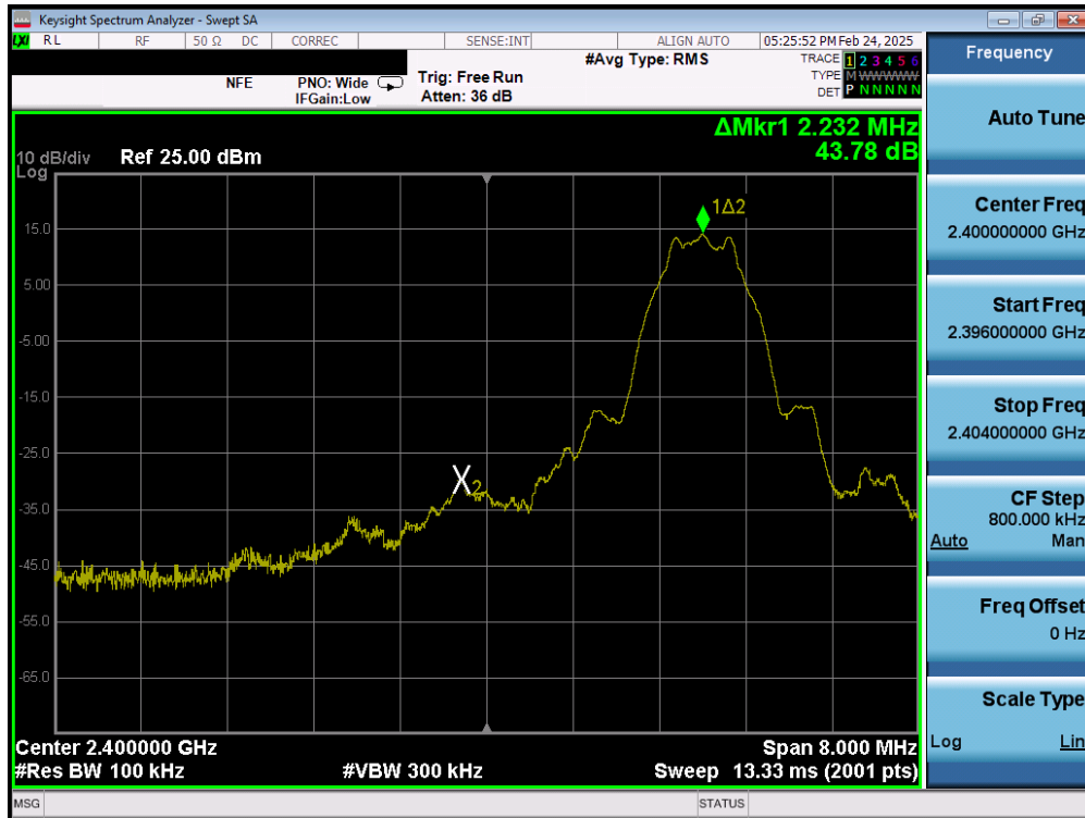
Plot 7-125. Band Edge Plot (Bluetooth (LE), 1Mbps – Ch. 37) – Dual Ant 1
