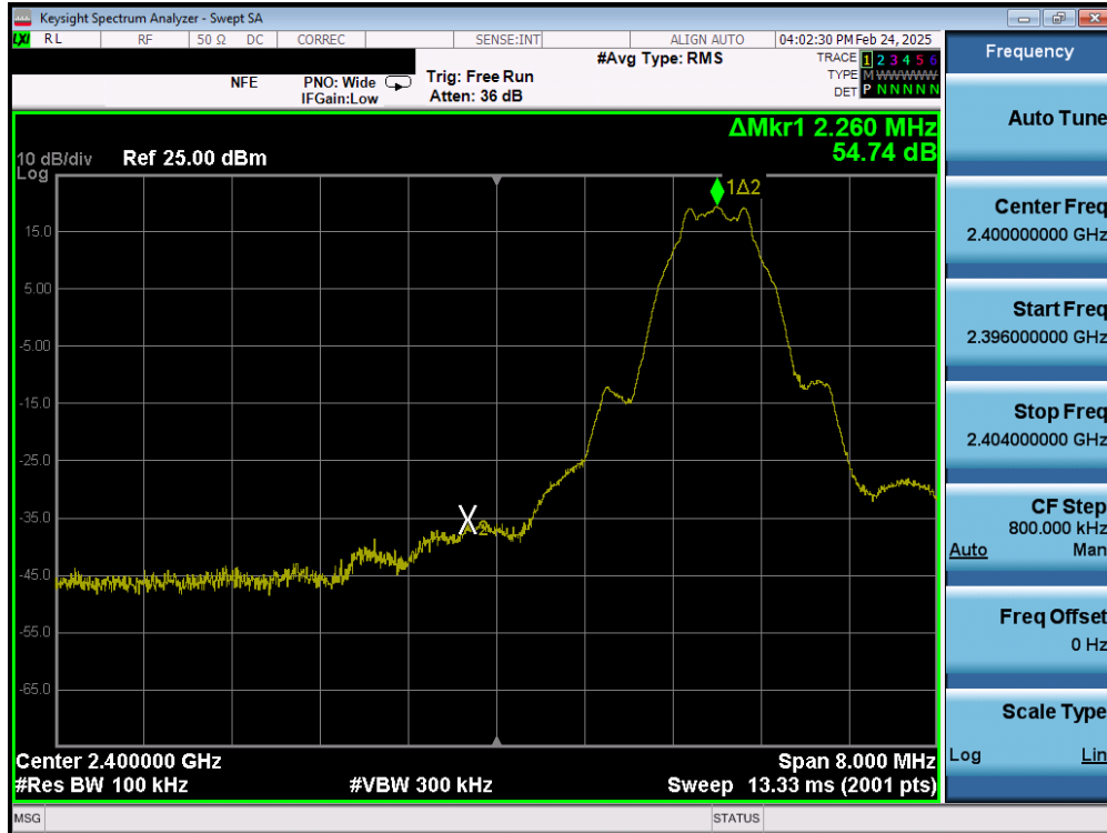
Plot 7-121. Band Edge Plot (Bluetooth (LE), 1Mbps - Ch. 37) - Ant 2
