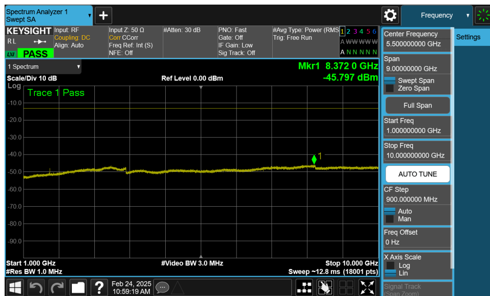
Plot 7-71. Conducted Spurious Plot (LTE Band 26/5 - 10MHz QPSK - 1 RB - Mid Channel – Ant2)
