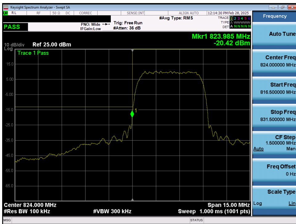
Plot 7-77. Lower Band Edge Plot (WCDMA Cell – Ch. 4132 – Ant1)
