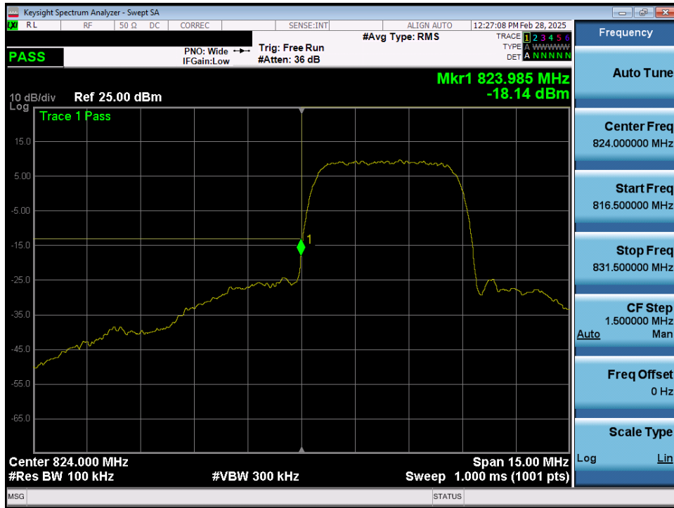
Plot 7-85. Lower Band Edge Plot (WCDMA Cell – Ch. 4132 – Ant2)
