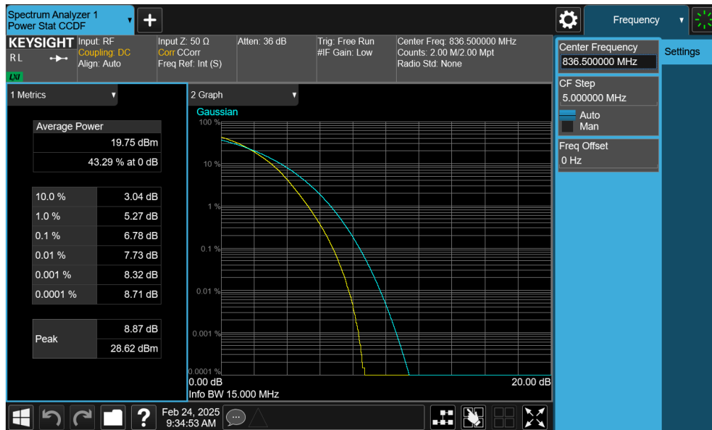
Plot 7-95. Peak-Average Ratio Plot (LTE Band 26 - 15MHz 256-QAM - Full RB - Ant1)
