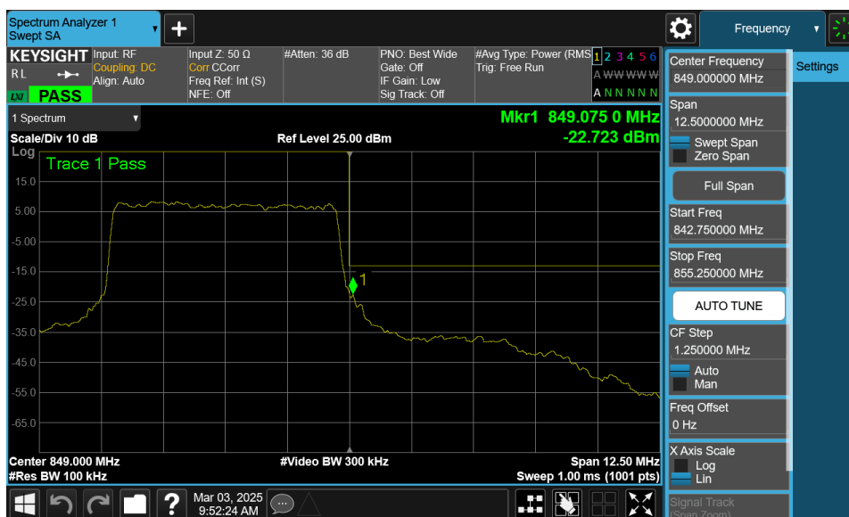
Plot 7-90. Upper Band Edge Plot (NR Band n5 – 5.0MHz - Full RB - Ant2)
