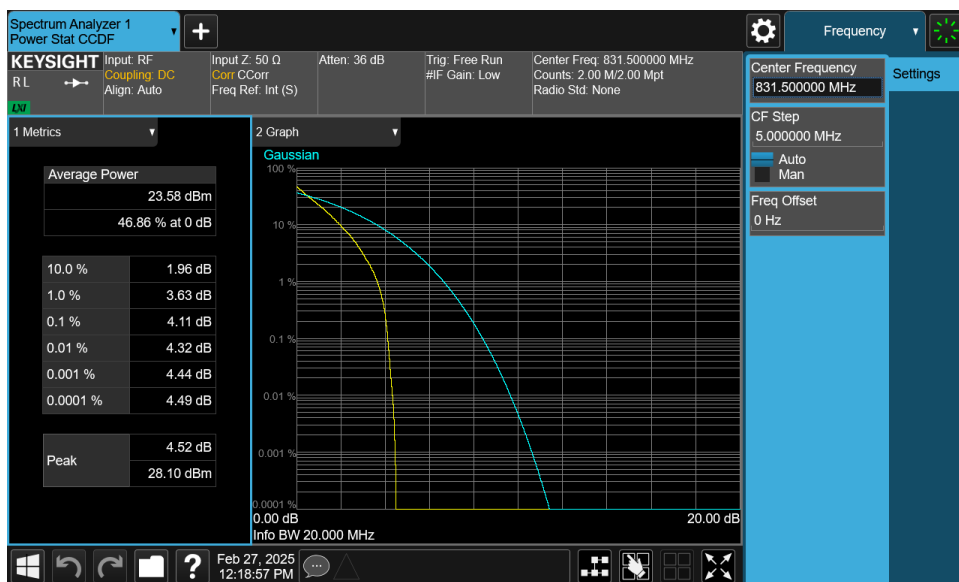
Plot 7-106. Peak-Average Ratio Plot (NR Band n5 - 20MHz \pi/2 BPSK - Full RB - Ant2)
