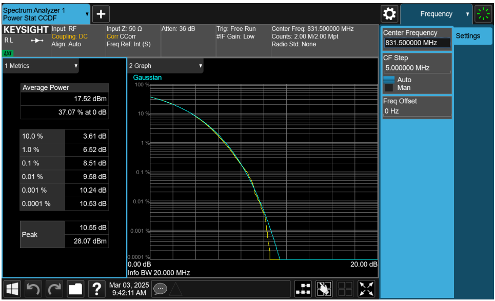
Plot 7-108. Peak-Average Ratio Plot (NR Band n5 - 20MHz 256-QAM - Full RB - Ant2)
