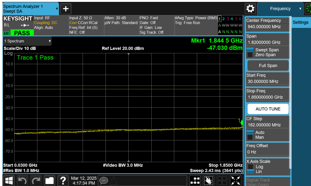
Plot 7-121. Conducted Spurious Plot (NR Band n25/2 -40.0MHz - 1RB - Low Channel - Ant2)
