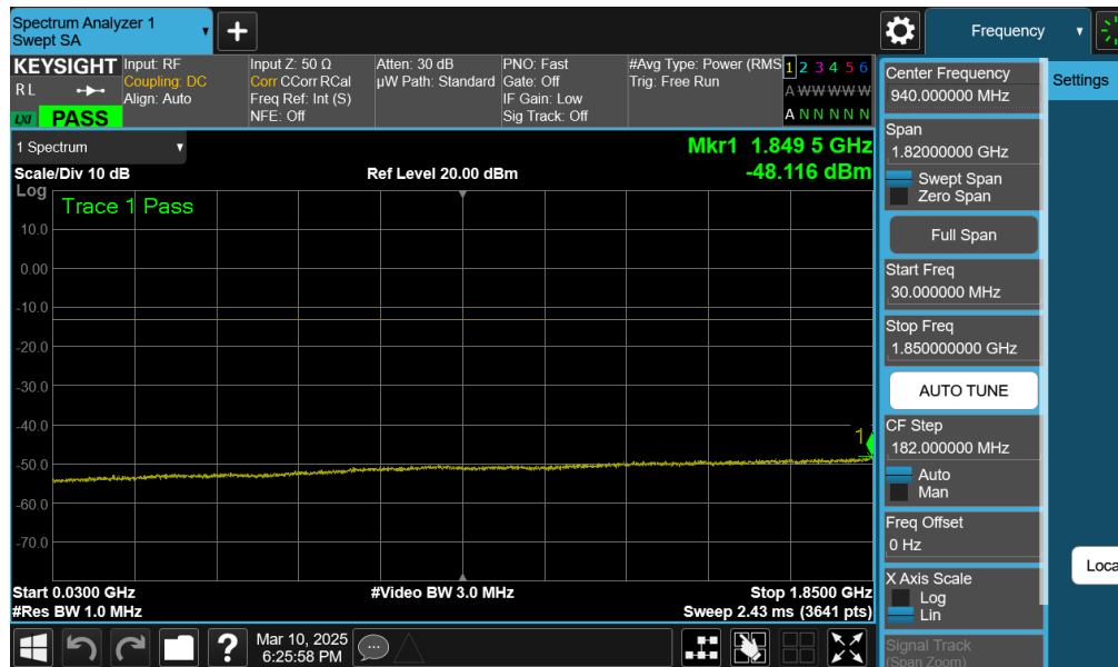
Plot 7-103. Conducted Spurious Plot (NR Band n25/2 -40.0MHz - 1RB - Low Channel - Ant1)
