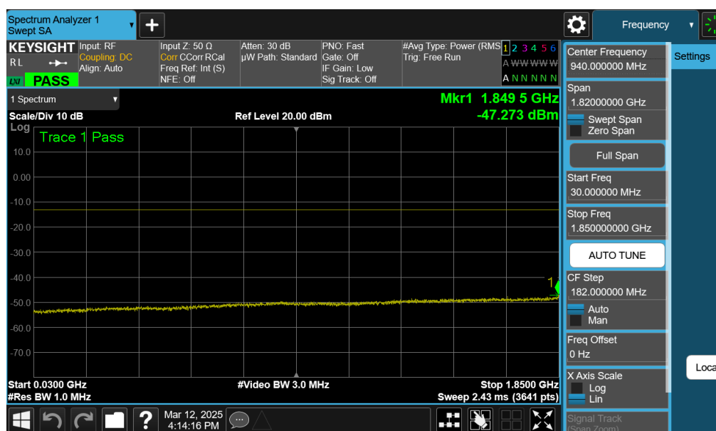
Plot 7-124. Conducted Spurious Plot (NR Band n25/2 - 40.0MHz - 1RB - Mid Channel - Ant2)
