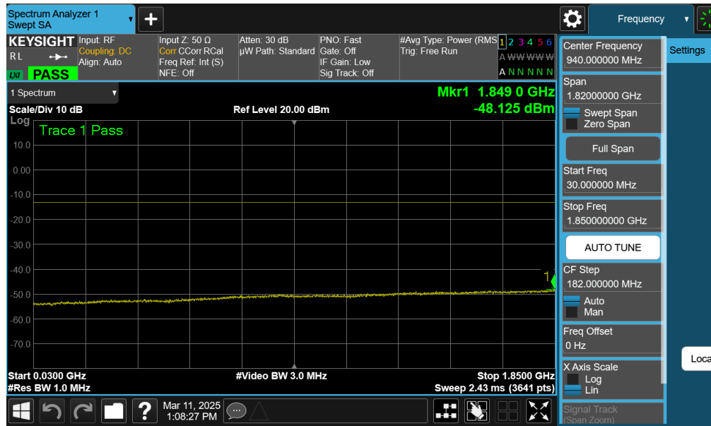
Plot 7-109. Conducted Spurious Plot (NR Band n25/2 - 40.0MHz - 1RB - High Channel - Ant1)
