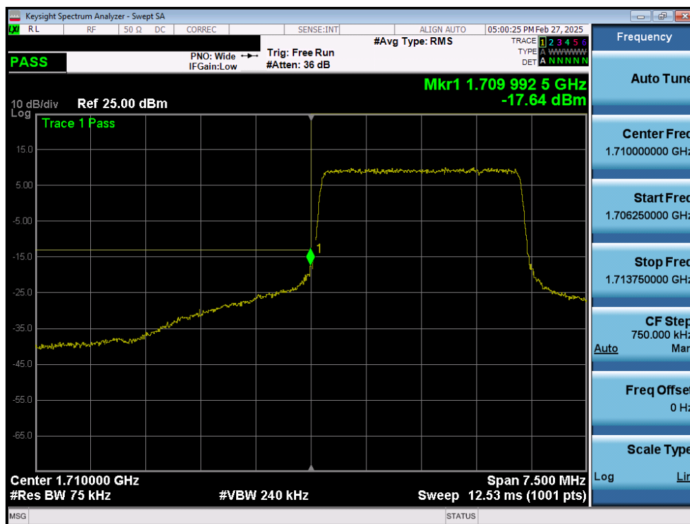
Plot 7-207. Lower Band Edge Plot (LTE Band 66/4 - 3MHz QPSK – Full RB - ANT2)
