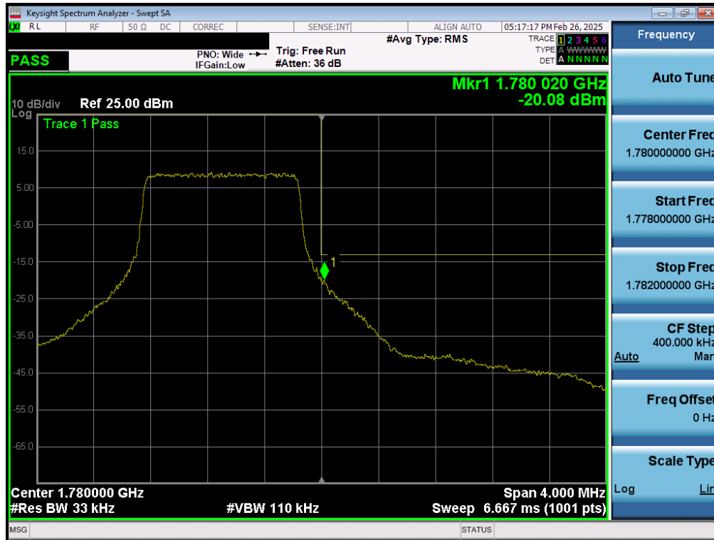
Plot 7-193. Upper Band Edge Plot (LTE Band 66 – 1.4MHz QPSK – Full RB - ANT1)
