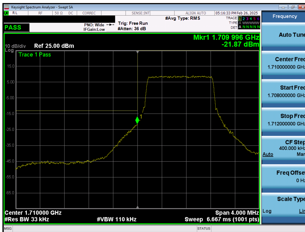
Plot 7-189. Lower Band Edge Plot (LTE Band 66/4 – 1.4MHz QPSK – Full RB - ANT1)
