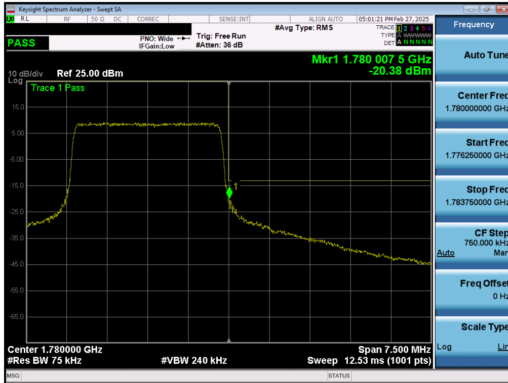
Plot 7-211. Upper Band Edge Plot (LTE Band 66 - 3MHz QPSK – Full RB - ANT2)
