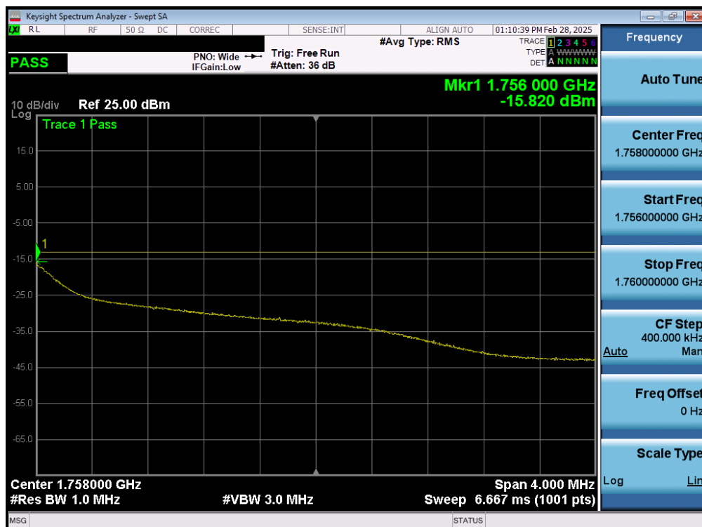
Plot 7-182. Upper Extended Band Edge Plot (WCDMA AWS – Ch. 1513– ANT1)
