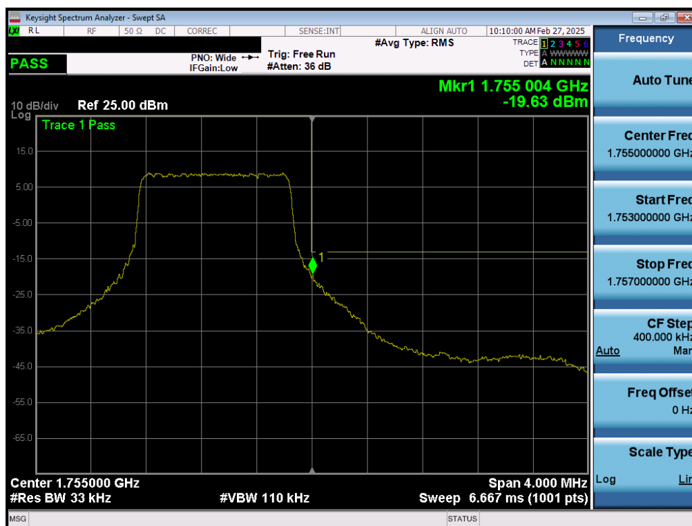
Plot 7-191. Upper Band Edge Plot (LTE Band 4 – 1.4MHz QPSK – Full RB - ANT1)
