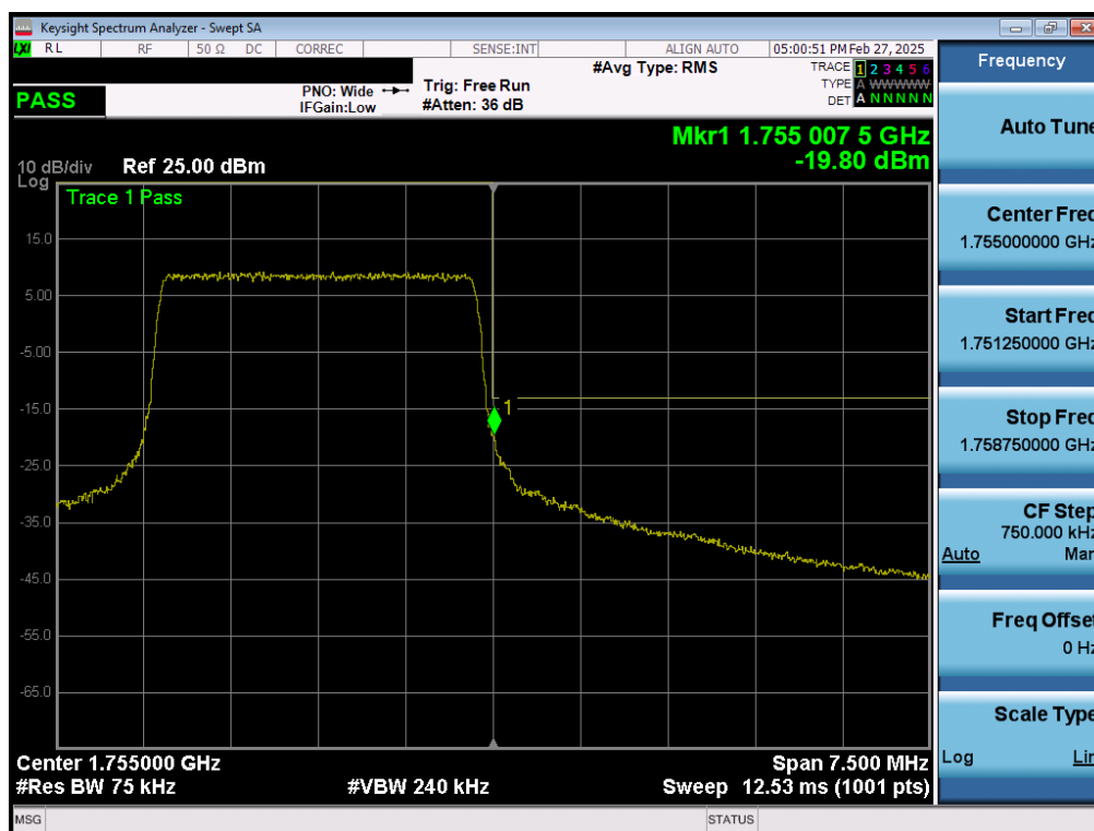
Plot 7-209. Upper Band Edge Plot (LTE Band 4 - 3MHz QPSK – Full RB - ANT2)
