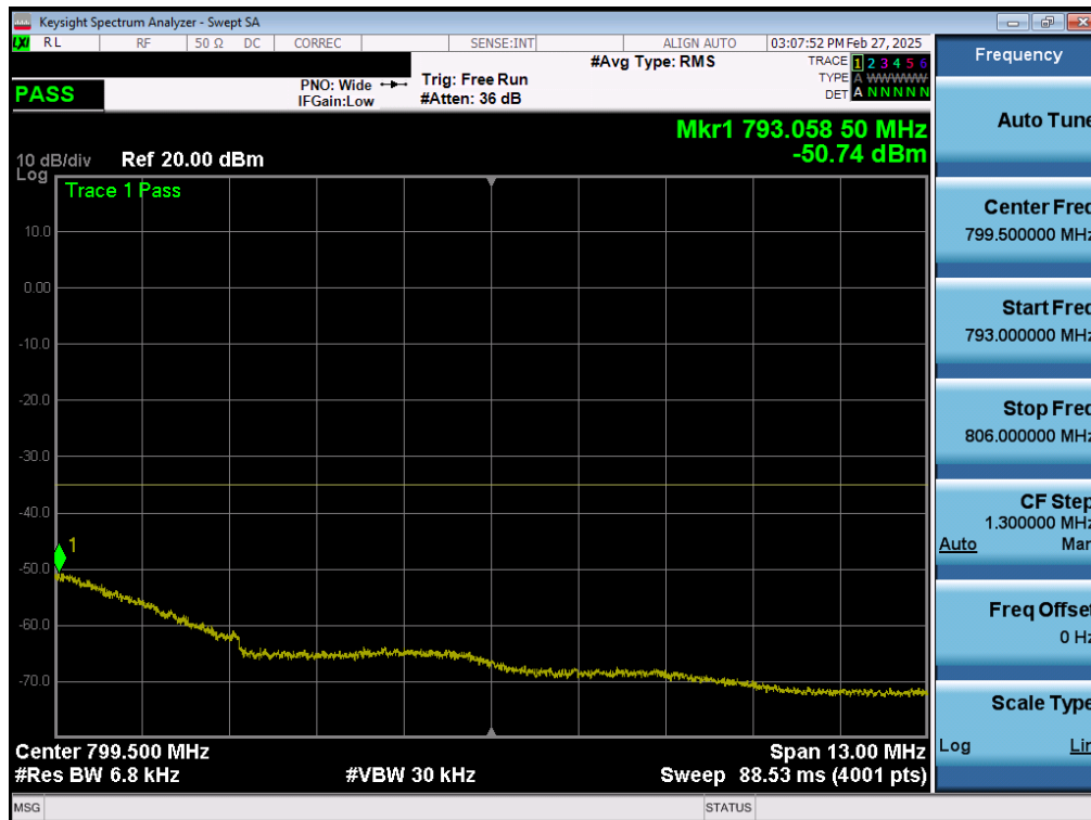
Plot 7-206. Upper Emission Mask Plot (LTE Band 13 - 5MHz QPSK - Full RB - ANT2)
