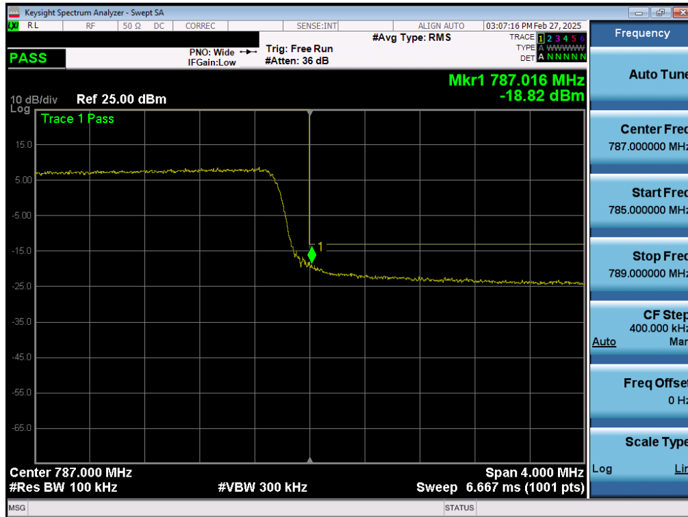
Plot 7-205. Upper Band Edge Plot (LTE Band 13 - 5MHz QPSK - Full RB - ANT2)
