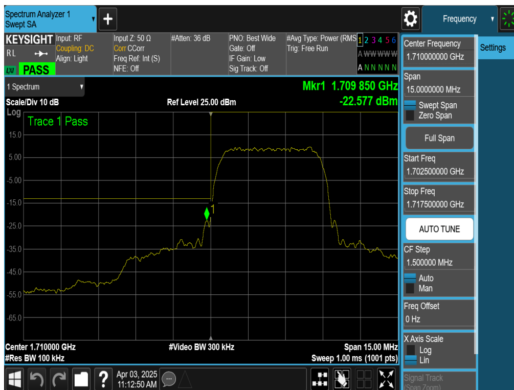
Plot 7-179. Lower Band Edge Plot (WCDMA AWS – Ch. 1312 – ANT1)
