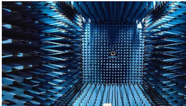
Figure 2: Geometry of Anechoic Chamber for Radiation patterns.
