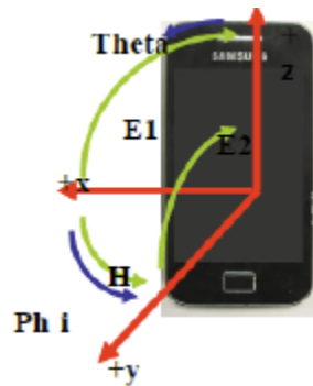
Figure 1 : Geometry for SC-56F for Radiation patterns
