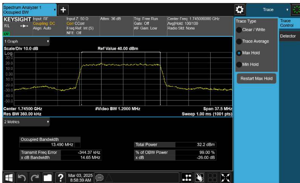
Plot 7-40. Occupied Bandwidth Plot (NR Band n66 - 15.0MHz DFT-s-OFDM BPSK - Full RB – ANT1)
