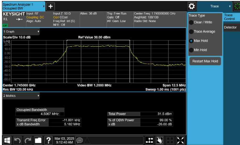
Plot 7-47. Occupied Bandwidth Plot (NR Band n66 - 5.0MHz CP-OFDM QPSK - Full RB – ANT1)
