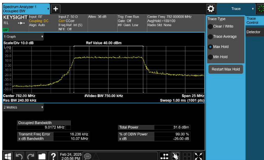
Plot 7-10. Occupied Bandwidth Plot (LTE Band 13 - 10MHz 16-QAM - Full RB – ANT1)
