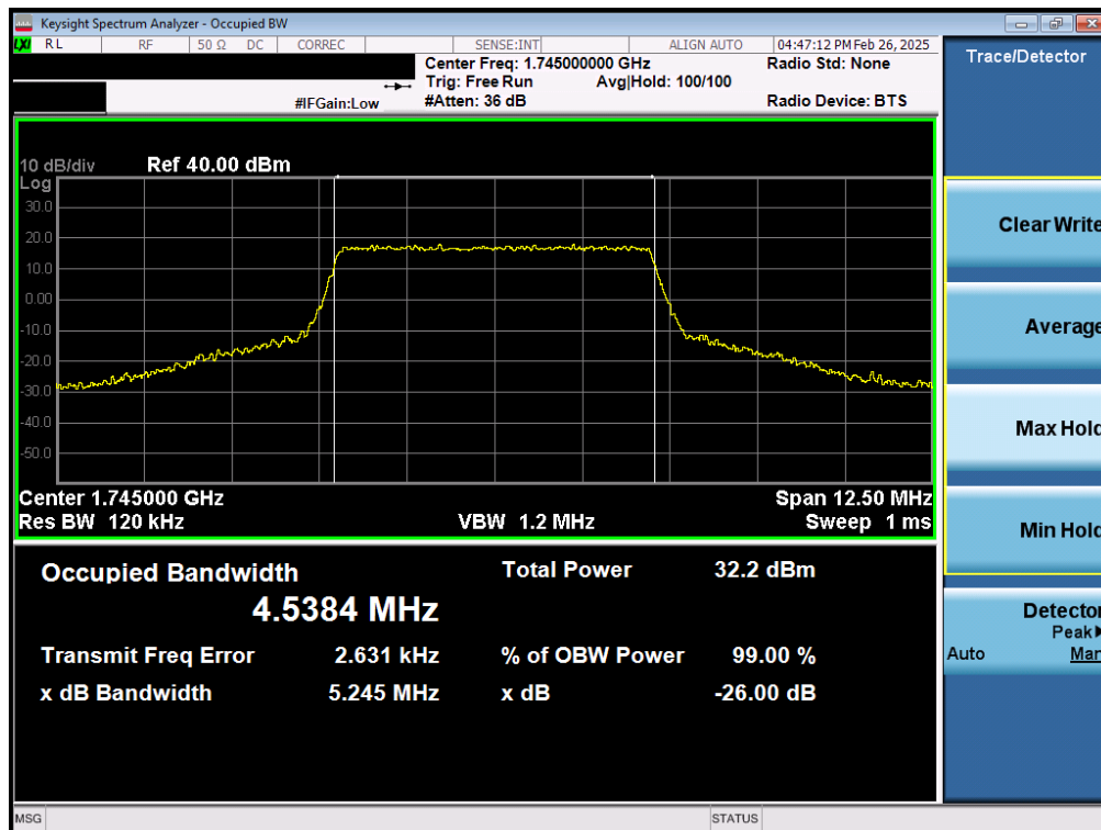
Plot 7-20. Occupied Bandwidth Plot (LTE Band 66/4 - 5MHz 16-QAM - Full RB - ANT1)
