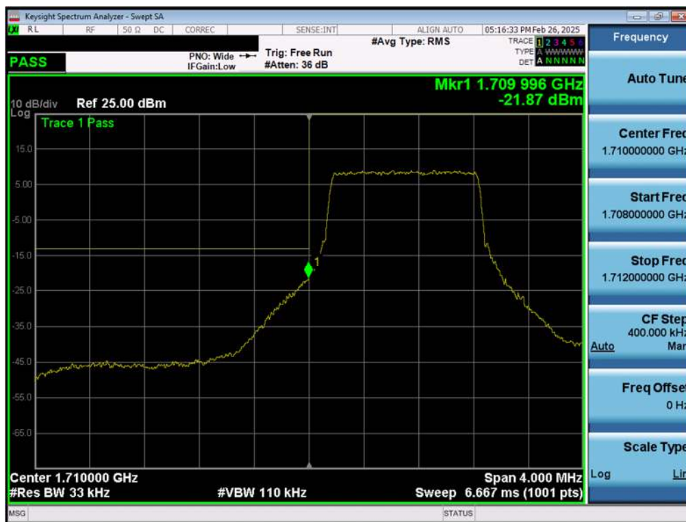
Plot 7-94. Lower Band Edge Plot (LTE Band 66/4 – 1.4MHz QPSK – Full RB - ANT1)
