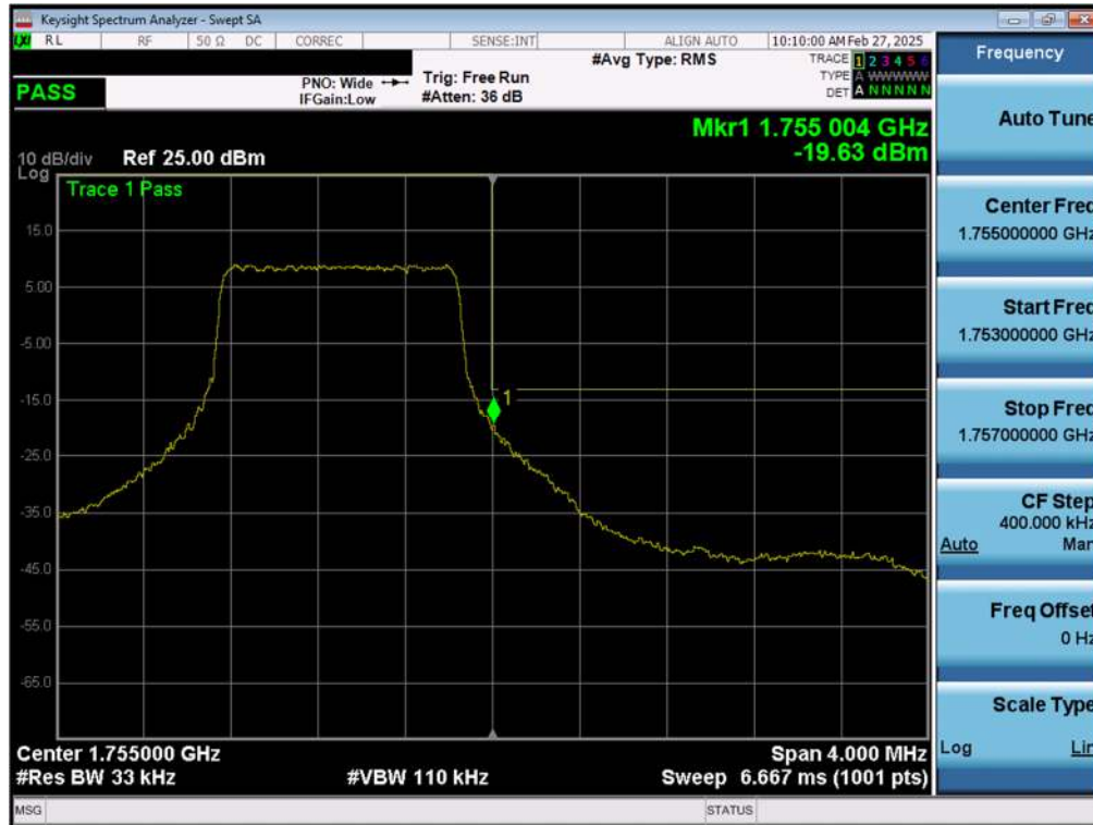
Plot 7-96. Upper Band Edge Plot (LTE Band 4 – 1.4MHz QPSK – Full RB - ANT1)
