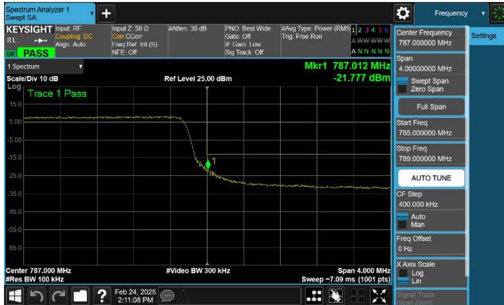
Plot 7-92. Upper Band Edge Plot (LTE Band 13 - 5MHz QPSK – Full RB - ANT1)
