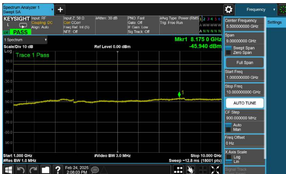
Plot 7-78. Conducted Spurious Plot (LTE Band 13 - 10MHz QPSK - 1 RB)
