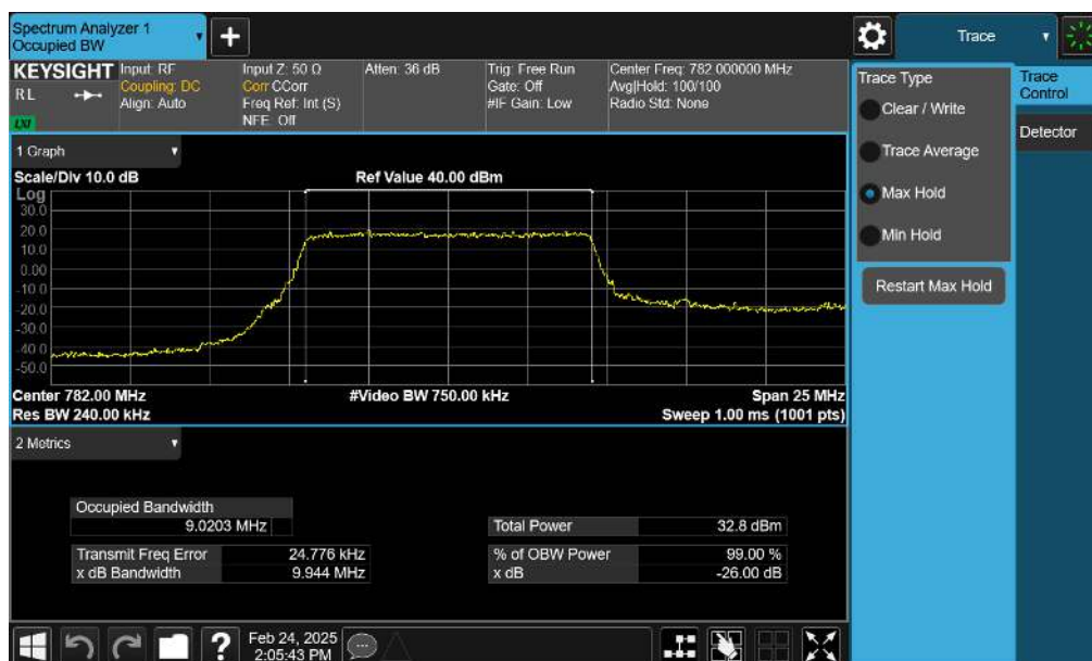
Plot 7-9. Occupied Bandwidth Plot (LTE Band 13 - 10MHz QPSK - Full RB – ANT1)
