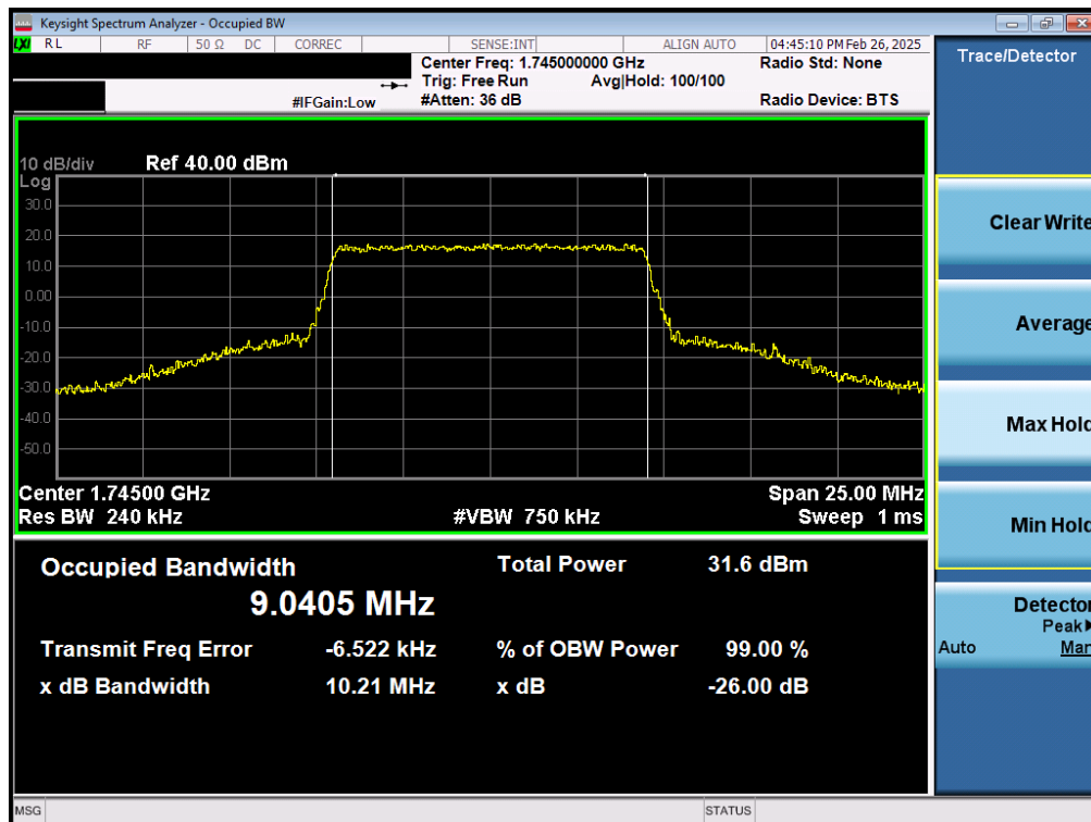
Plot 7-18. Occupied Bandwidth Plot (LTE Band 66/4 - 10MHz 16-QAM - Full RB - ANT1)
