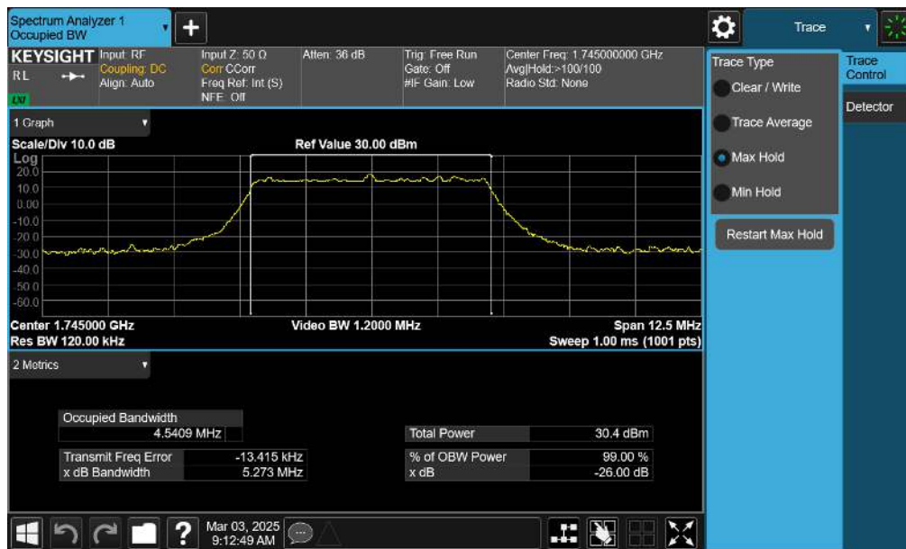
Plot 7-48. Occupied Bandwidth Plot (NR Band n66 - 5.0MHz CP-OFDM 16QAM - Full RB – ANT1)
