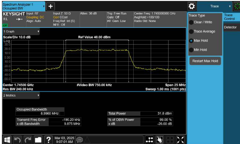
Plot 7-43. Occupied Bandwidth Plot (NR Band n66 - 10.0MHz DFT-s-OFDM BPSK - Full RB – ANT1)
