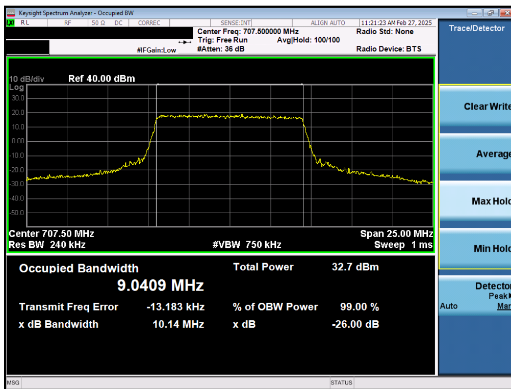
Plot 7-1. Occupied Bandwidth Plot (LTE Band 12 - 10MHz QPSK - Full RB – ANT1)
