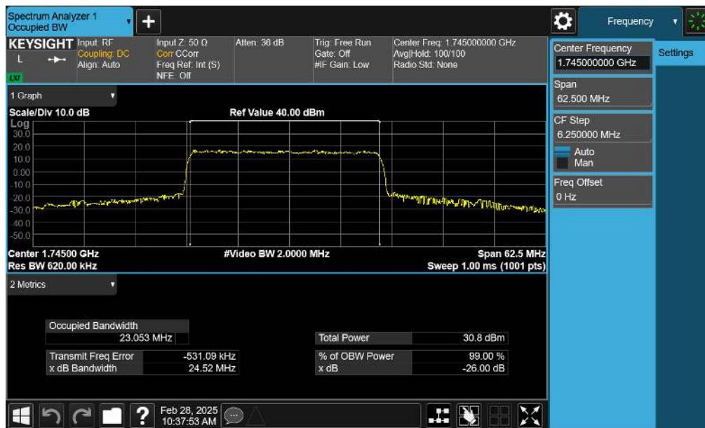
Plot 7-60. Occupied Bandwidth Plot (NR Band n66 - 25.0MHz CP-OFDM 16QAM - Full RB – ANT2)
