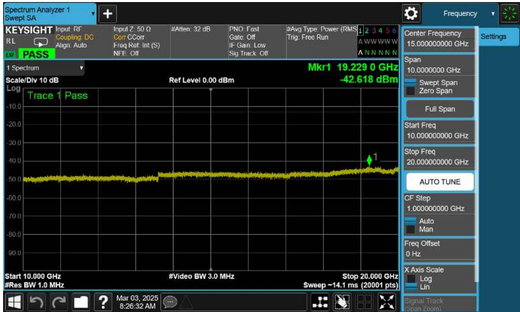
Plot 7-84. Conducted Spurious Plot (NR Band n66 - 40.0MHz - 1 RB - Low Channel - ANT1)
