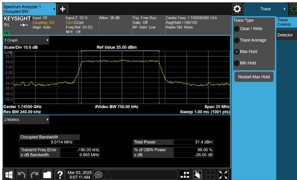
Plot 7-44. Occupied Bandwidth Plot (NR Band n66 - 10.0MHz CP-OFDM QPSK - Full RB – ANT1)
