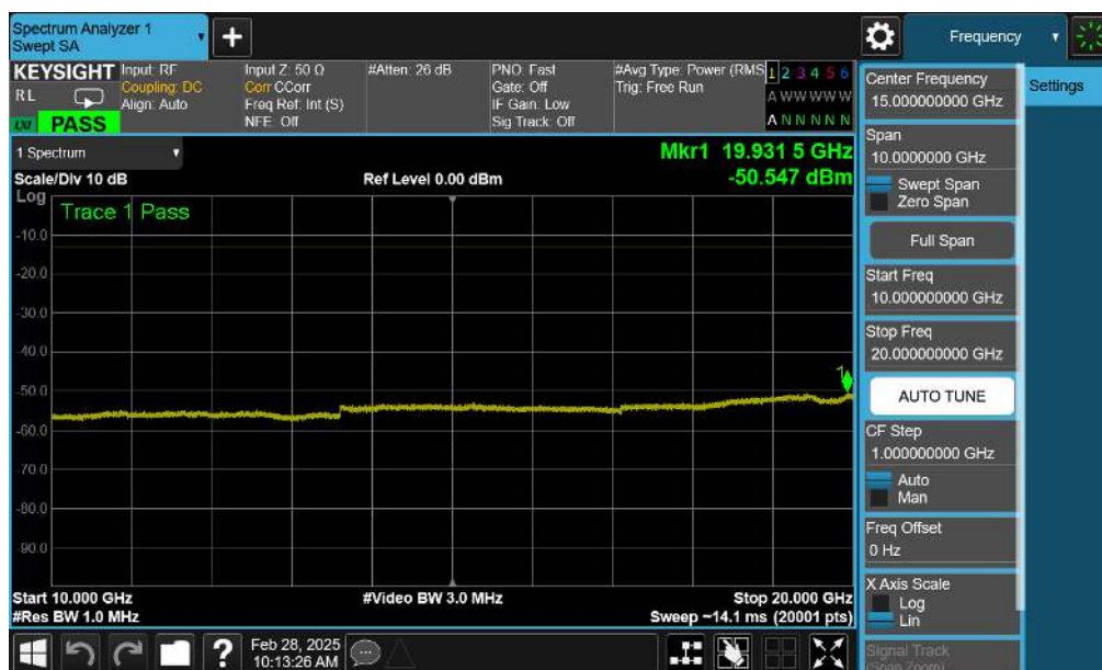
Plot 7-87. Conducted Spurious Plot (NR Band n66 - 40.0MHz - 1 RB - Mid Channel - ANT2)
