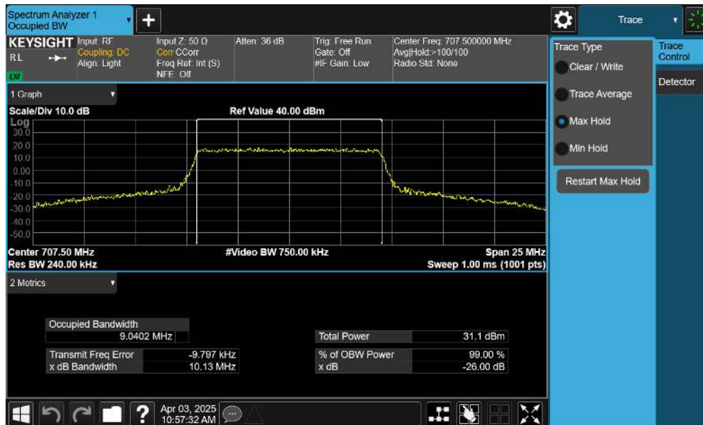
Plot 7-2. Occupied Bandwidth Plot (LTE Band 12 - 10MHz 16-QAM - Full RB – ANT1)
