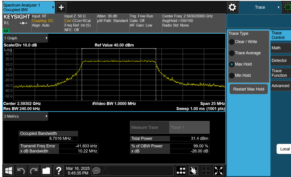
Plot 7-91. Occupied Bandwidth Plot (NR Band n41 PC2 – 10MHz QPSK – Full RB – Switch – Ant1)
