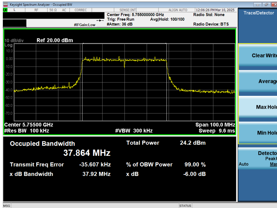
Plot 7-49. 6dB Bandwidth Plot MIMO ANT2 (40MHz 802.11ax/be (UNII Band 3) – Ch. 151)
