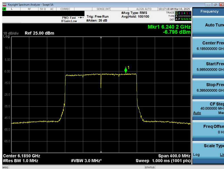
Plot 7-41. Power Spectral Density Plot MIMO ANT2 (160MHz 802.11ax/be (UNII Band 5) – Ch. 47) - LPI/SP
