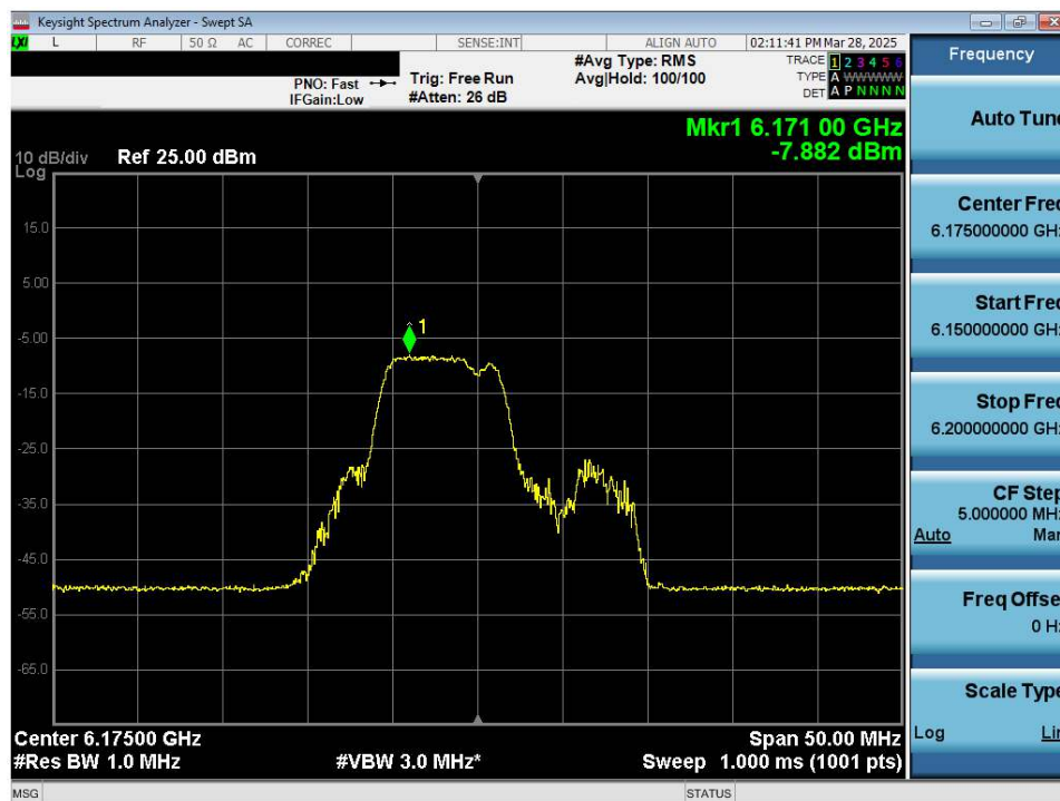
Plot 7-48. Power Spectral Density Plot MIMO ANT2 (20MHz 802.11be (52+26 Tones) (UNII Band 5) – Ch. 45) - VLP
