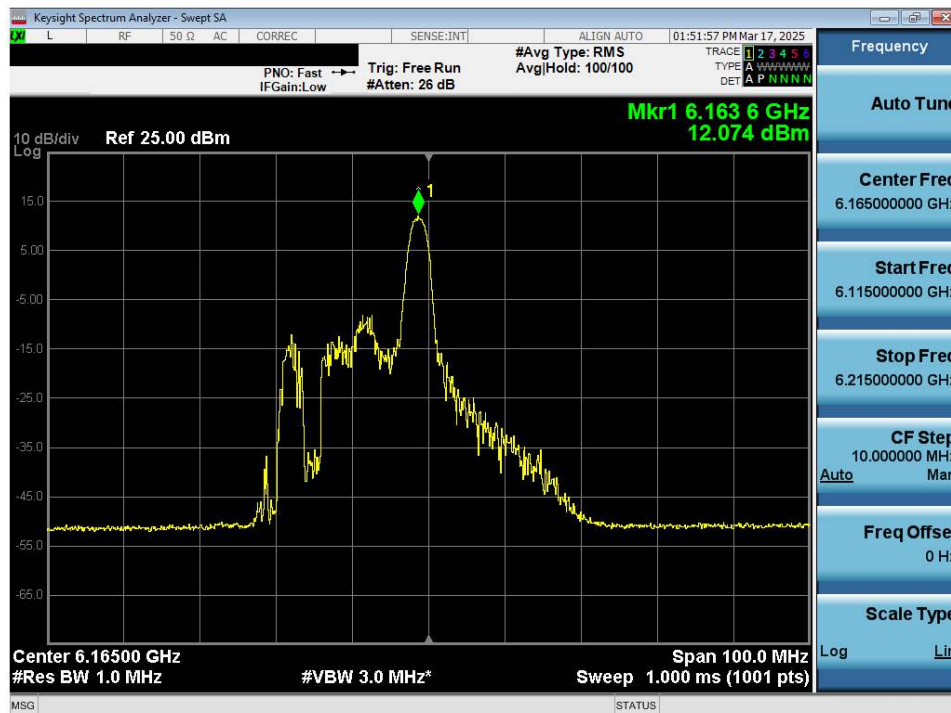
Plot 7-77. Power Spectral Density Plot MIMO ANT2 (40MHz 802.11ax/be (26 Tones) (UNII Band 5) – Ch. 43) - SP
