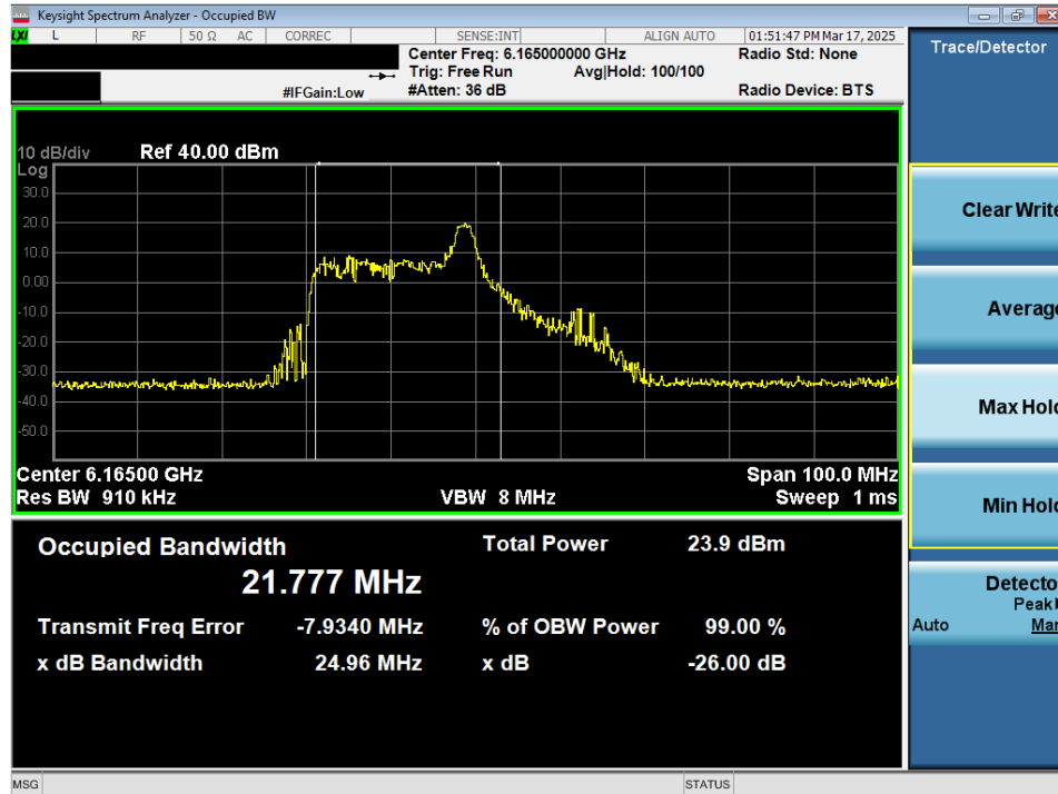
Plot 7-33. 26dB Bandwidth Plot MIMO ANT2 (40MHz 802.11ax/be (26 Tones) (UNII Band 5) – Ch. 43) - SP
