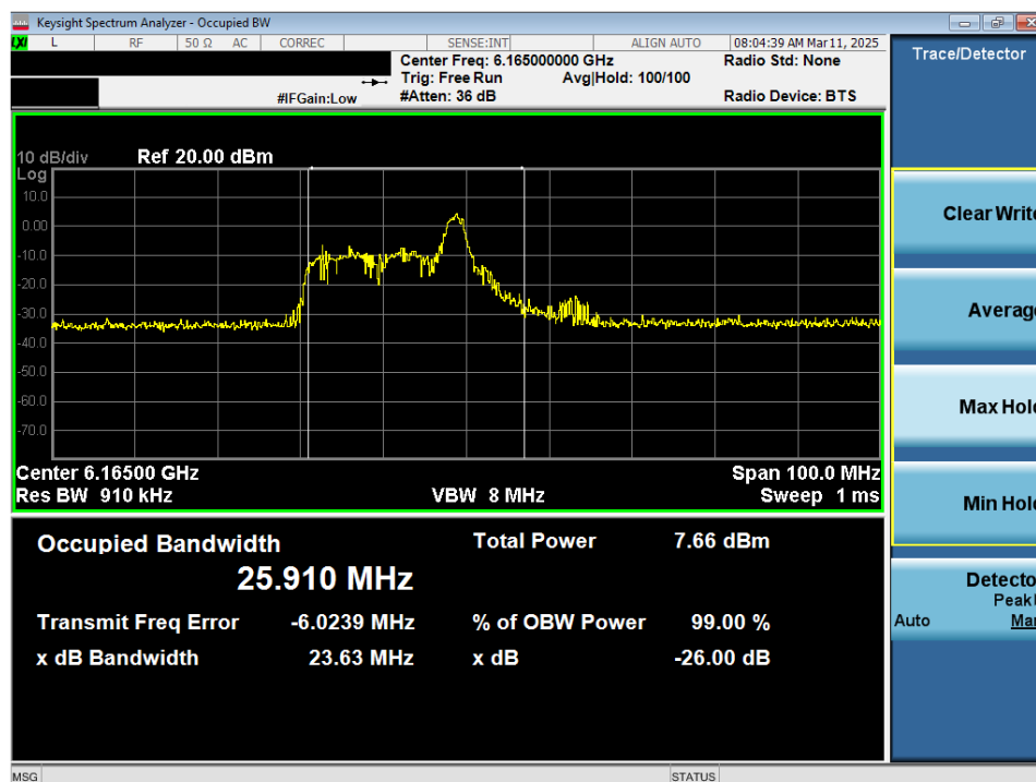
Plot 7-24. 26dB Bandwidth Plot MIMO ANT2 (40MHz 802.11ax/be (26 Tones) (UNII Band 5) – Ch. 43) - LPI
