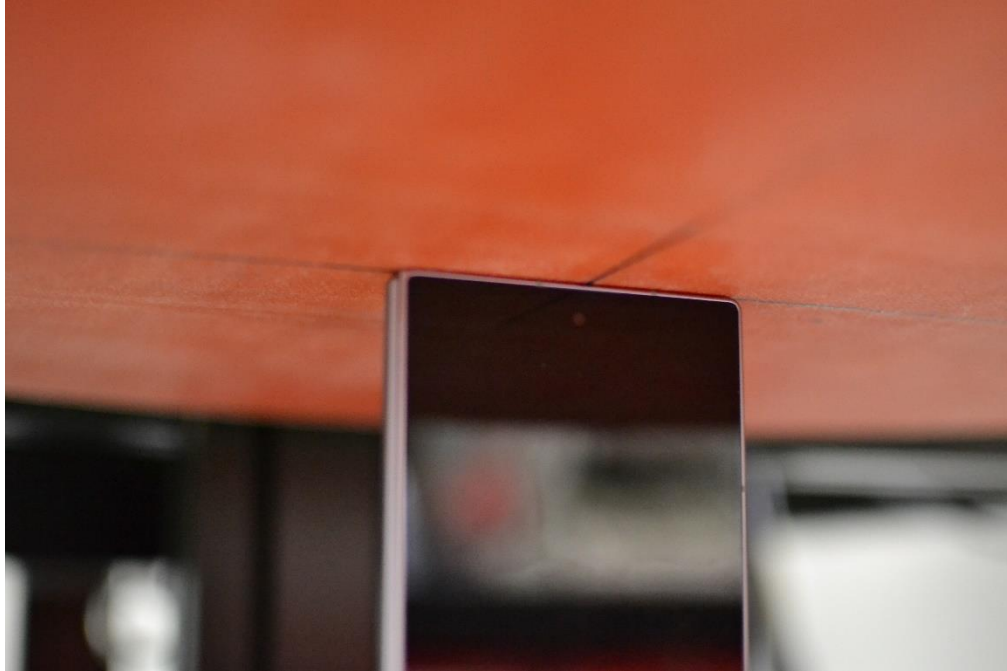
SAR Test Setup Photo 33 – NFC Phablet, Folder Closed, Top Edge at 0mm
