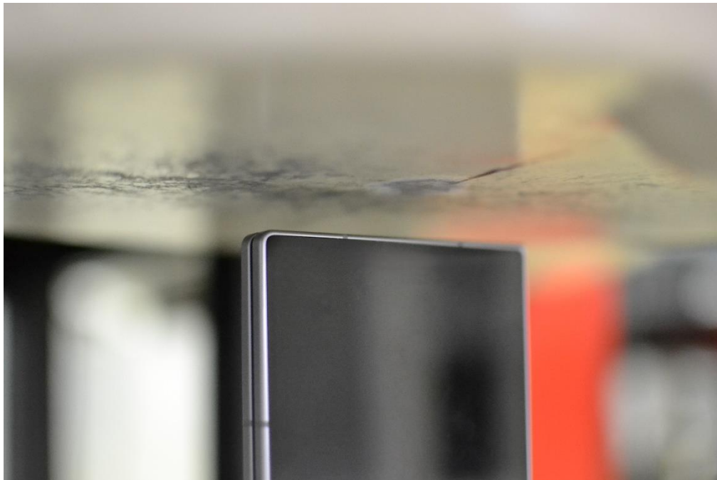
SAR Test Setup Photo 16 – Hotspot, Folder Closed, Bottom Edge at 10mm
