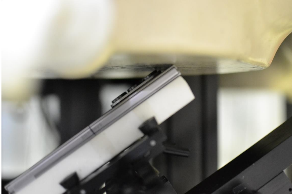
SAR Test Setup Photo 11 – Phablet, Folder Closed, Back Side at 0mm (for AG1)
