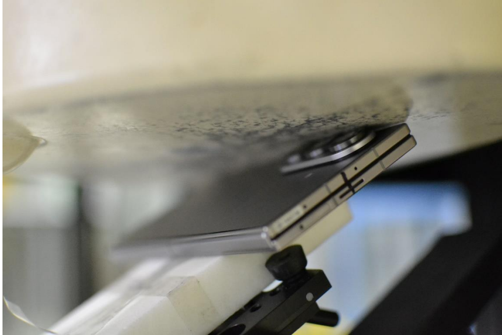
SAR Test Setup Photo 13 – Phablet, Folder Closed, Back Side at 0mm (for Antenna H)
