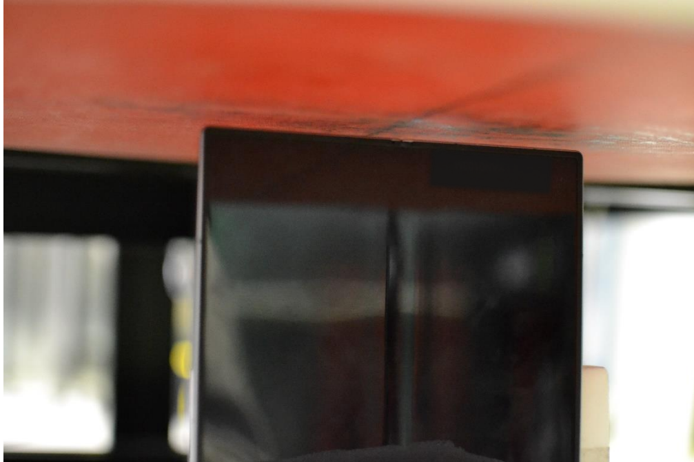
SAR Test Setup Photo 37 – NFC Tablet, Folder Open, Bottom Edge at 5mm
