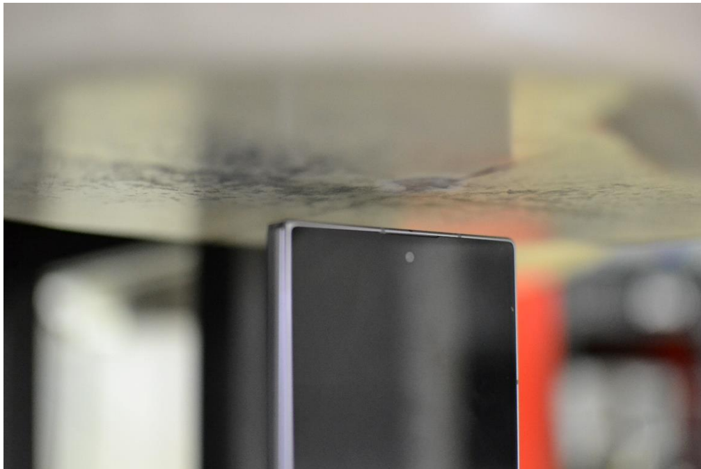
SAR Test Setup Photo 18 – Hotspot, Folder Closed, Top Edge at 10mm
