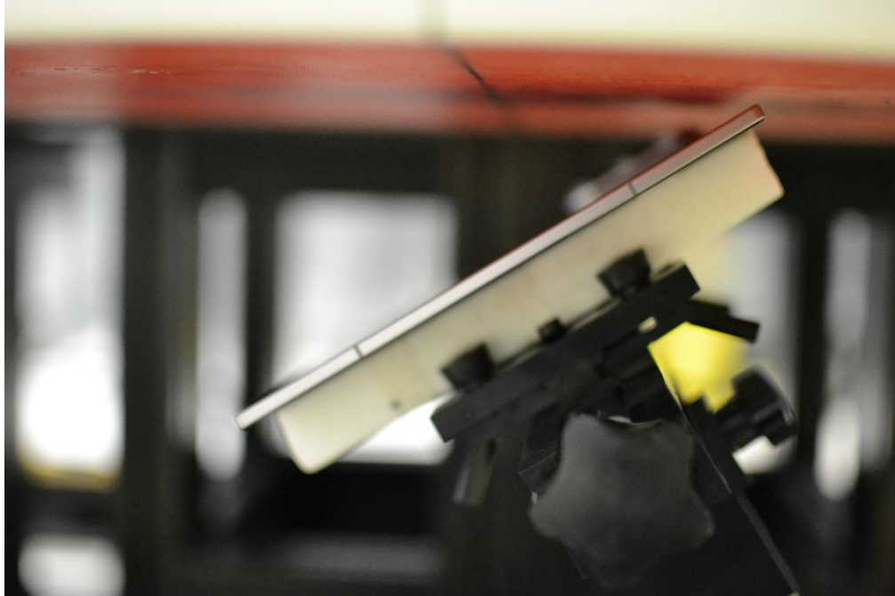
SAR Test Setup Photo 35 – NFC Tablet, Folder Open, Back Side at 5mm
