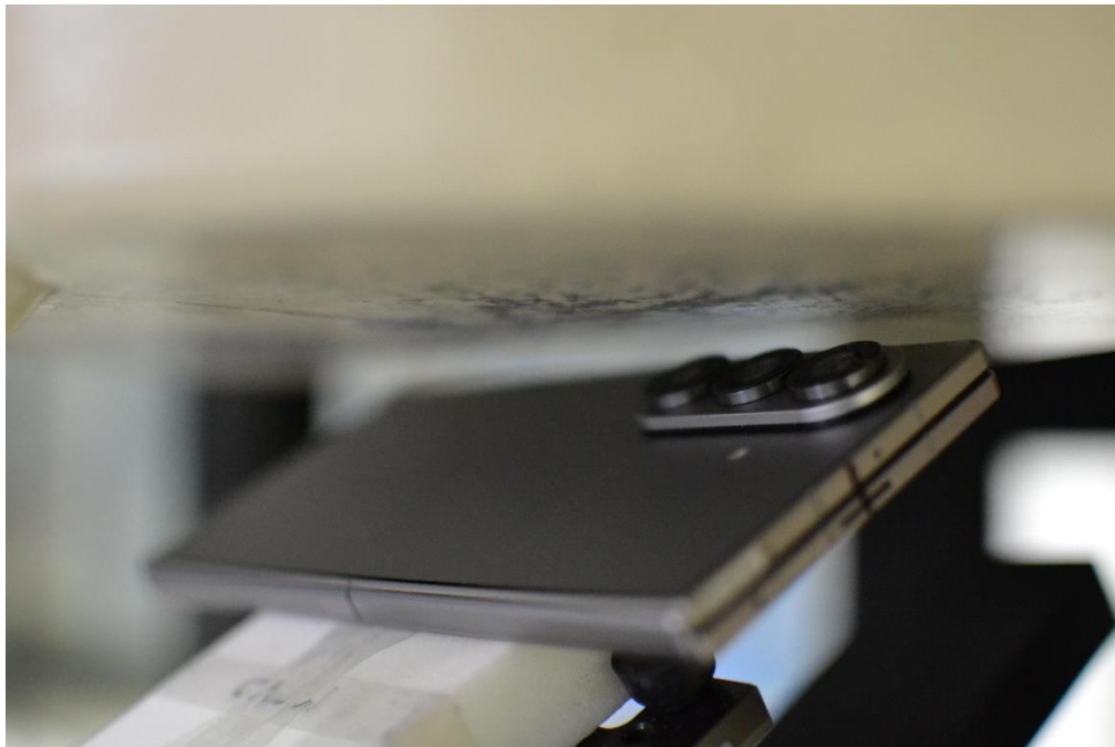
SAR Test Setup Photo 12 – Body-worn/Hotspot, Folder Closed, Back Side at 5mm (for Antenna H)
