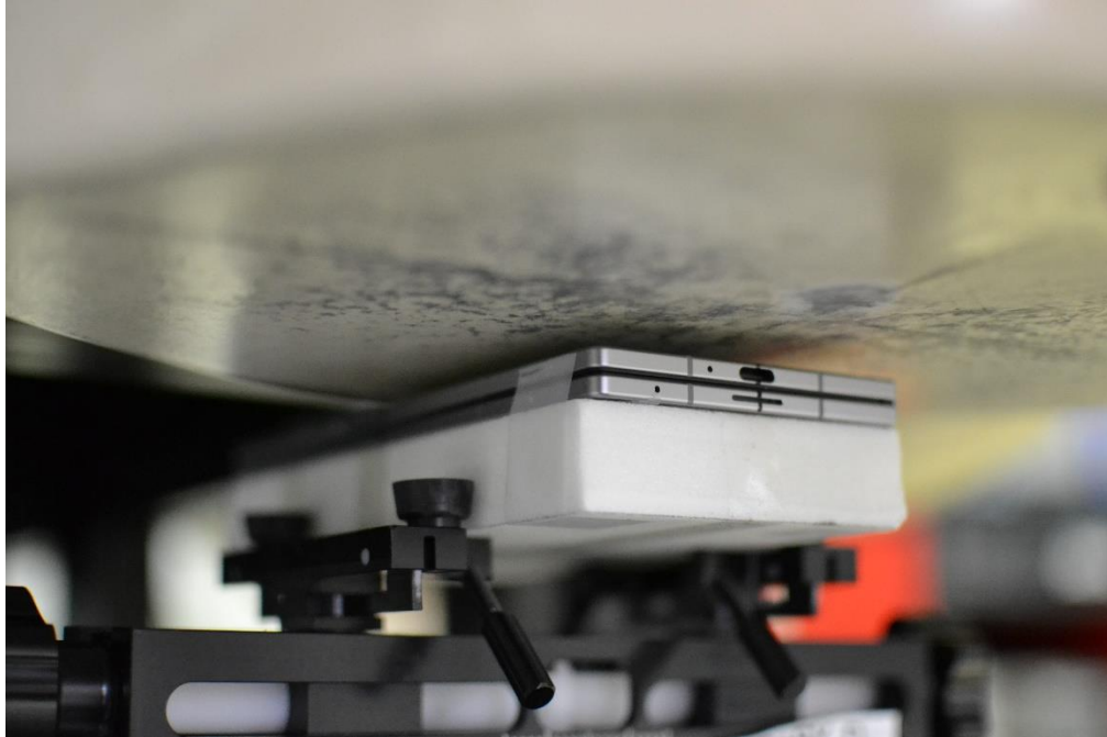
SAR Test Setup Photo 9 – Body-worn/Hotspot, Folder Closed, Back Side at 5mm (for AG0)
