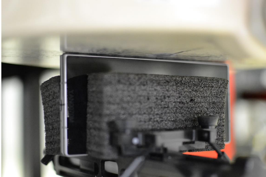
SAR Test Setup Photo 23 – Phablet, Folder Closed, Left Edge at 0mm
