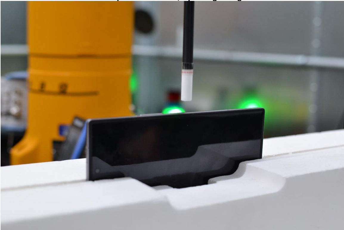
PD Test Setup Photo 50 – PD, Open Right Edge at 9.24mm
