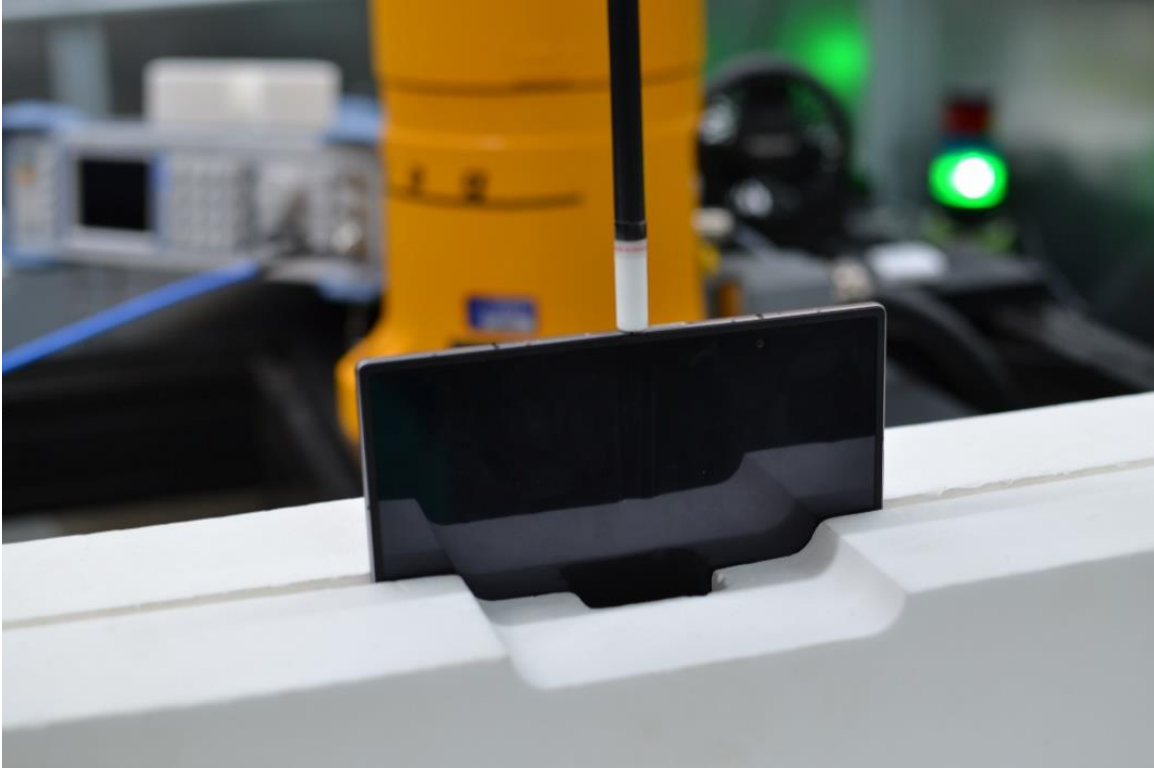
PD Test Setup Photo 47 – PD, Open Top Edge at 2mm
